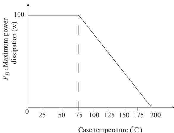
**Fig. 7.27** Typical power derating curve for silicon transistor
