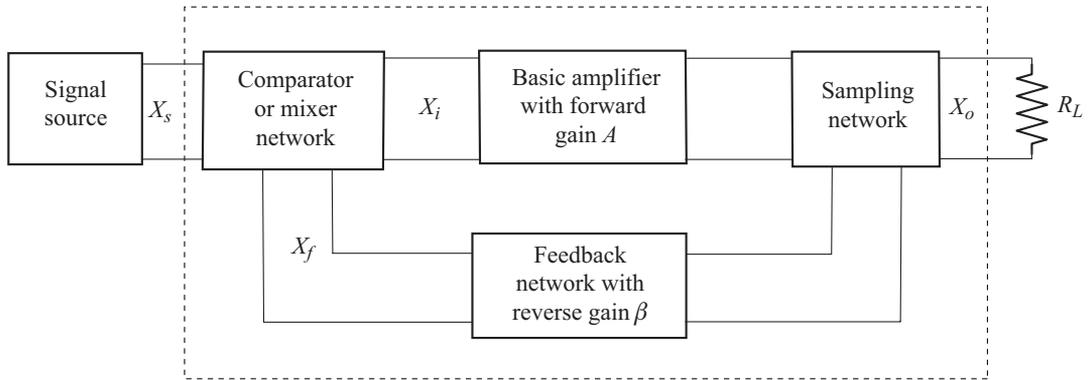
**Fig. 6.5** Block diagram of a typical feedback amplifier
