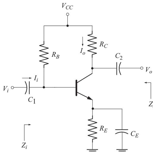
Fig. 3.48 CE emitter bias configuration with bypassed  $R_E$
