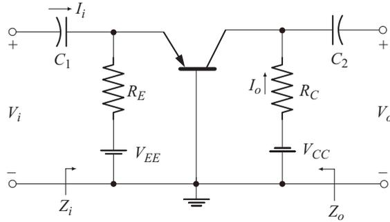
**Fig. 5.31** Common-base configuration
