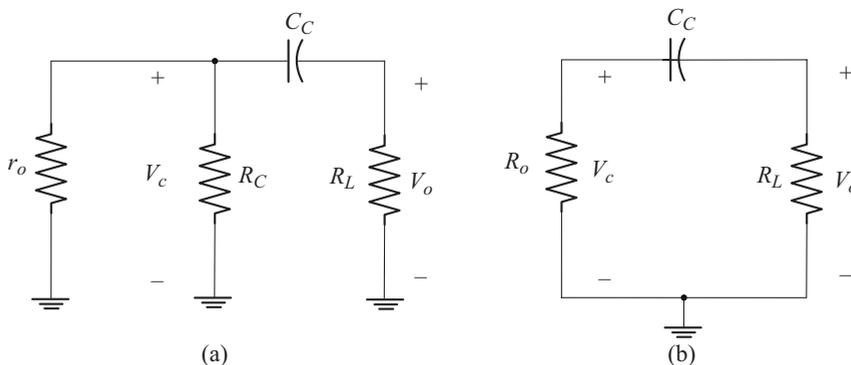
**Fig. 4.16** (a) AC equivalent circuit of output side
