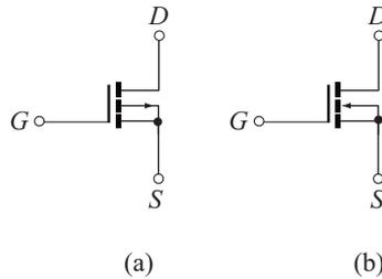
**Fig. 9.35** (a) Circuit symbol of p MOS device
