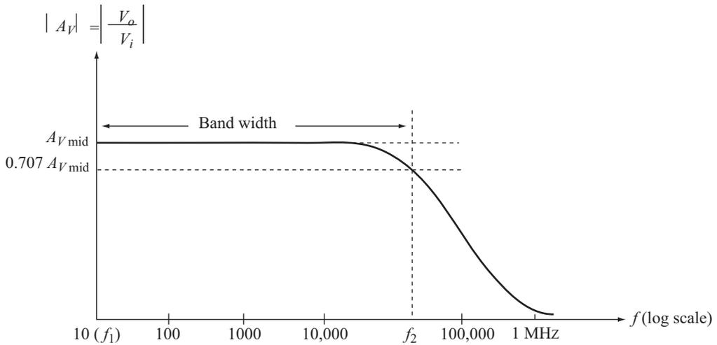
**Fig. 4.3** Frequency response of direct coupled amplifier
