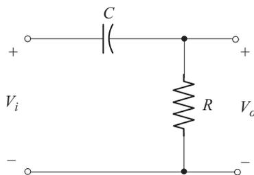
Fig. 4.7 Amplifier modelled as high-pass RC circuit
