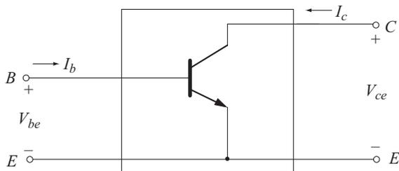
Fig. 3.16 Two port network representation of CE configuration
