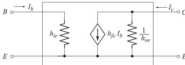
Fig. 3.32 Low frequency hybrid model with  $h_{re}$  removed
