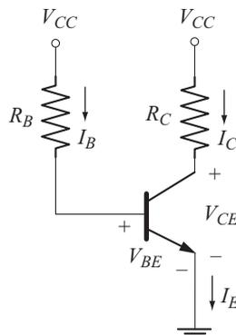
Fig. 2.5 DC equivalent circuit of the fixed-bias circuit
