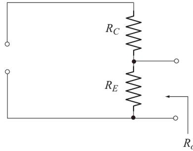
**Fig. 6.38** Circuit to find output resistance
