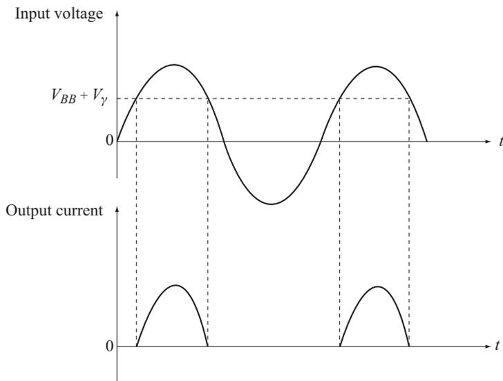
**Fig. 7.4** Current pulses in class C power amplifier
