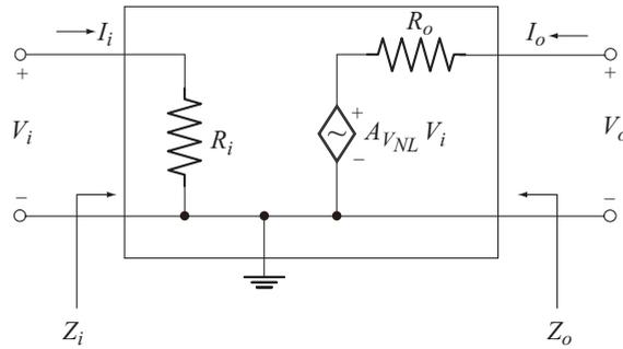
**Fig. 3.86** Amplifier represented by two - port system
