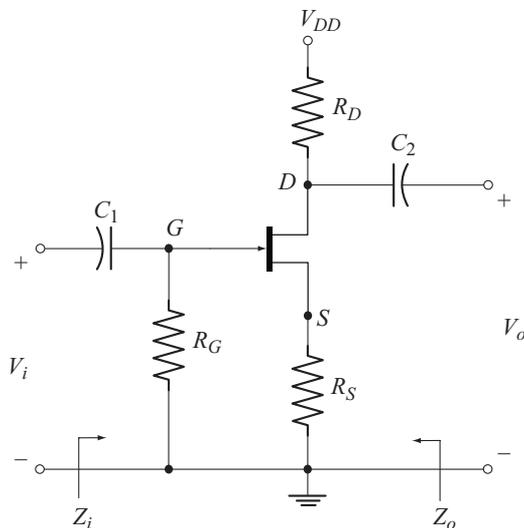
**Fig. 9.15** JFET Common-source amplifier with unbypassed  $R_S$
