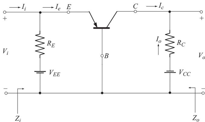
**Fig. 3.61** Common-base configuration
