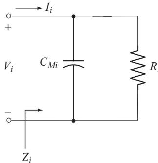
**Fig 4.24** Miller input capacitance [ $C_{Mi}$ ]
