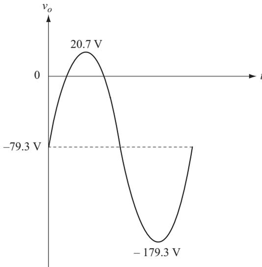
Output waveform with Si diode
