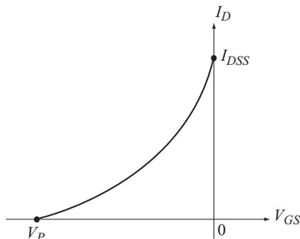
**Fig. 9.3** Transfer characteristics of FET
