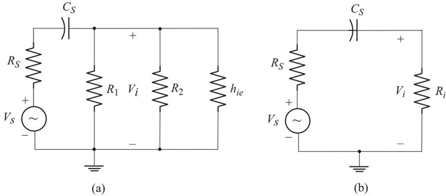
**Fig. 4.15** (a) Input ac equivalent circuit
