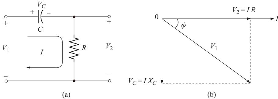
**Fig. 8.4** (a) Single RC-section
