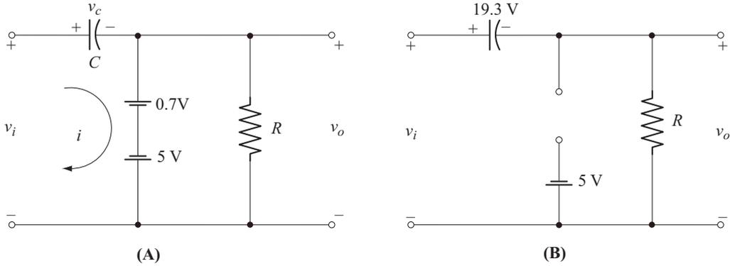
Applying KVL to the current path in the circuit of Fig. A, we have
