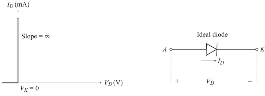
Fig. 1.10 Characteristics and equivalent circuit of ideal diode
