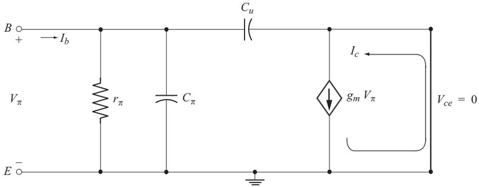
**Fig. 4.36** Circuit to find short circuit current gain
