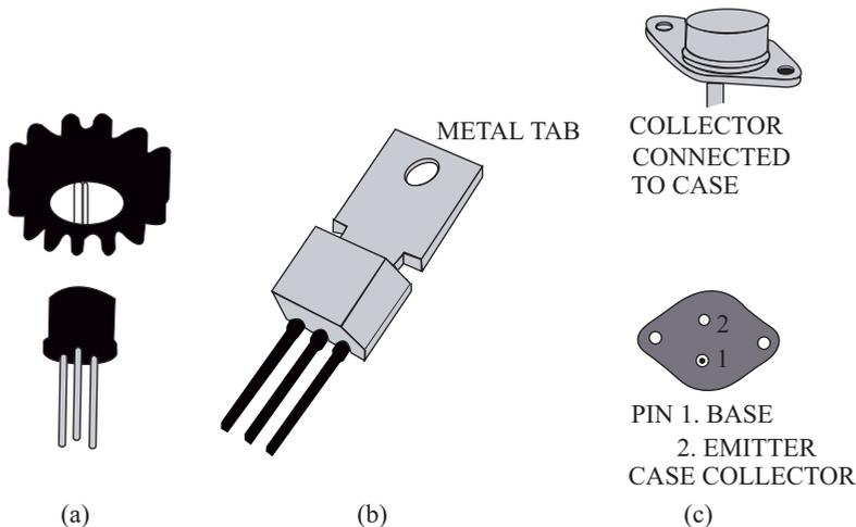
**Fig. 7.26** (a) Push-on heat sink
