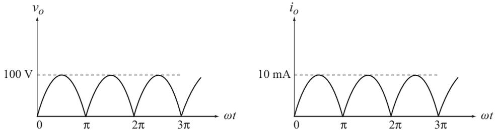
(b)  $v_o$  is a full rectified voltage with peak value of 100 V
