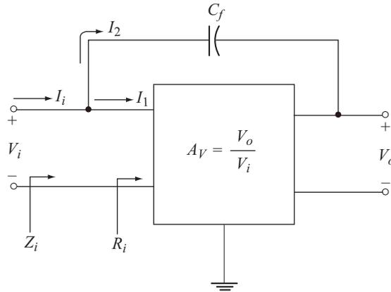
**Fig. 4.23** Circuit to find Miller input capacitance
