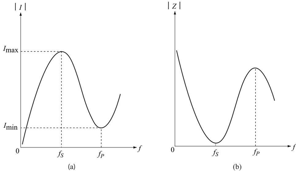
**Fig. 8.12** (a) Frequency response of piezoelectric crystal
