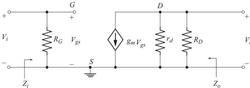
**Fig. 9.14** AC equivalent circuit using small signal model
