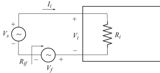
**Fig. 6.17** Input stage of feedback amplifier with series mixing
