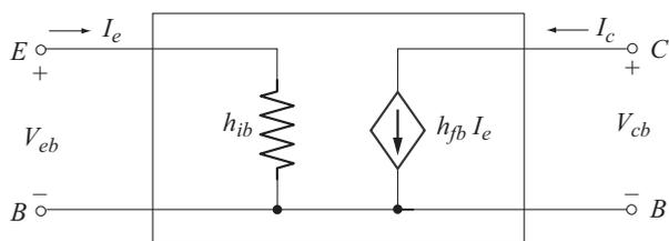
Fig. 3.26 Approximate hybrid equivalent circuit for CB configuration
