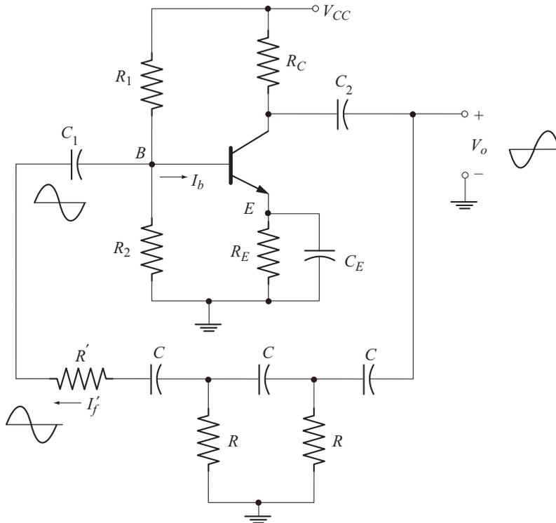
**Fig. 8.5** Transistor RC-phase shift oscillator
