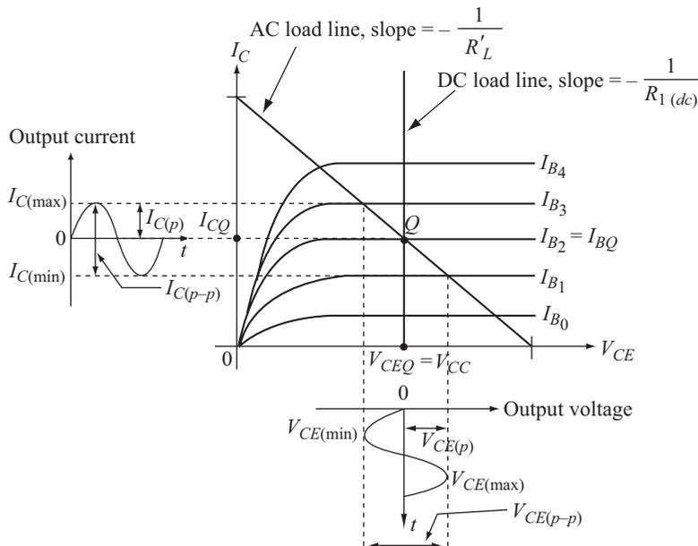
**Fig. 7.12** The ac load line with output voltage and current variations in a transformer-coupled class A power amplifier
