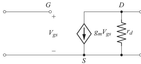
**Fig. 9.36** Small Signal ac model of E-MOSFET
