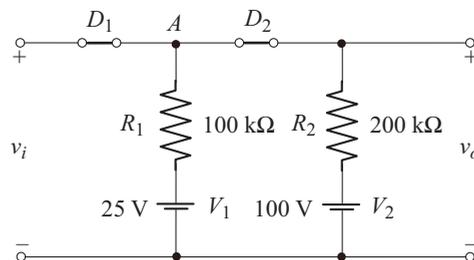
This situation continues until  $v_i$  or  $v_A$  reaches 100 V beyond which point  $D_2$  turns off. Hence,  $D_1$  is on and  $D_2$  is off and  $v_o = 100 \text{ V}$ .
