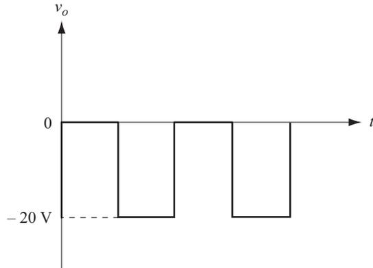
Since the required positive peak is 2.7 V, the waveform shown should be shifted up by 2.7 V. Therefore a dc source of voltage 2.7 V must be placed in series with the diode as shown below.
