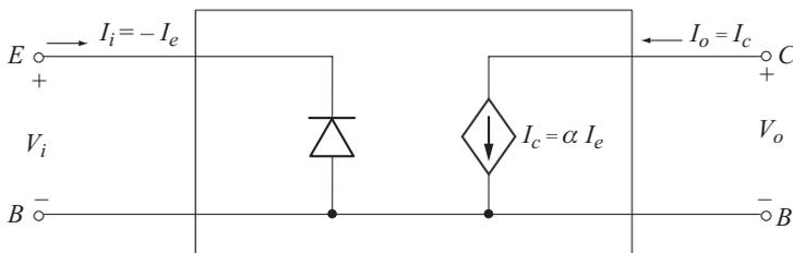
Fig. 3.3  $r_e$  model of transistor in CB configuration
