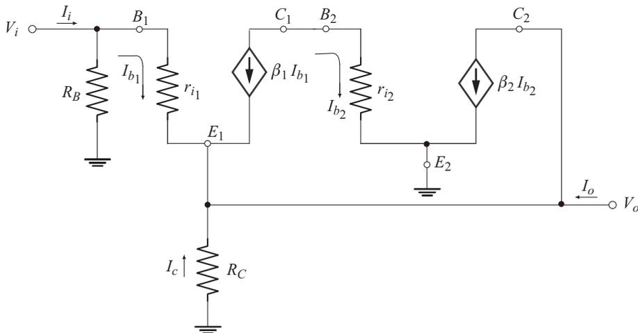
Fig. 5.13 AC equivalent circuit of feedback pair
