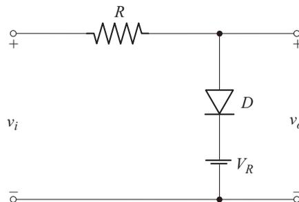
Fig. 1.29 Shunt clipper
