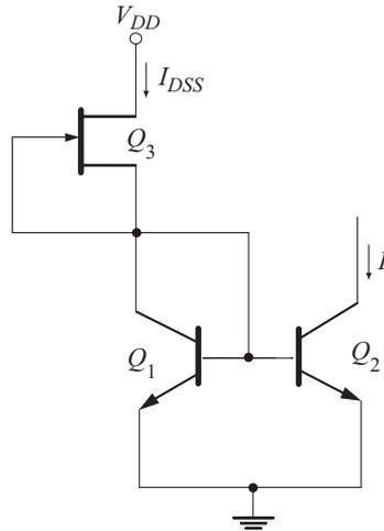
Fig. 5.18 Current mirror using JFET
