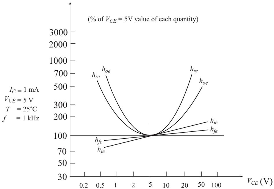
Fig. 3.21 Variation of CE h-parameters with collector-emitter voltage
