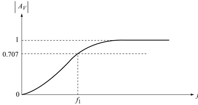
**Fig. 4.10** Low frequency response of high pass-RC circuit
