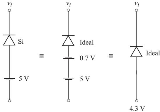
Diode conducts for  $v_i \leq 4.3\text{ V}$ . The equivalent circuit is shown in Fig. A.
