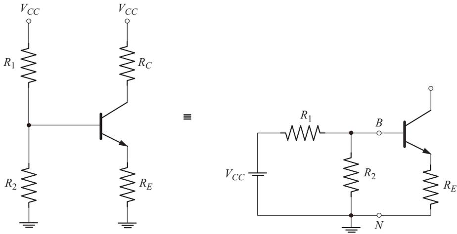
Fig. 2.14 Base circuit of voltage divider bias circuit
