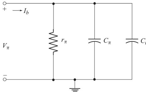
**Fig. 4.37** Circuit to find  $I_b$
