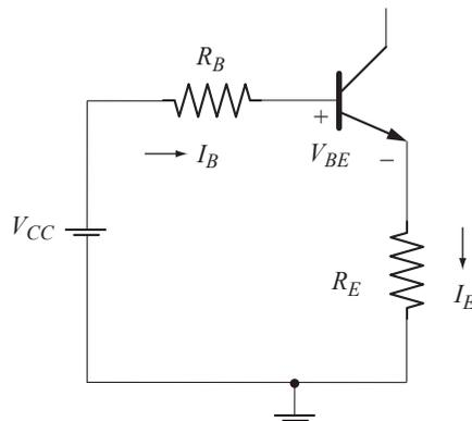
**Fig. 2.11** Base-emitter dc circuit of emitter-bias circuit
