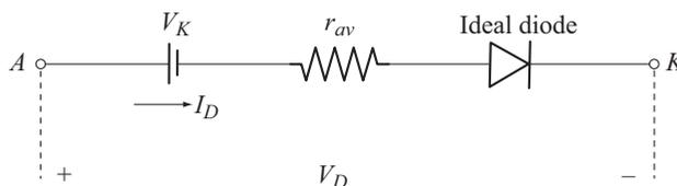
Fig. 1.8 Piecewise linear equivalent circuit of a diode
