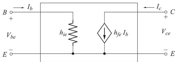
Fig. 3.25 Approximate hybrid equivalent circuit for CE configuration
