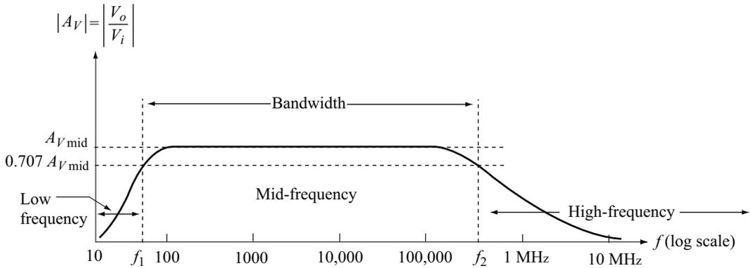
**Fig. 4.1** Frequency response of R-C coupled amplifier
