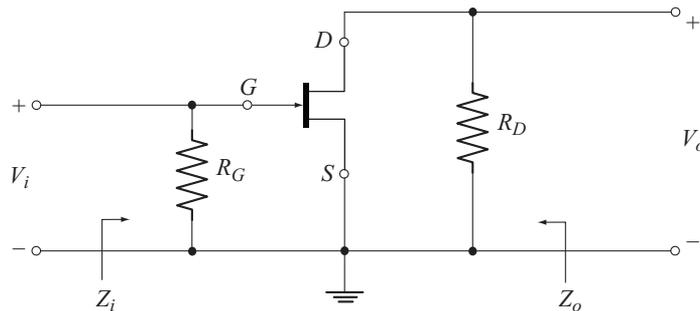
Fig. 9.9 Ac equivalent circuit of JFET common-source amplifier
