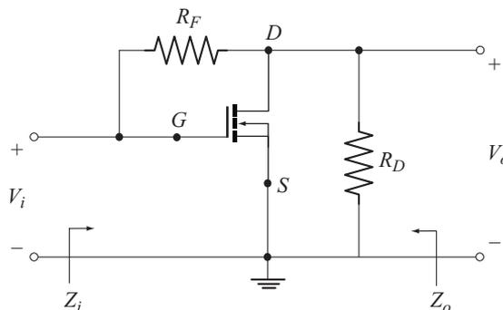
**Fig 9.38** AC equivalent circuit of E-MOSFET drain-feedback configuration
