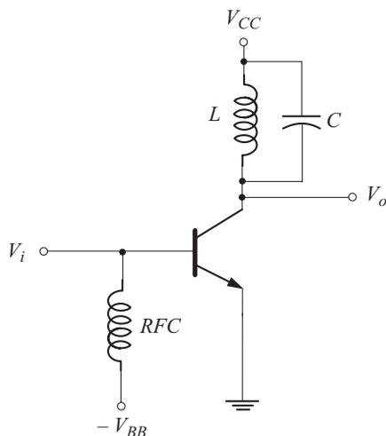
**Fig. 7.5** Tuned class C power amplifier
