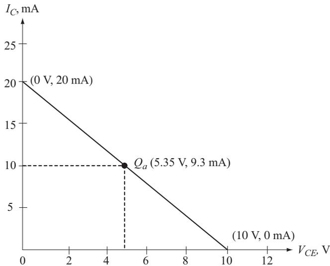
The  $Q$ -point is nearly at the center of the load line.
