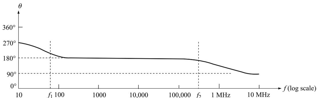
Fig. 4.6 Phase plot of single stage RC-coupled amplifier
