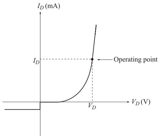
**Fig. 1.4** Determination of  $R_D$  of a diode
