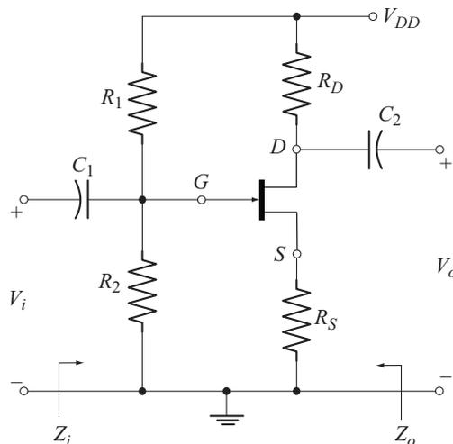
**Fig. 9.21** JFET Voltage-divider configuration with unbypassed  $R_S$
