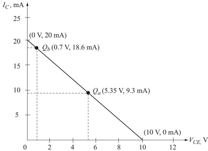
The  $Q$ -point has moved into the saturation region. In general, fixed-bias circuits do not provide stability against variation in  $\beta$ .
