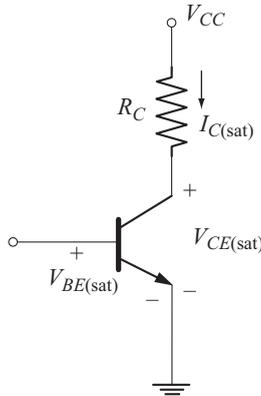
Fig. 2.6 Transistor in saturation
