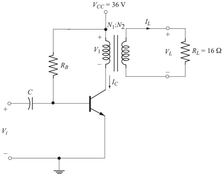
$$\frac{V_1}{V_L} = \frac{N_1}{N_2} = \frac{I_L}{I_C} \quad (\text{A})$$
