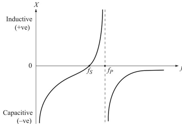
**Fig. 8.13** Crystal reactance versus frequency
