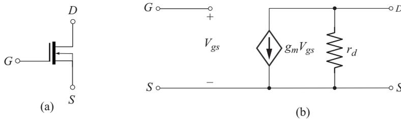
**Fig. 9.34** (a) Circuit symbol of n channel D-MOSFET
