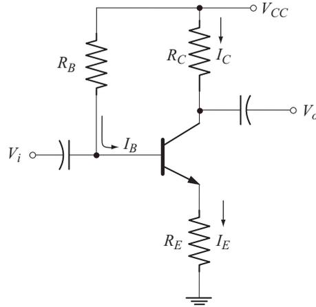
**Fig. 2.10** Emitter-bias circuit
