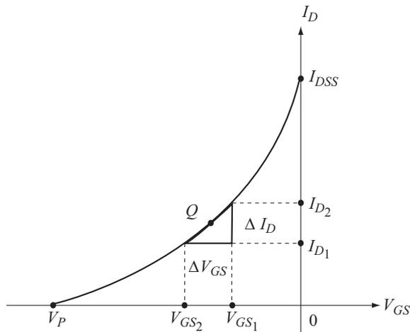
**Fig. 9.6** Graphical determination of  $g_m$
