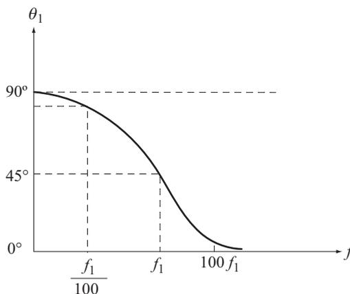
**Fig. 4.12** Phase response of RC network of Fig 4.7
