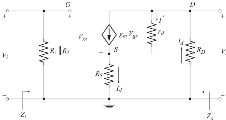
**Fig. 9.22** Ac equivalent circuit of the JFET amplifier of Fig. 9.21
