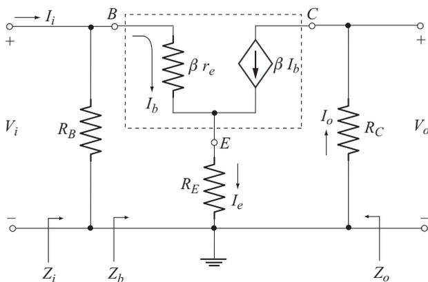
Fig. 3.45 AC equivalent circuit using  $r_e$  model
