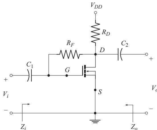
**Fig 9.37** E - MOSFET drain-feedback configuration
