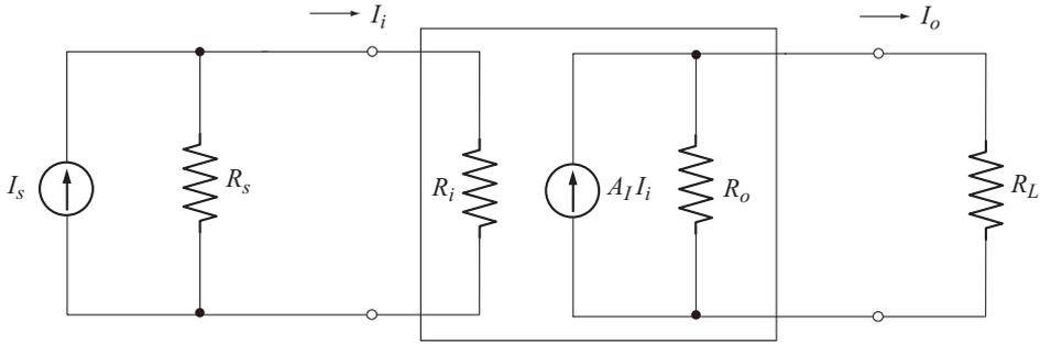
**Fig. 6.2** Equivalent circuit of current amplifier
