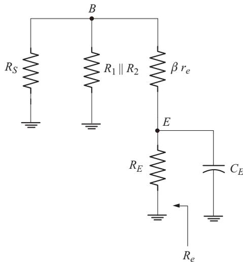
Fig. 4.19 Circuit to find  $R_e$
