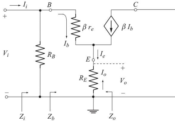
Fig. 3.56 AC equivalent circuit with  $r_e$  model
