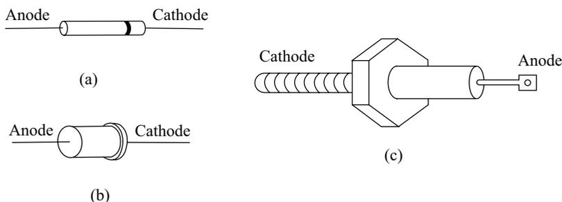
**Fig. 1.13** (a) Low current diode
