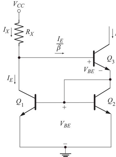
Fig. 5.17 Current mirror circuit with higher output impedance
