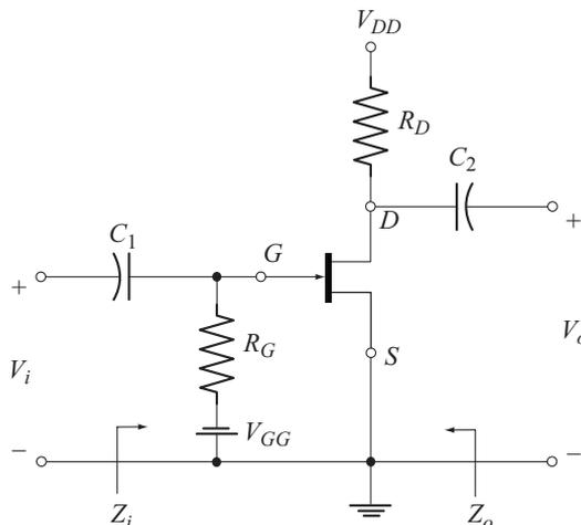
Fig. 9.8 JFET common-source amplifier using fixed bias configuration
