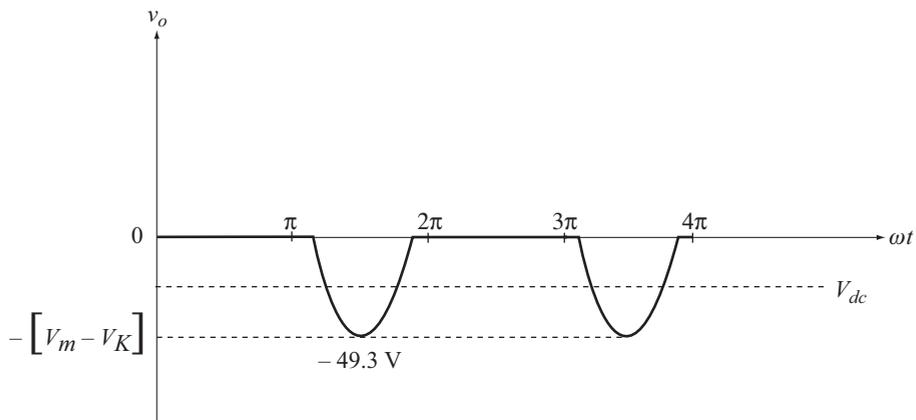
Note that the load current direction is reversed but the diode current flows from anode to cathode only. Therefore we have the following results.
