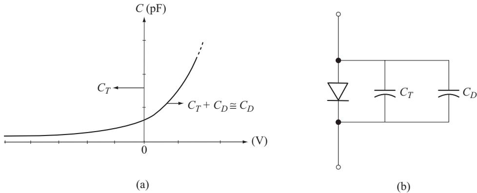
**Fig. 1.11** (a) Transition and diffusion capacitance versus applied bias for a Si diode
