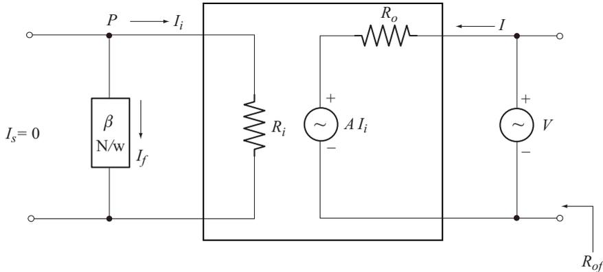
**Fig. 6.26** Output resistance of voltage shunt feedback amplifier
