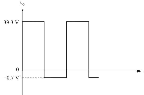
But the desired output voltage has a positive peak of 30 V. Therefore, the waveform shown above has to be shifted down by 9.3 V. This can be done by using an additional dc source  $V_R$ , whose value is given by
