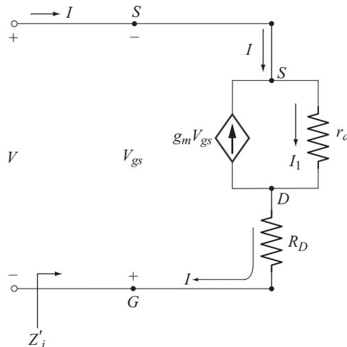
**Fig. 9.32** Circuit to find  $Z'_i$
