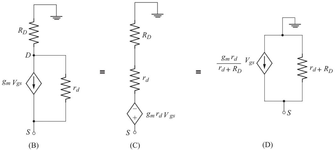
The current source  $g_m V_{gs}$  in parallel with  $r_d$  in Fig. B is converted into its equivalent voltage source as shown Fig. (C). The voltage source is converted back into its equivalent current source in Fig. (D).
