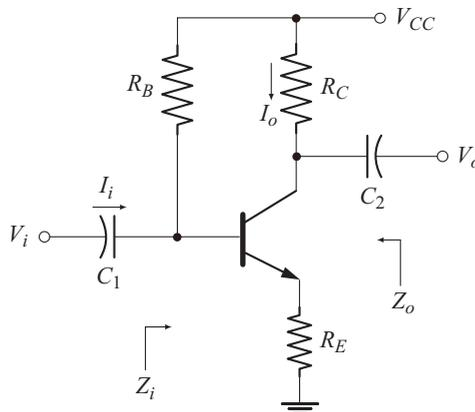
Fig. 5.27 Emitter bias configuration with un bypassed  $R_E$
