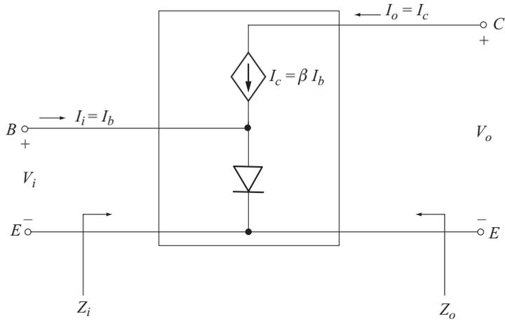
**Fig. 3.7**  $r_e$  model of transistor in CE Configuration
