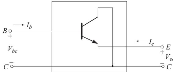
**Fig. 3.18** Two port network representation of CC configuration
