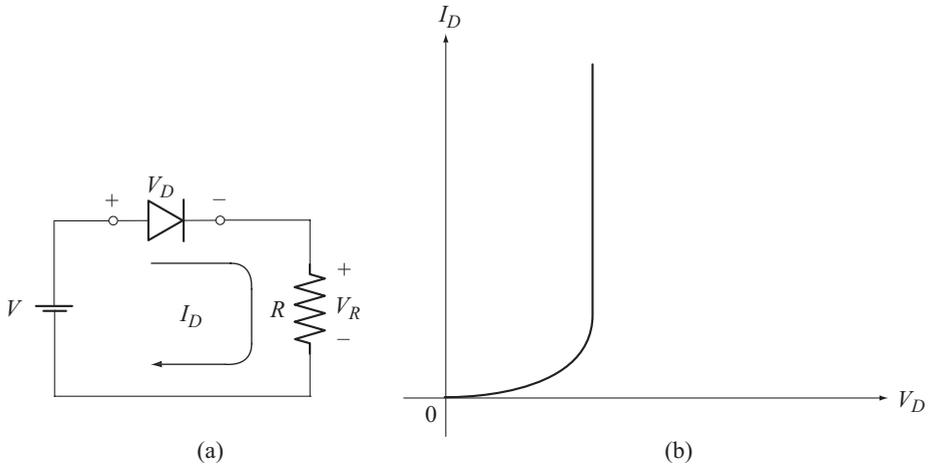
**Fig. 1.14** (a) Series diode configuration
