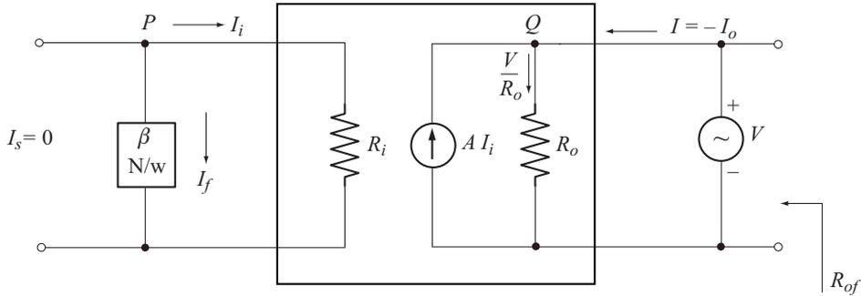
**Fig. 6.28** Output resistance of current shunt feedback amplifier
