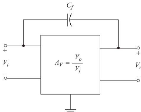
**Fig. 4.22** Inverting amplifier with capacitance between input and output nodes
