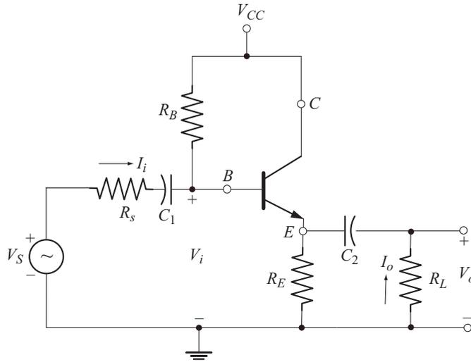
Fig. 3.82 Emitter-follower configuration with  $R_S$  and  $R_L$
