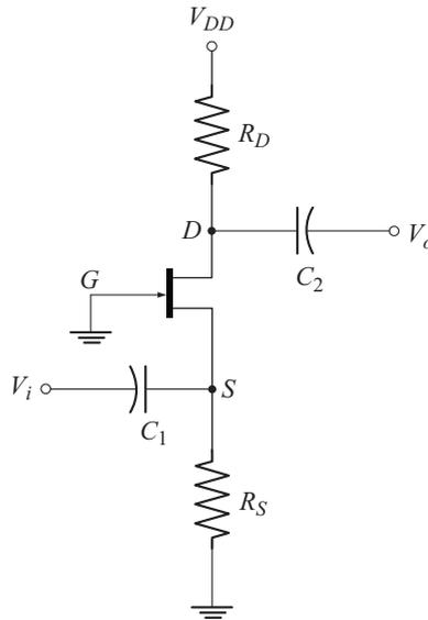
**Fig. 9.29** Alternate representation of the circuit of Fig. 9.28
