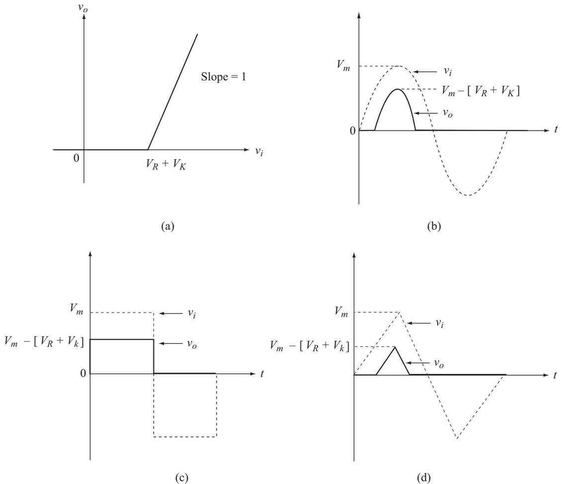
**Fig. 1.37** (a) Transfer characteristics
