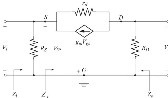
**Fig. 9.31** AC equivalent circuit using JFET small signal model
