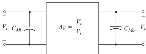
Fig. 4.26 Amplifier with  $C_f$  replaced by Miller capacitances
