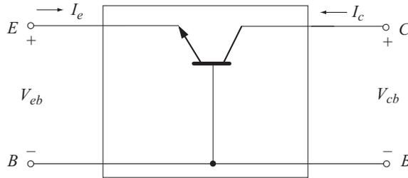
**Fig. 3.14** Two port network representation of CB configuration
