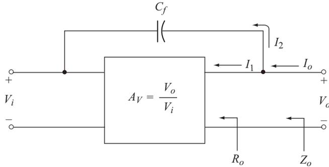
**Fig 4.25** Circuit to find miller output capacitance
