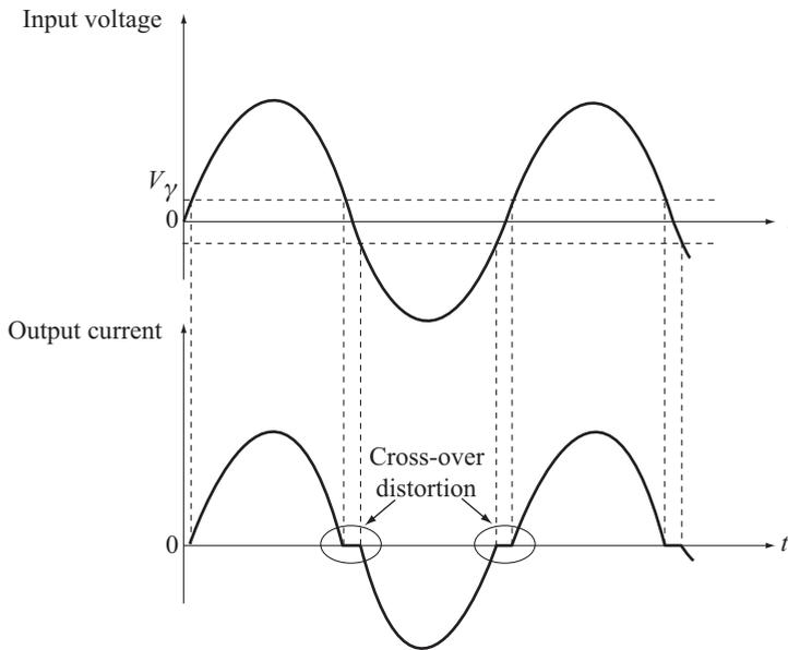
**Fig. 7.3** Cross-over distortion in class B push-pull amplifier
