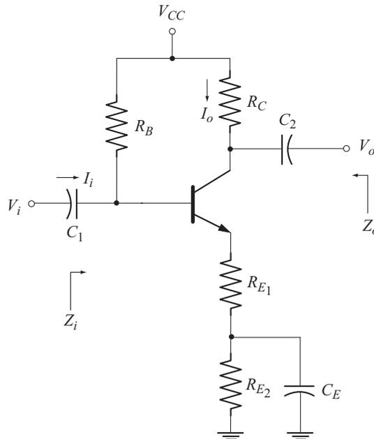
Fig. 3.52 Emitter-bias configuration with partly bypassed  $R_E$
