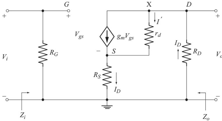
**Fig. 9.16** Ac equivalent of the amplifier of Fig. 9.15
