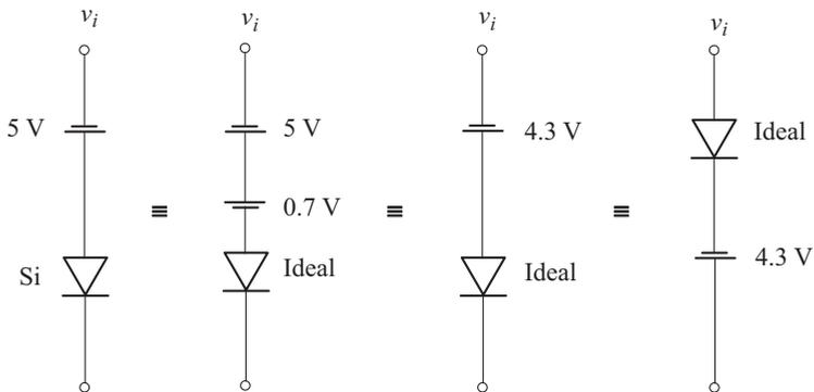
Diode conducts for  $v_i \geq -4.3$  V. The equivalent circuit during diode conduction is shown in Fig. A.
