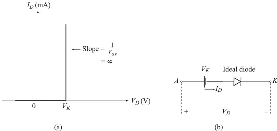
**Fig. 1.9** (a) Piece wise linear characteristics with  $r_{av} = 0 \Omega$
