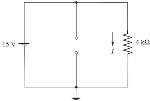
$$I = \frac{15 \text{ V}}{4 \text{ k}\Omega} = 3.75 \text{ mA}$$
