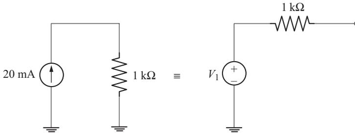
$$V_1 = (20 \text{ mA})(1 \text{ k}\Omega) = 20 \text{ V}$$
