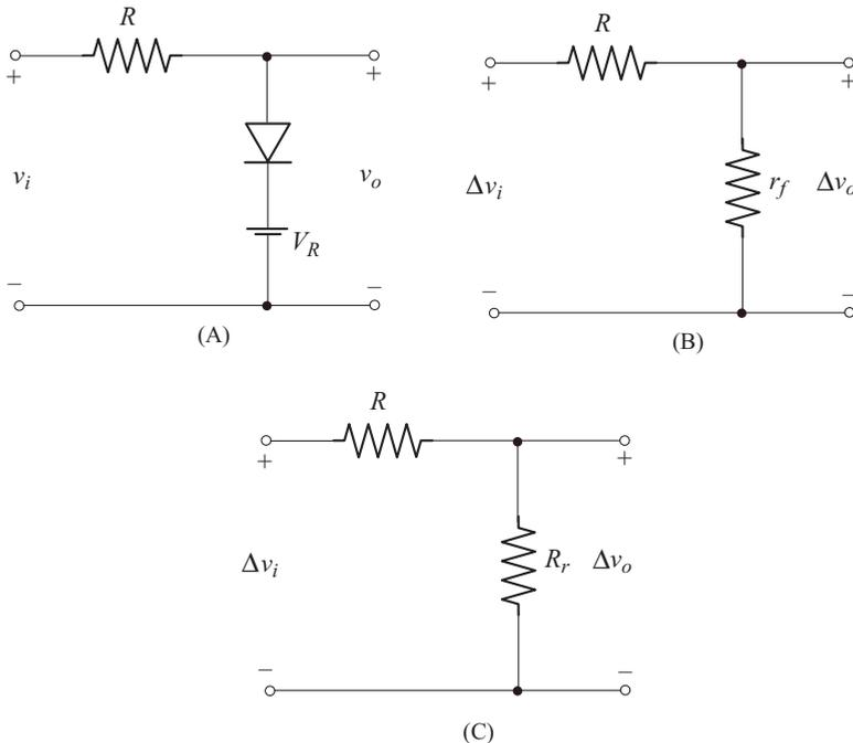
The equivalent circuit during diode conduction is shown in Fig. B. It should be noted that  $r_f$  is same as  $r_{av}$ . Since we have considered the incremental values,  $\Delta v_i$  and  $\Delta v_o$  of  $v_i$  and  $v_o$  respectively,  $V_K$  and  $V_R$  are not shown. This is because  $\Delta V_K = 0$  and  $\Delta V_R = 0$ , since  $V_K$  and  $V_R$  are constant values.
