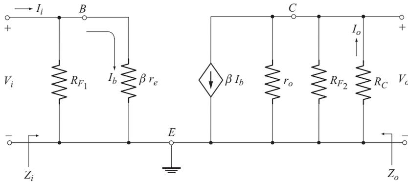
**Fig. 3.70** AC equivalent circuit with  $r_e$  model
