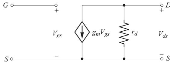
**Fig. 9.5** Small signal ac model of FET
