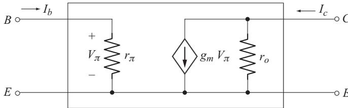
Fig. 3.31 Simplified low frequency hybrid  $\pi$  model
