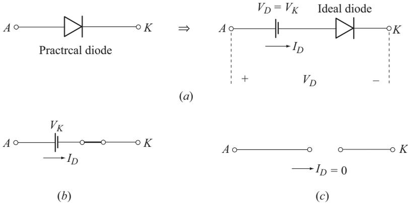
**Fig. 1.16** (a) Approximate equivalent circuit of diode
