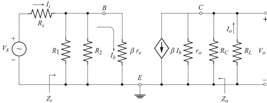
Fig. 3.81 Ac equivalent circuit using  $r_e$  model
