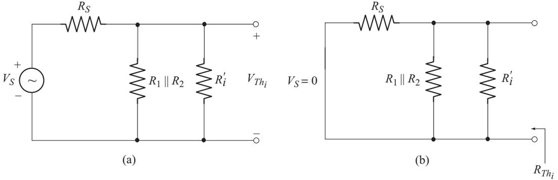
**Fig. 4.30** (a) Circuit to find  $V_{Th_i}$  (b) Circuit to find  $R_{Th_i}$
