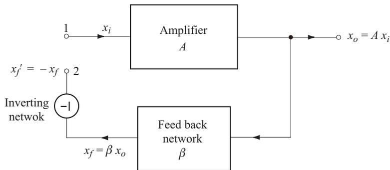
**Fig. 8.1** Illustration of basic principle of oscillators
