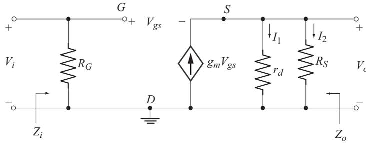
**Fig. 9.26** Ac equivalent circuit of Fig. 9.25 redrawn
