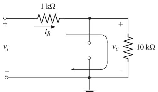
**Fig. A** Equivalent circuit during diode conduction
