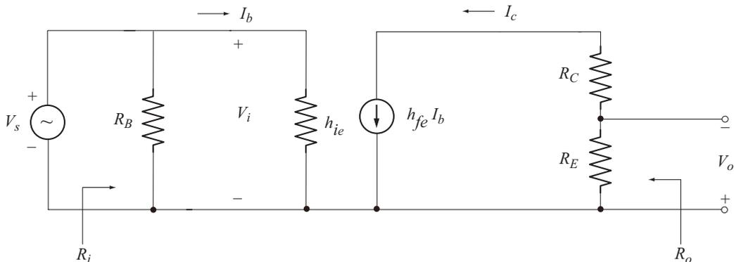
**Fig. 6.37** Basic amplifier without feedback using hybrid model
