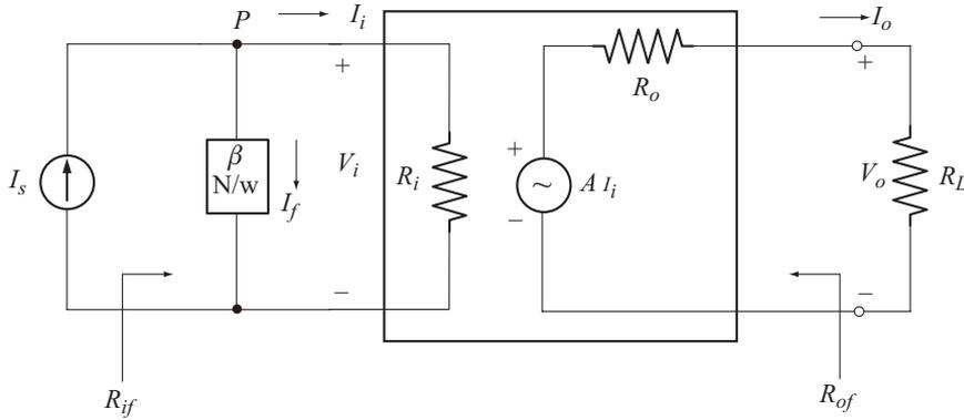
Fig. 6.20 Voltage - shunt feedback amplifier
