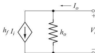
Fig. 3.11 Circuit model of  $V_i = h_i I_i + h_r V_o$
