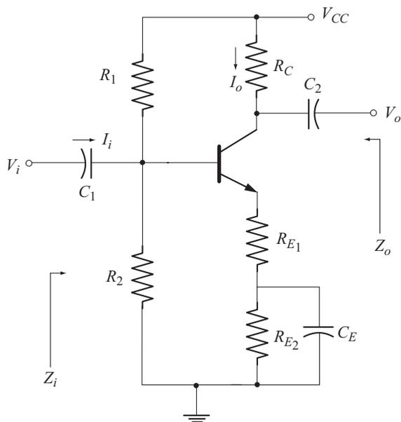
Fig. 3.53 Voltage divider-bias configuration with partly bypassed  $R_E$
