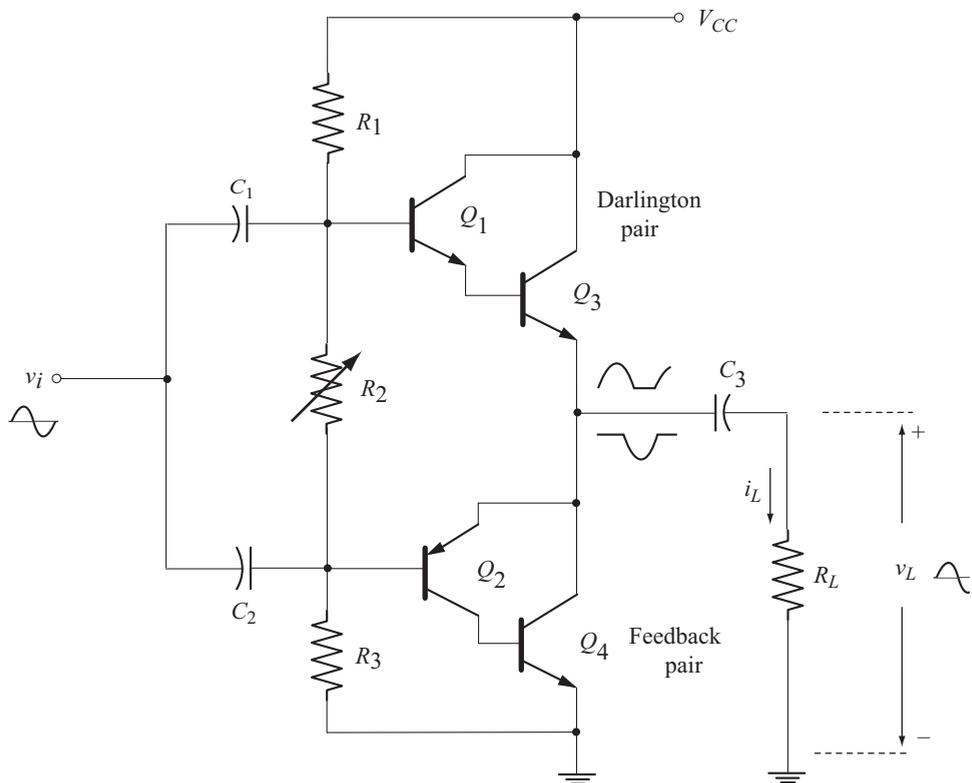
Fig. 7.23 Quasi-complementary class B push-pull power amplifier
