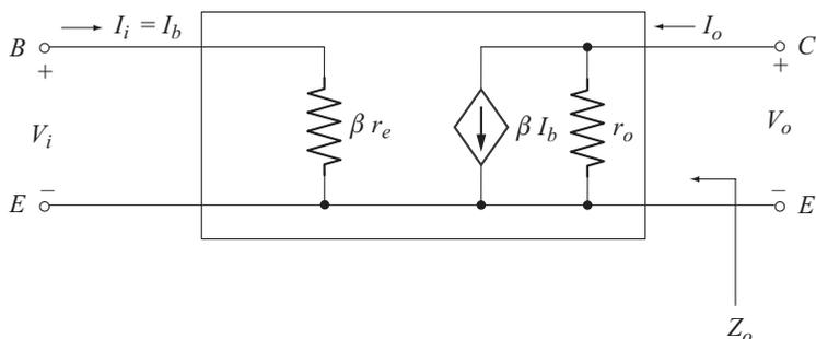
Fig. 3.9  $r_e$  model of CE configuration including  $r_o$
