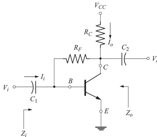
**Fig. 3.64** Collector feedback configuration
