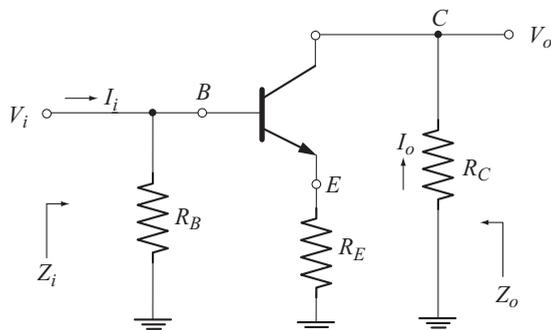
Fig. 3.44 AC equivalent circuit
