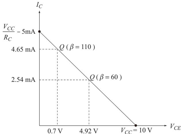
Observe that, when  $\beta$  changes from 60 to 110, the  $Q$  point shifts from the middle of the active region to near saturation. Therefore fixed bias circuit has very poor stability of the operating point. The reason for this is that, there is no change in the value of the base current.
