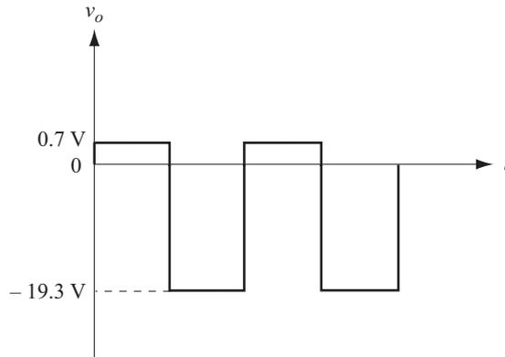
The desired output voltage has a positive peak of 2.7 V. Therefore the waveform shown above has to be shifted up by 2 V. This can be done by using an additional dc source  $V_R$  given by
