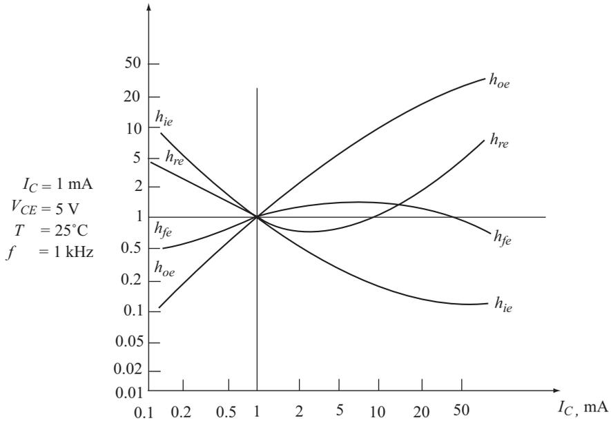
Fig. 3.20 Variation of CE h-parameters with collector current
