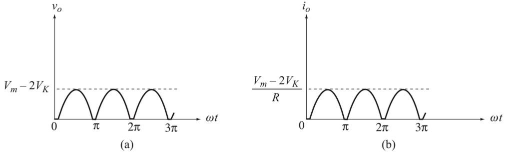
**Fig. 1.24** Wave forms of  $v_o$  and  $i_o$
