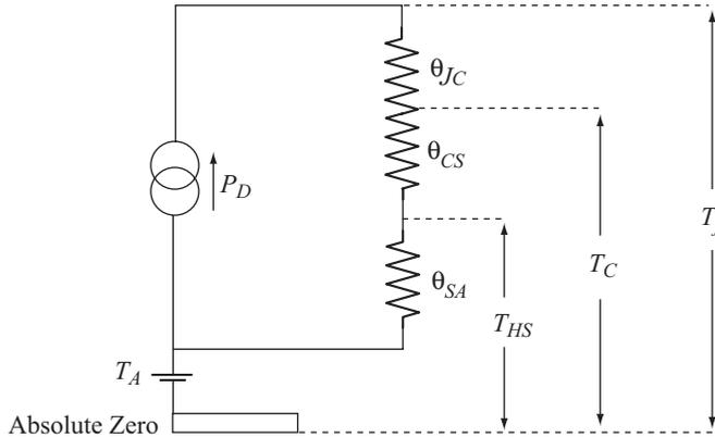
**Fig. 7.28** Thermal-to-electrical analogy
