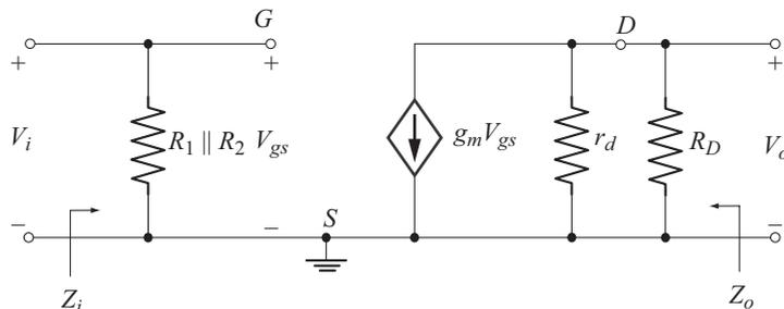
**Fig. 9.20** Ac equivalent circuit redrawn using small-signal ac model of JFET
