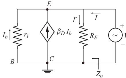
**Fig. 5.9** Simplified circuit to find  $Z_o$ .
