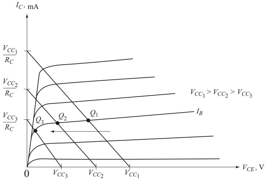
Fig. 2.9 Effect of Variation in  $V_{CC}$  on Q-point
