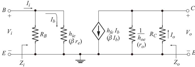
**Fig. 5.25** AC equivalent circuit
