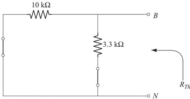
Fig. C Circuit to find  $R_{Th}$
