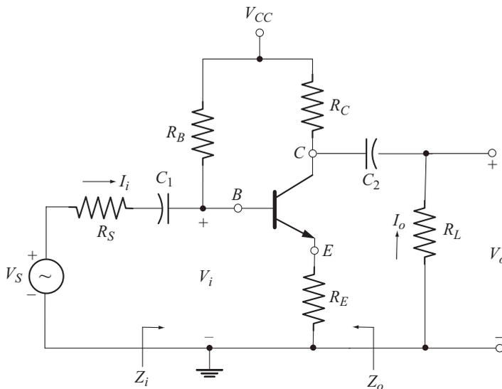
**Fig. 3.84** CE emitter-bias configuration with  $R_S$  and  $R_L$
