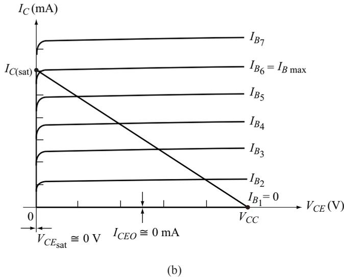
Fig. 2.22 (a) Transistor switch (b) Output characteristics
