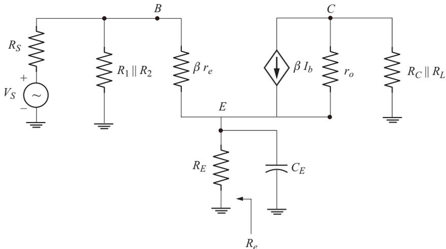
Fig. 4.18 AC equivalent circuit using hybrid model
