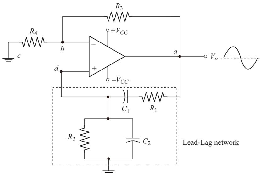
**Fig. 8.6** Wein bridge oscillator using Op-Amp amplifier
