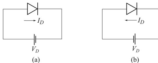
**Fig. 1.1** (a) Forward biased  $p$ - $n$  junction
