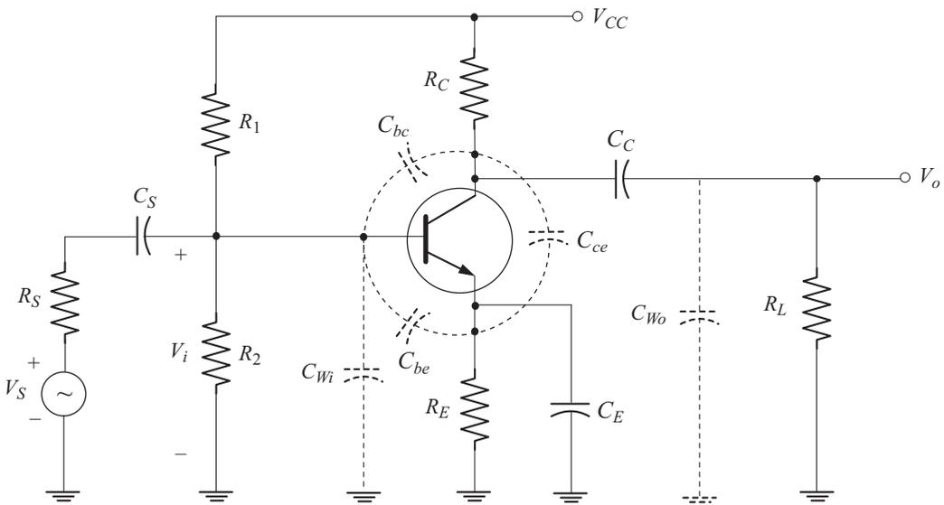
Fig. 4.27 RC-coupled amplifier with parasitic and wiring capacitances
