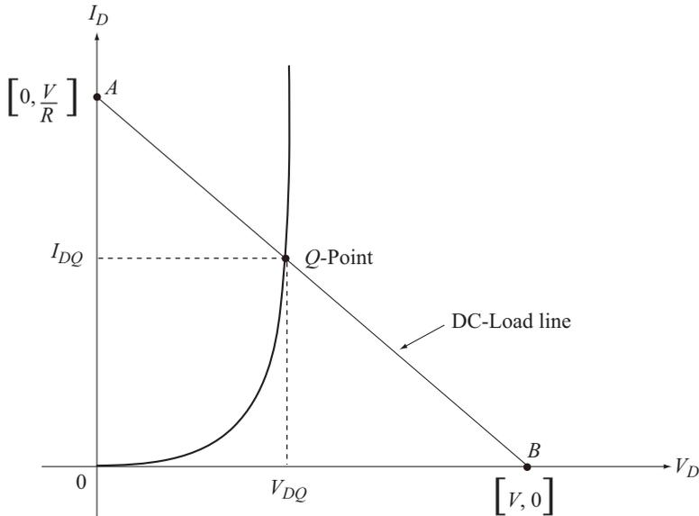
Fig. 1.15 DC load-line drawn on diode characteristics
