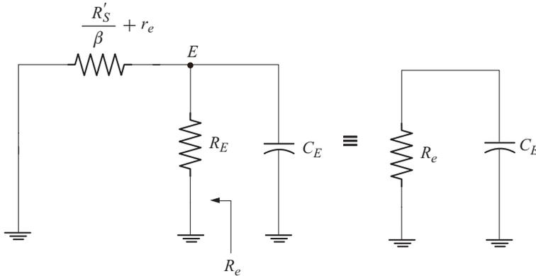
**Fig. 4.21** Circuit to find  $R_e$
