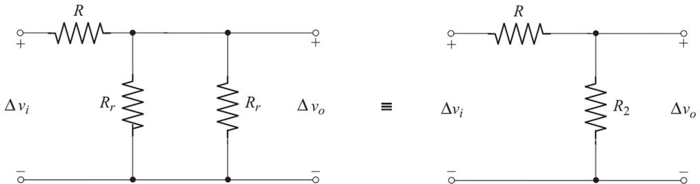
$$R_2 = R_r \parallel R_r = \frac{R_r}{2} = 50 \text{ k}\Omega$$
