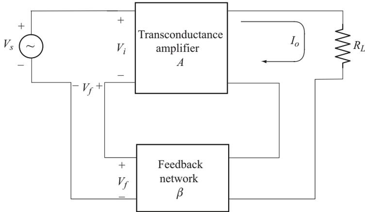
**Fig. 6.15** Current-series feedback topology
