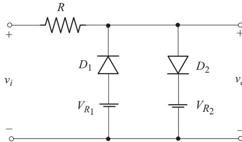
**Fig. 1.38** Clipping circuit with two reference voltages
