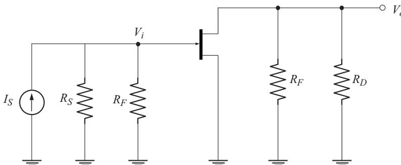
Fig. 6.48 Basic amplifier circuit with out feedback
