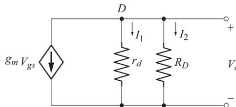
**Fig. 9.12** Output ac equivalent Circuit
