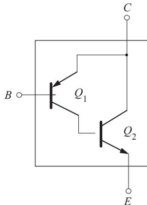
Fig. 5.10 Feedback pair connection
