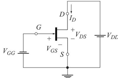
**Fig. 9.2** Biasing arrangement for  $n$ -channel FET
