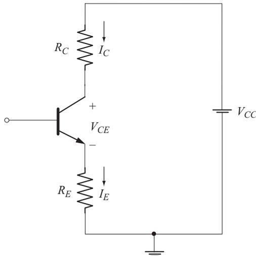
Fig. 2.12 Collector-emitter dc circuit of emitter-bias circuit
