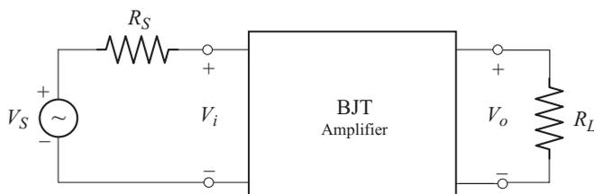
**Fig. 3.75** Defining loaded voltage gain with  $R_s$
