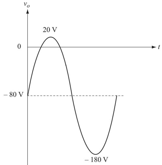
Output waveform with ideal diode
