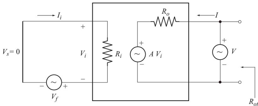
**Fig. 6.25** Output resistance of voltage series feedback amplifier
