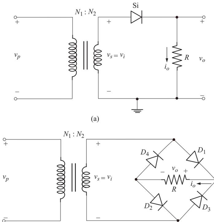
**Fig. 1.25** (a) Half wave rectifier
