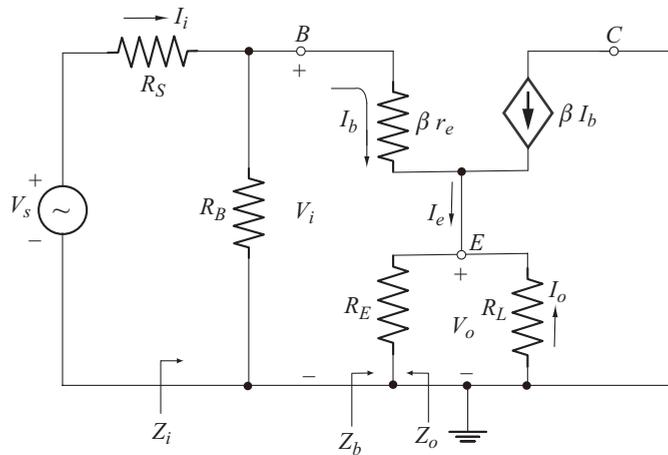
Fig. 3.83 Ac equivalent circuit using  $r_e$  model
