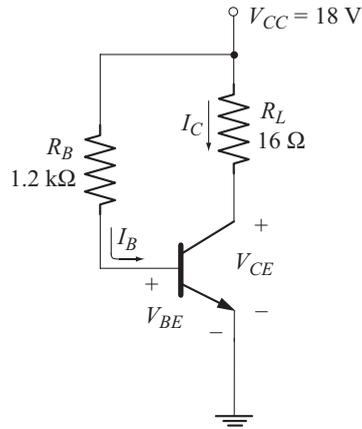
$$I_B = I_{BQ} = \frac{V_{CC} - V_{BE}}{R_B} = \frac{18 \text{ V} - 0.7 \text{ V}}{1.2 \text{ k}\Omega} = 14.42 \text{ mA}$$
