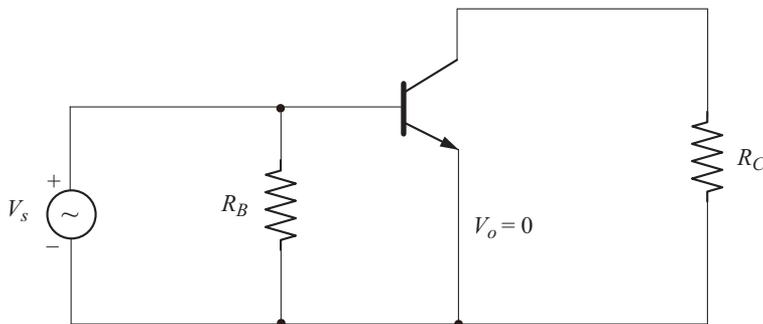
**Fig. 6.34** Input circuit obtained by short circuiting  $R_E$
