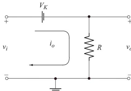
Fig. 1.19 Equivalent Circuit when the diode conducts
