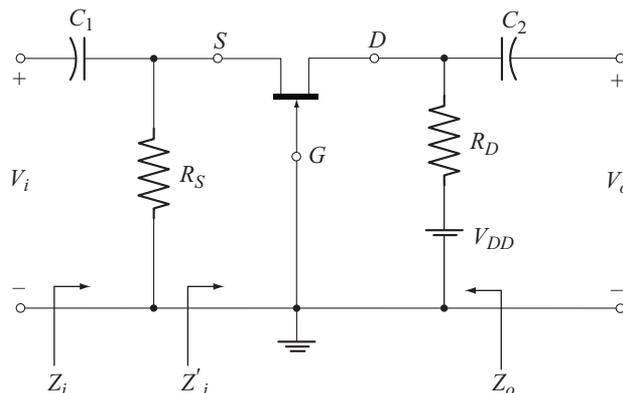
Fig. 9.28 JFET common-gate configuration
