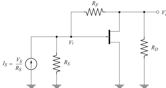
Fig. 6.47 Ac equivalent circuit of voltage-shunt feedback amplifier
