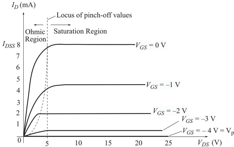
Fig. 9.4 Drain characteristics of FET
