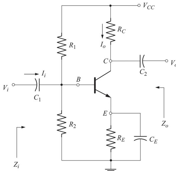
Fig. 3.40 CE configuration using voltage divider bias
