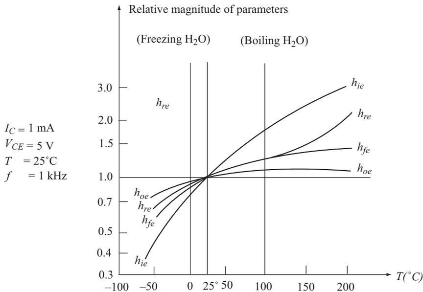
Fig. 3.22 Variation of CE  $h$ -parameters with temperature
