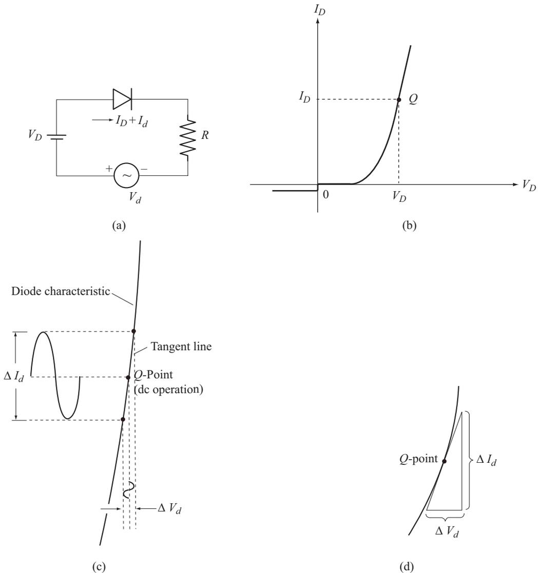
**Fig. 1.5** (a) Biased diode with ac input
