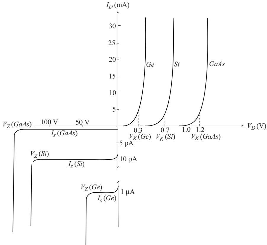
Fig. 1.2 Comparison of Ge, Si, and GaAs diodes
