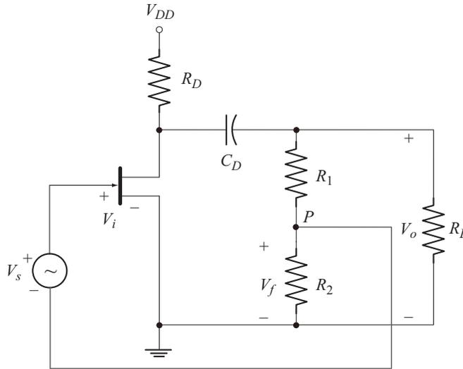
**Fig. 6.30** FET amplifier with voltage-series feedback
