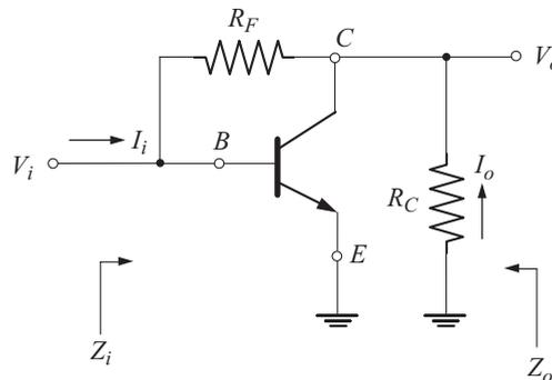
**Fig. 3.65** AC equivalent circuit
