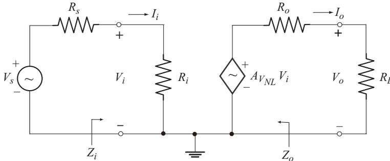
Fig. 3.89 Two - port system with  $R_s$  and  $R_L$
