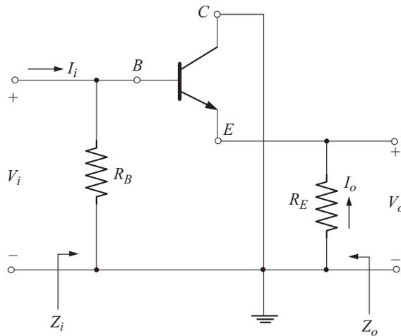
**Fig. 3.55** AC equivalent circuit
