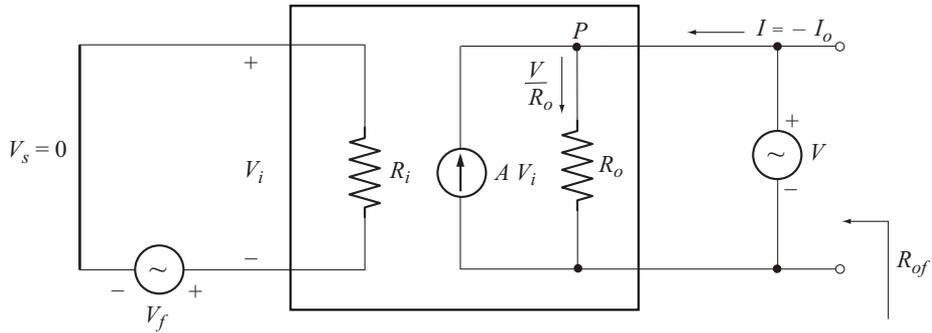
**Fig. 6.27** Output resistance of current series feedback amplifier
