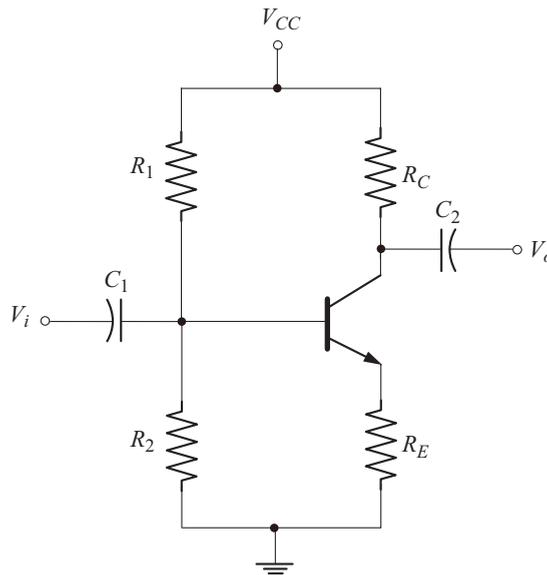
Fig. 2.13 Voltage divider bias or universal bias circuit
