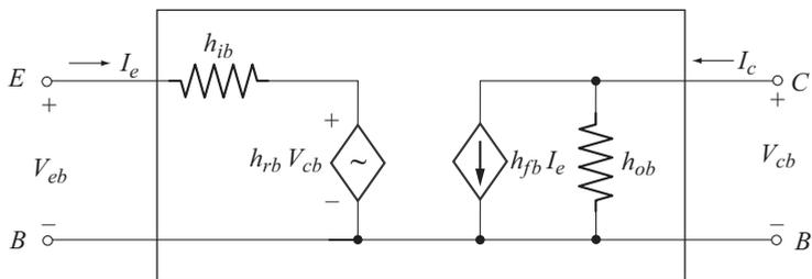
Fig. 3.15 Hybrid model of CB configuration
