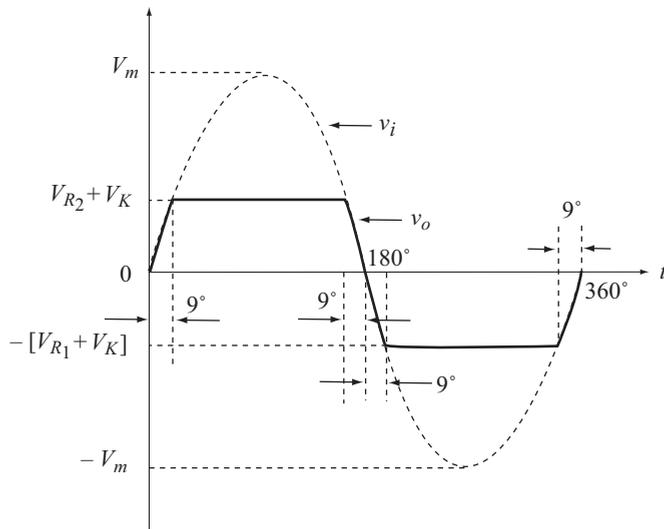
Observe that the sinusoid becomes flat at  $9^\circ$ . Value of  $v_i$  at  $\theta = 9^\circ$  is
