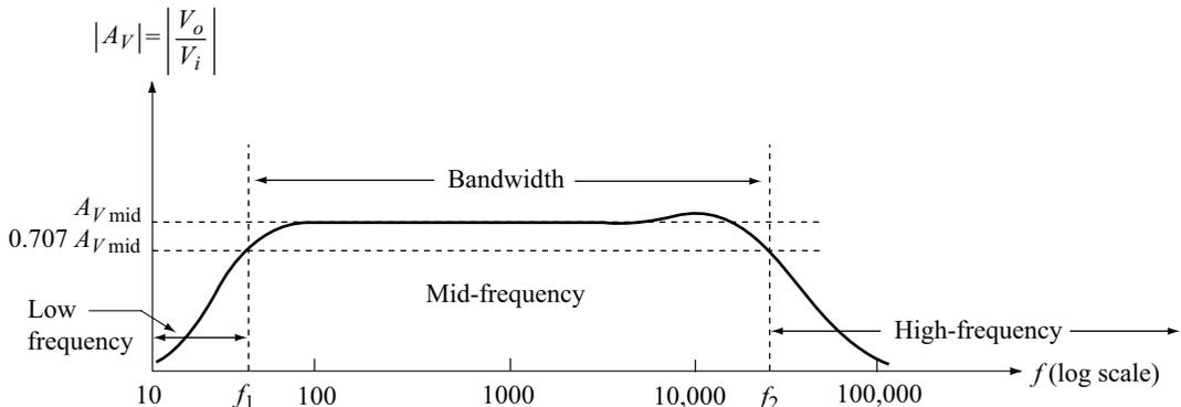
**Fig 4.2** Frequency response of transformer coupled amplifier
