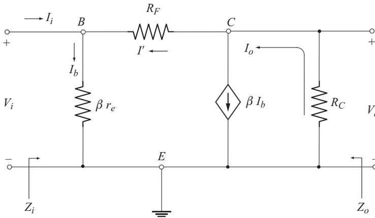
Fig. 3.66 AC Equivalent circuit with  $r_e$  model
