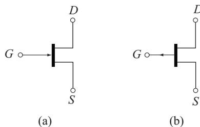
**Fig. 9.1** (a) Circuit symbol of  $n$ -channel FET
