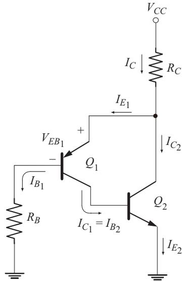
Fig . 5.11 DC biasing of feedback pair
