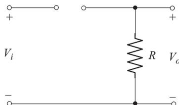
Fig. 4.8 Capacitor acts as open circuit at  $f = 0$
