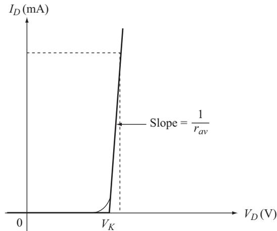
Fig. 1.7 Piece-wise linear characteristics of a diode
