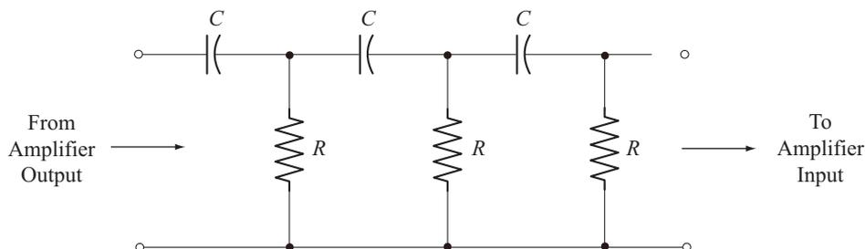
**Fig. 8.3** Feedback network in RC-phase shift oscillator
