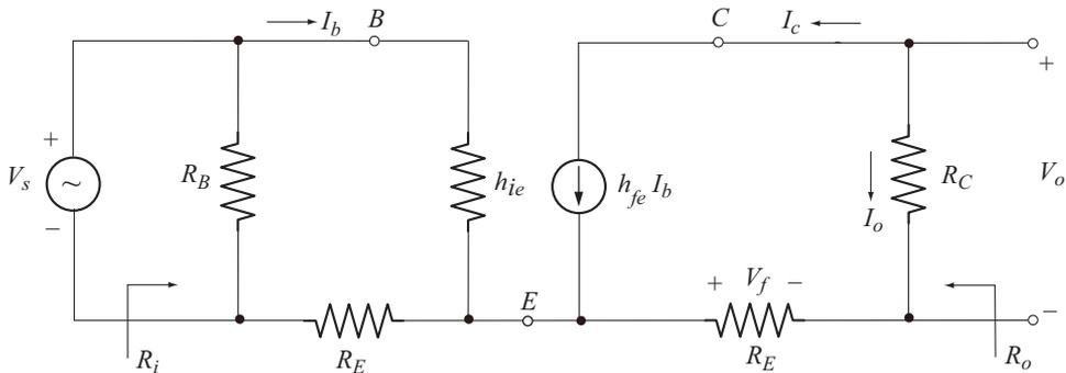
**Fig. 6.44** AC equivalent circuit using hybrid model
