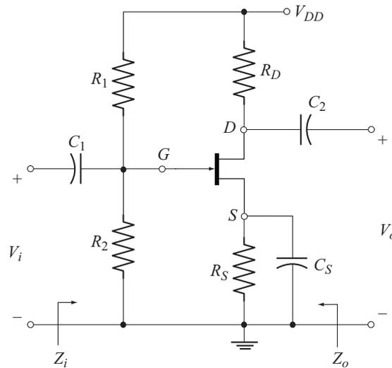
**Fig. 9.18** JFET common-source amplifier using voltage divider configuration
