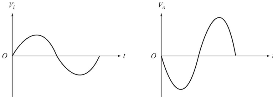
Fig. 3.39  $180^\circ$  Phase shift between  $V_i$  and  $V_o$
