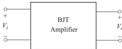
**Fig. 3.73** Defining no load voltage gain
