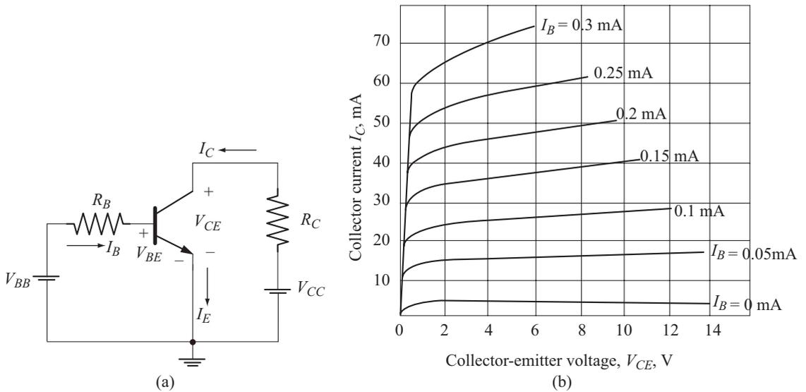
Fig. 2.1 The common-emitter configuration and its output characteristics
