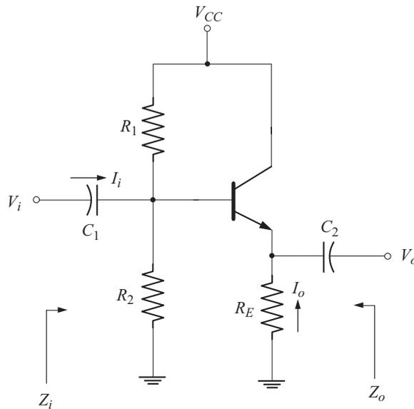
Fig. 3.59 Emitter follower using voltage divider bias
