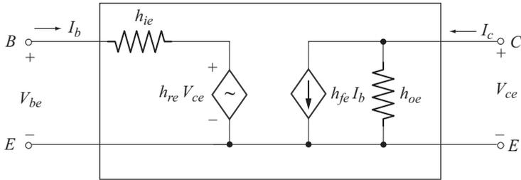
**Fig. 3.17** Hybrid model of CE configuration
