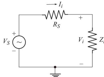
**Fig. 3.78** Simplified output equivalent circuit      **Fig. 3.79** Simplified input equivalent circuit
