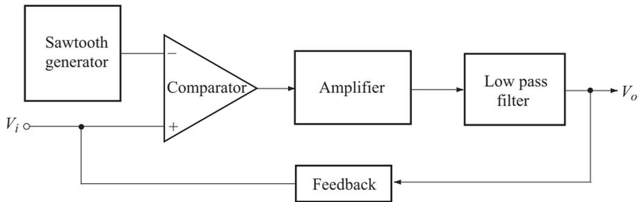
Fig. 7.24 Block diagram of class D power amplifier
