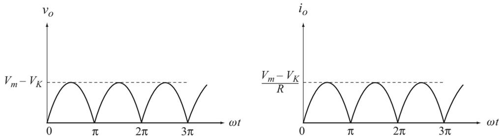
**Fig. 1.28** Wave forms of  $v_o$  and  $i_o$
