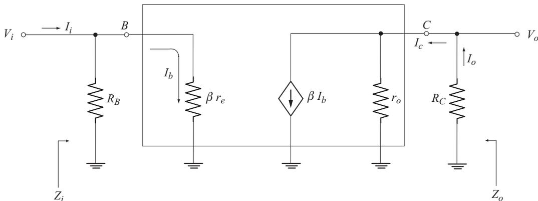
**Fig. 3.36** AC equivalent circuit with  $r_e$  model
