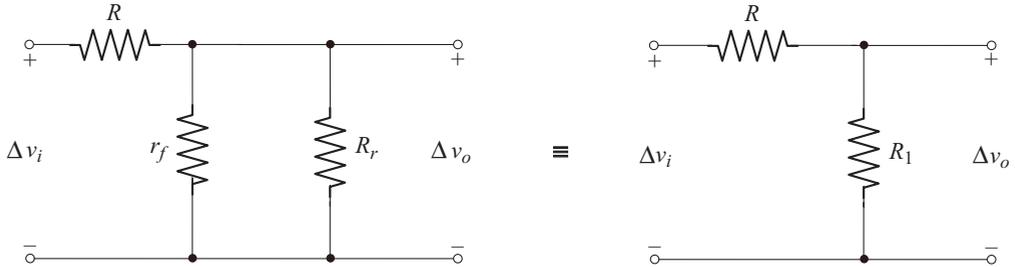
$$R_1 = r_f \parallel R_r = 0.1 \text{ k}\Omega \parallel 100 \text{ k}\Omega = 0.099 \text{ k}\Omega$$
