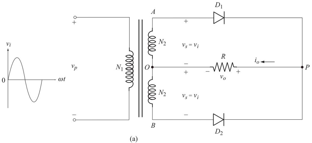
Fig. 1.26 Full wave rectifier with centre-tapped transformer
