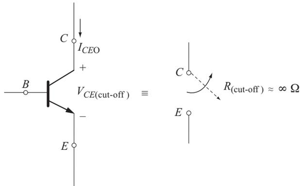
**Fig. 2.24** Representation of transistor when operating at cut-off
