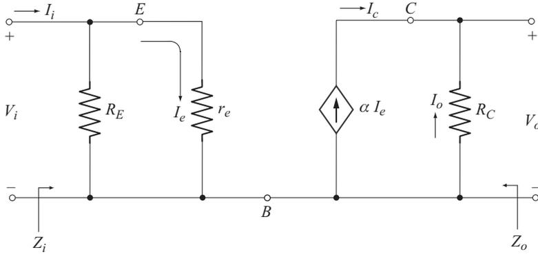
**Fig. 3.62** AC equivalent circuit with  $r_e$  model
