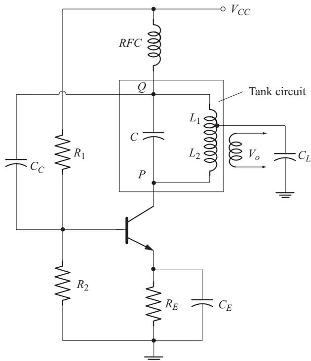
Fig. 8.10 Transistor Hartley oscillator
