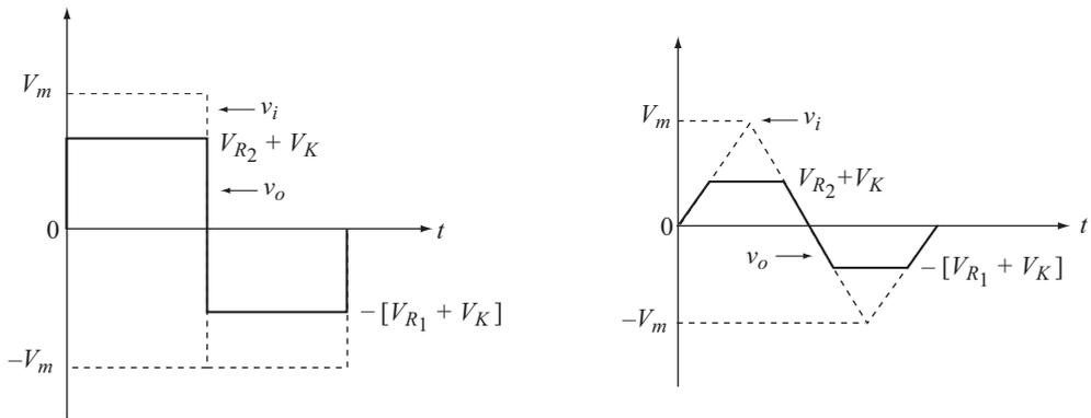
**Fig. 1.45** Output waveform for square and triangular inputs
