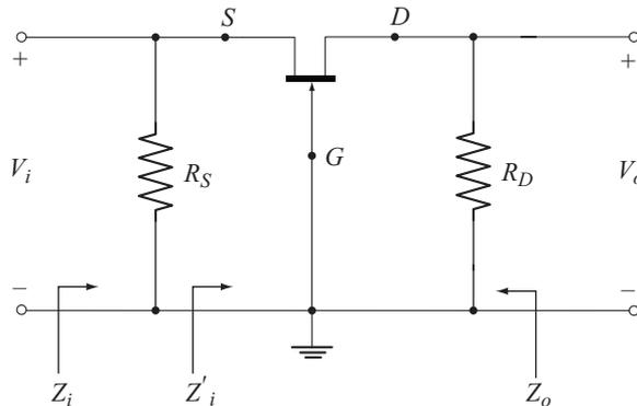
**Fig. 9.30** Ac equivalent circuit of common-gate configuration
