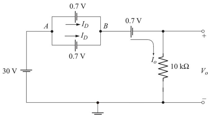
Voltage between points  $A$  and  $B$  is  $0.7\text{ V}$ .
