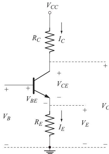
**Fig. 2.17** Collector circuit of voltage divider bias
