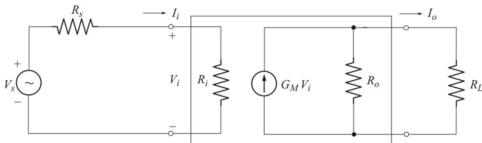
**Fig. 6.3** Equivalent circuit of transconductance amplifier
