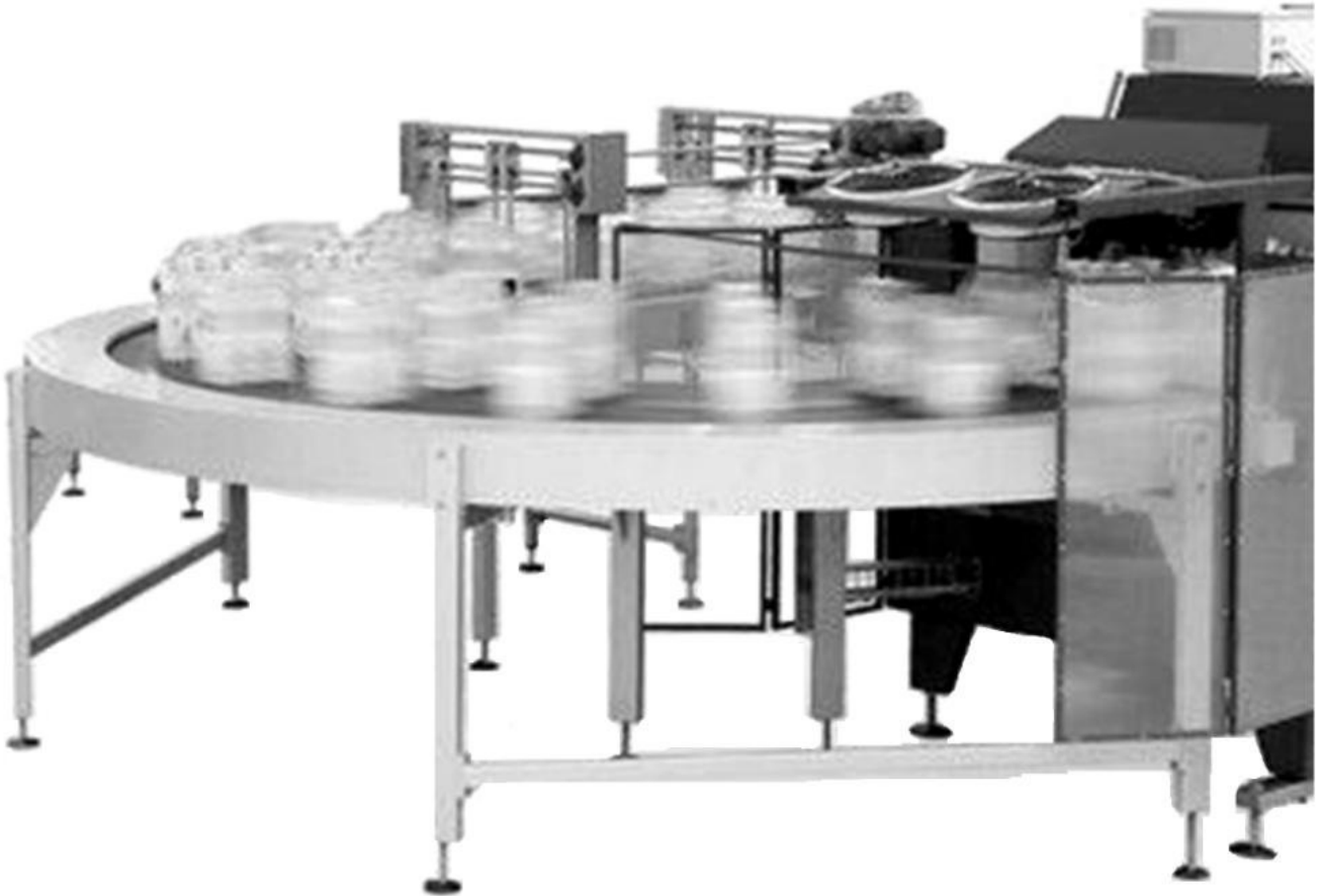
Figure 8.41: Bottle conveyor system
