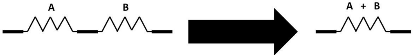
Figure 1.11: Series resistor rule
