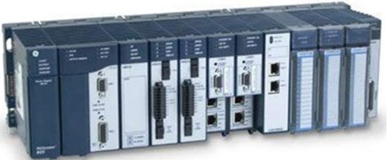
Figure 8.1: GE Programmable Automation Controller (PAC)
