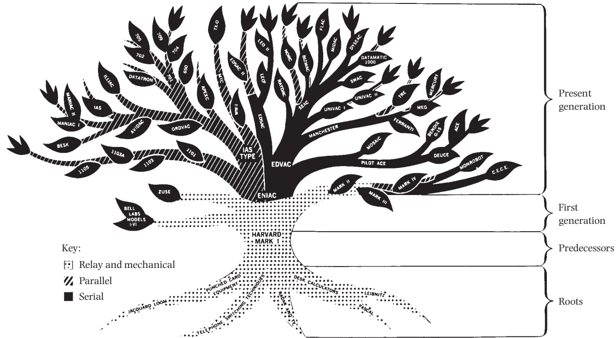
Fig. 1 The NSF 'family tree' of computer design. (Redrawn from the original 1957 diagram by Olwen Harrison and Jack Copeland.)
