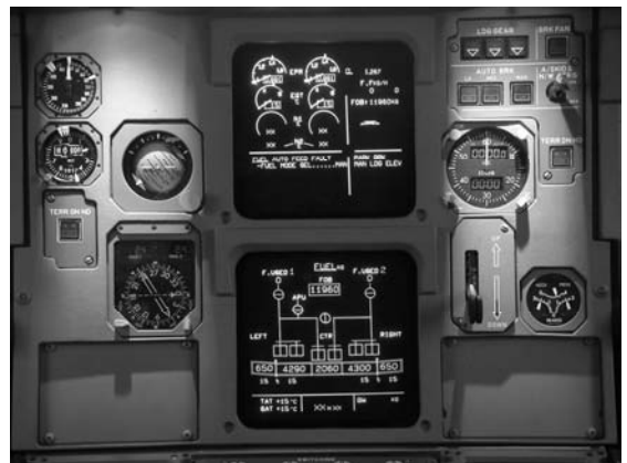
Figure 1.18 A320 ECAM displays located above the centre console between the captain and first officer
