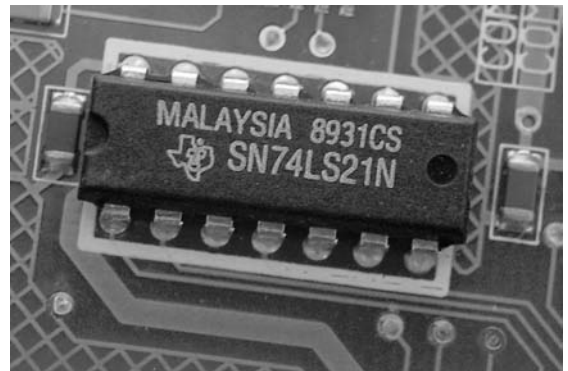
Figure 5.28 A low-power Schottky TTL logic circuit supplied in a 14-pin DIL package
