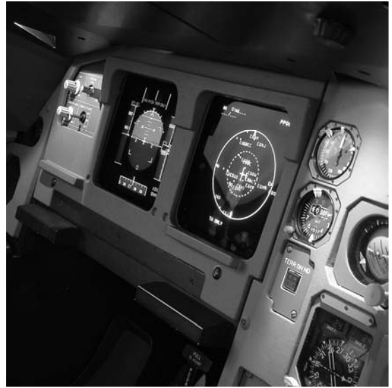
Figure 15.3 'Glass cockpit' (EFIS) displays in an A320
