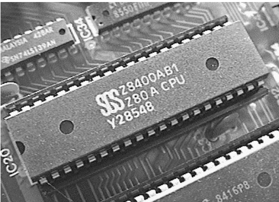
Figure 7.4 The Z80 is a basic 8-bit microprocessor supplied in a 40-pin dual-in-line (DIL) package. The chip operates from a single +5 V supply.
