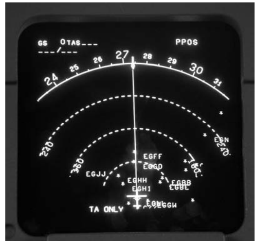
Figure 1.17 EFIS navigation display
