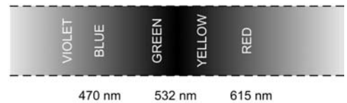
Figure 11.12 Typical spectral response for the human eye
