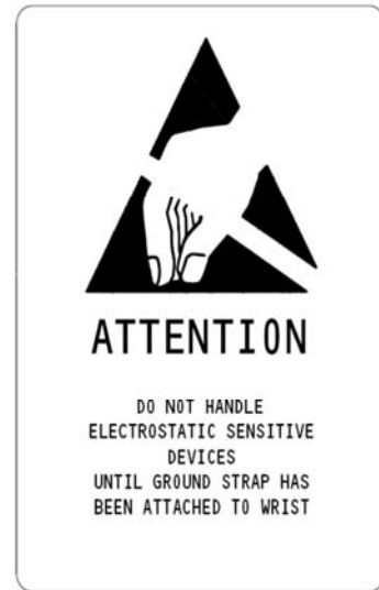
Figure 12.8 ESD wrist strap warning notice
