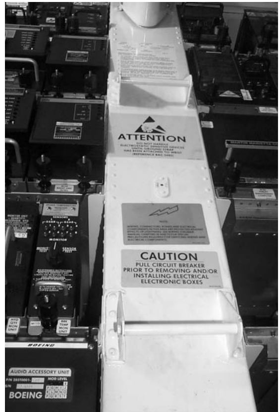
Figure 12.4 ESD warning notice (third from bottom) in the avionics bay of a Boeing 737
