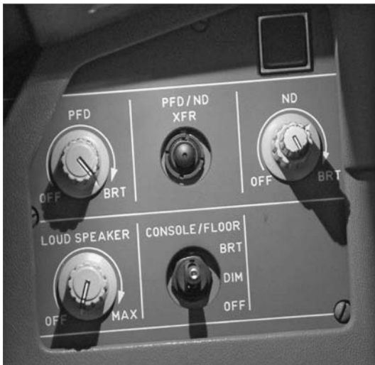
15.4 A320 PFD and ND brightness and transfer controls
