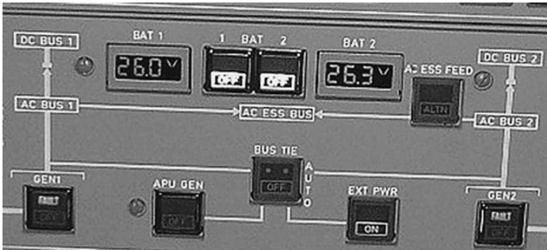
11.21 Three-digit seven segment displays used for battery bus voltage indication
