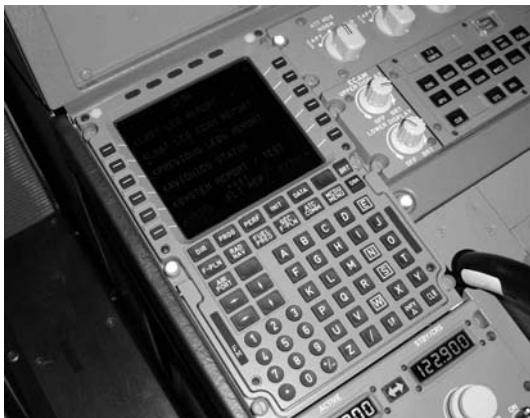
15.11 Typical Airbus FMC CDU
