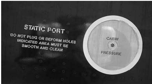
1.12 An aircraft static port
