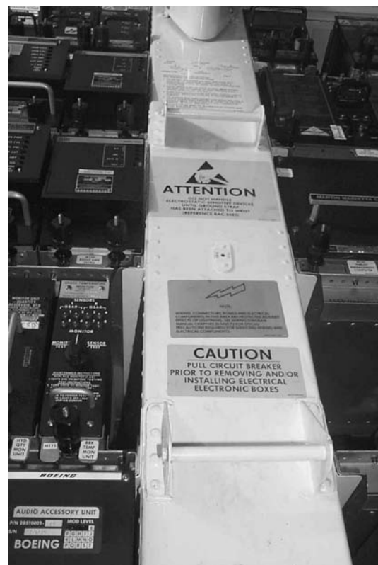
12.4 ESD warning notice (third from bottom) in the avionics bay of a Boeing 737
