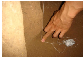
Fig. 9. The shear deformation of wheat-lime pile
