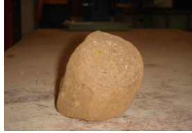
Fig. 8. Pile cement with the soil around pile
