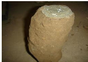
Fig. 10. Fly ash-lime pile cement with the soil around pile
