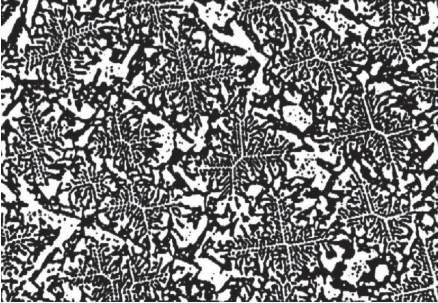
9.4 Micrograph of a transverse section of a uni-directionally solidified rod of mixture of magnetostrictive \text{CoFe}_2\text{O}_4 and piezoelectric \text{BaTiO}_3 , with an excess of \text{TiO}_2 (1.5 wt%). 2
