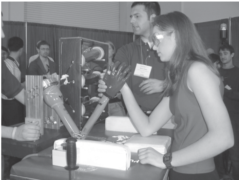
8.20 An EAP driven arm made by students from Virginia Tech and the human opponent, a 17-year-old student.
