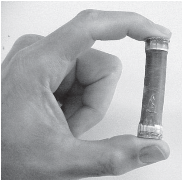
8.3 A dielectric elastomer EAP-based multifunctional electroelastomer roll (MER) spring roll. Courtesy of Qibing Pei, UCLA, Roy Kornbluh, SRI International, and SPIE (adapted from Pei et al. , 2002; and Kornbluh et al. , 2002).
