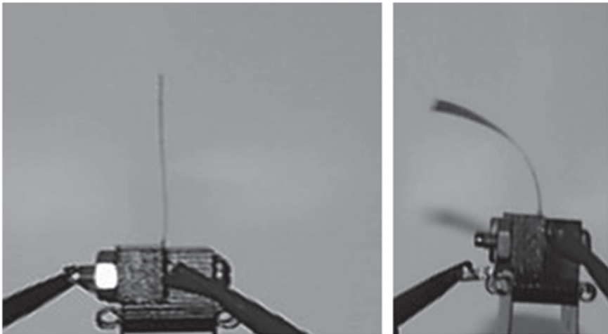
8.8 An electrostrictive grafted elastomer-based bimorph actuator in an unexcited state (left) and in one of the two directions of the excited state (right). Courtesy of Ji Su, NASA LaRC, VA.
