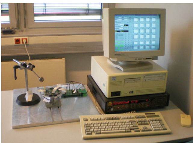
Fig. 1.20 Equipment for the calibration of the force-and-torque sensor
