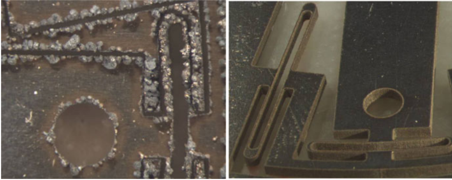
Fig. 1.7 Result of laser cutting of the transducer. To the left using standard laser cutting and to the right with water jet guided laser cutting
