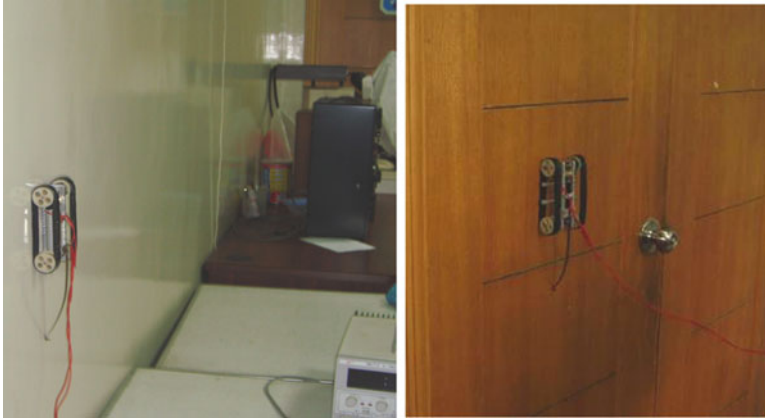
Fig. 9.11 The robot is climbing on a vertical wall and a wooden door
