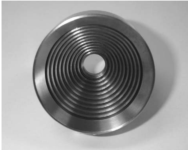
Figure 8-36 Conical corrugated horn antenna [23]. Reprinted with permission from John Wiley & Sons, Inc.
