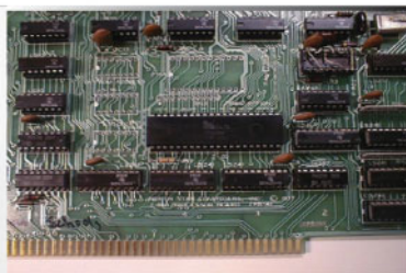
(c) Printed Circuit Board (NorthStar Horizon Z80 processor)
