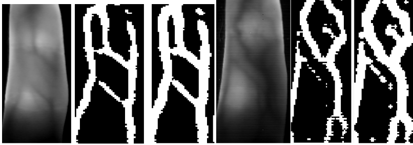
Fig. 4. Original, vein extraction and dilation images of two different fingers
