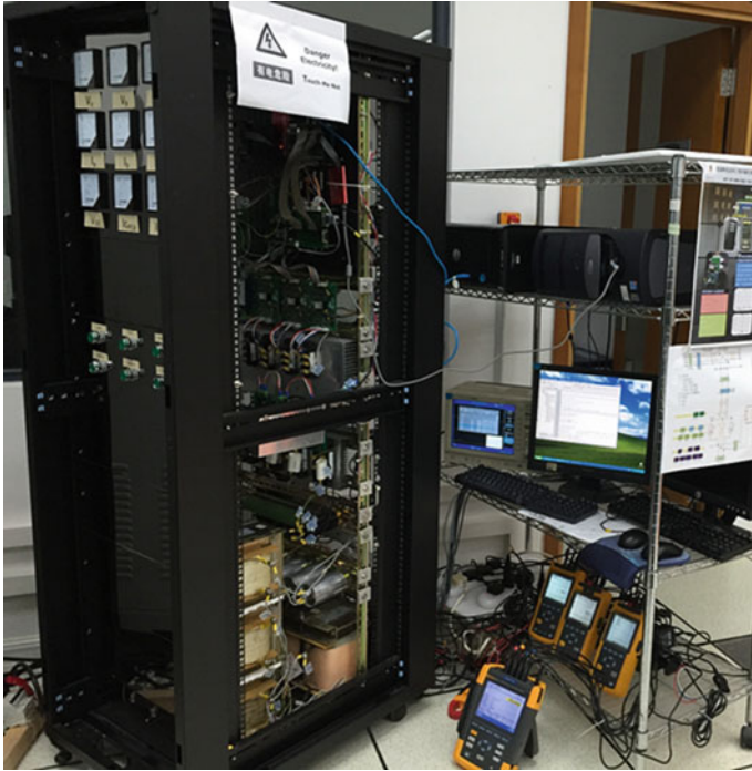
Fig. 9.2 Experimental setup of the 110 V-5 kVA TCLC-HAPF experimental prototype
