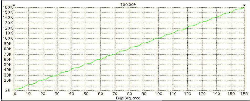
Fig. 4-4. Derived edge positions from curve fitting
