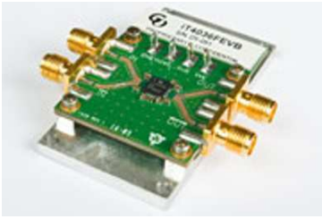
Fig. 5-10. Phase delay line iT4036 evaluation board (courtesy of GigOptix)
