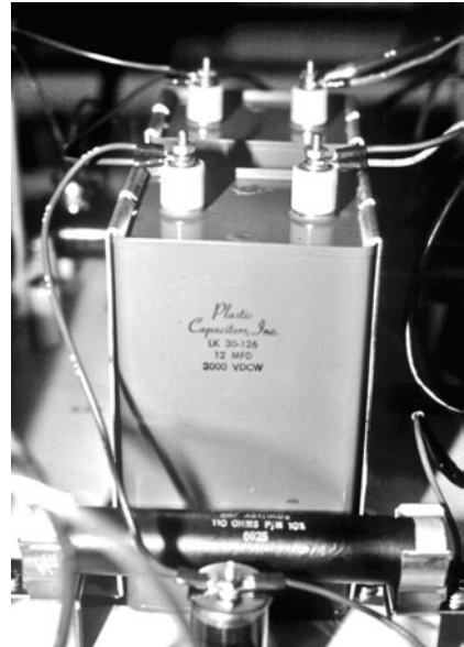
Figure 5.5 An oil-filled, high-voltage capacitor.
