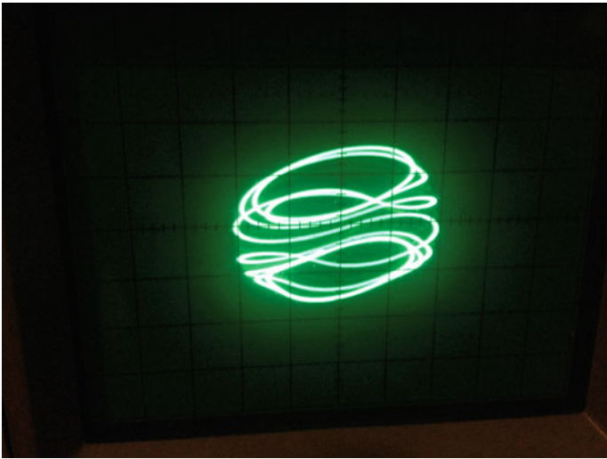
Fig. 4.22 Torus-breakdown route to chaos, as realized on the FPGA. Scales are 0.5 V/div on both channels
