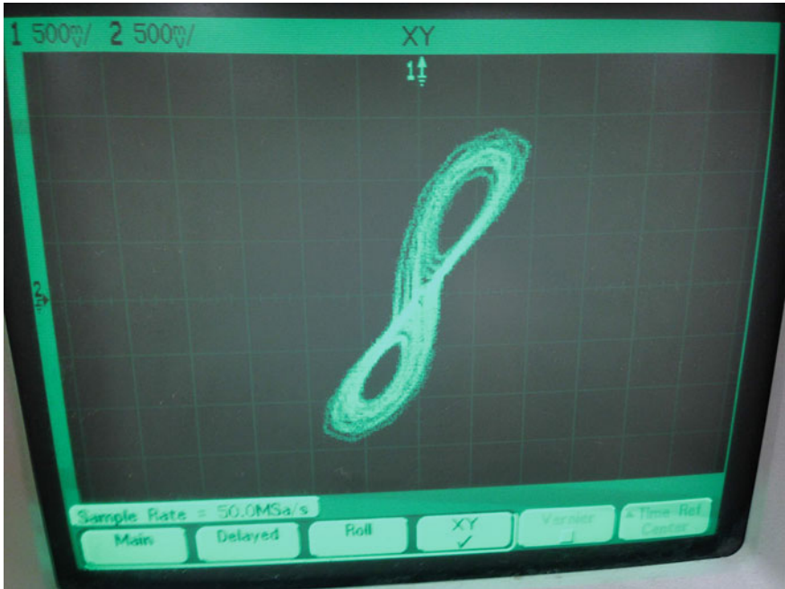
Fig. 3.6 y(t) versus x(t) Phase plot of the Lorenz attractor, the left (right) audio channel is on input X or channel 1 (input Y or channel 2) of the scope. Screen intensity has been set to 50%
