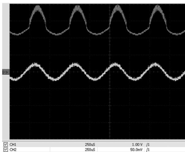
**Figure 10-27** Oscilloscope trace for AM on the laser
