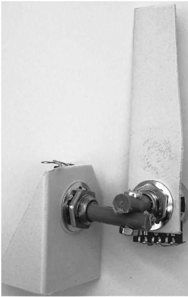
**Figure 4-6** The variable resistors attached to each other
