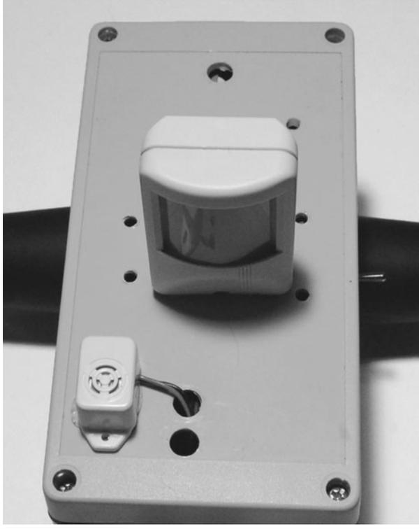
**Figure 15-16** The PIR sensor and buzzer attached to the box lid
