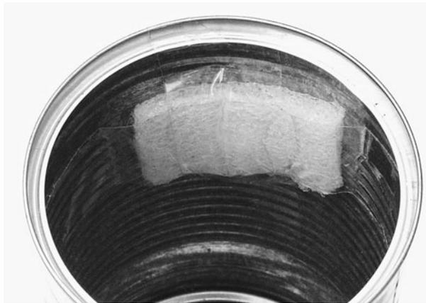
**Figure 5-26** Fitting the diffuser
