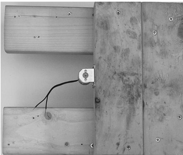
**Figure 8-31** A wooden base for the motor
