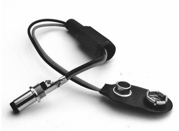
**Figure 8-23** The battery clip for the LED unit
