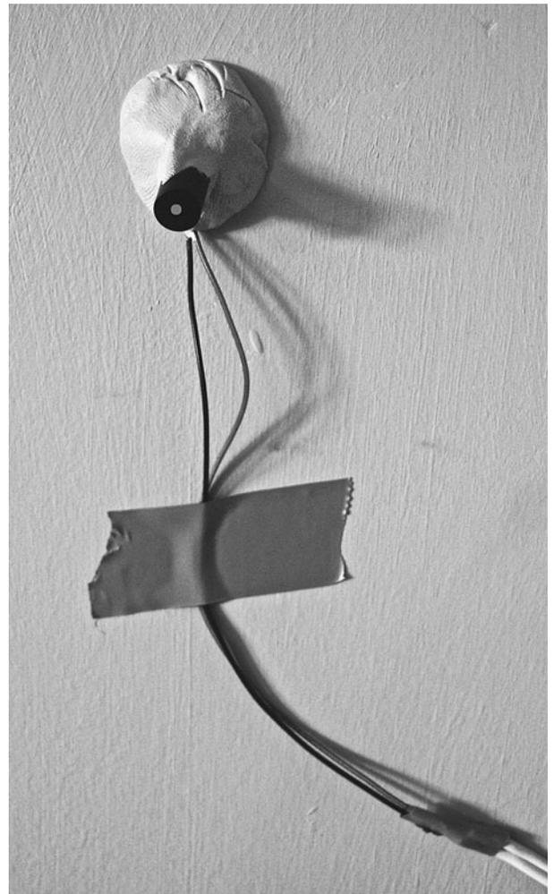
**Figure 7-12** Fixing the laser module to the wall
