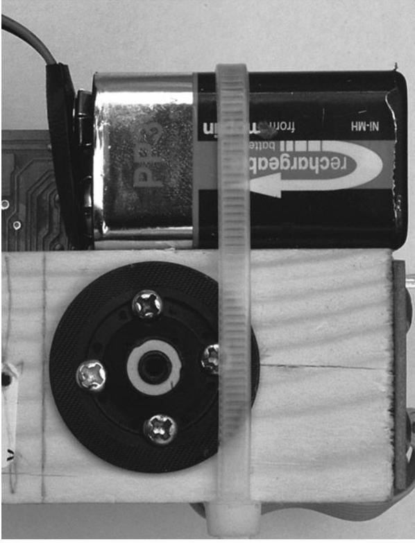
**Figure 8-33** Attaching the arm to the motor
