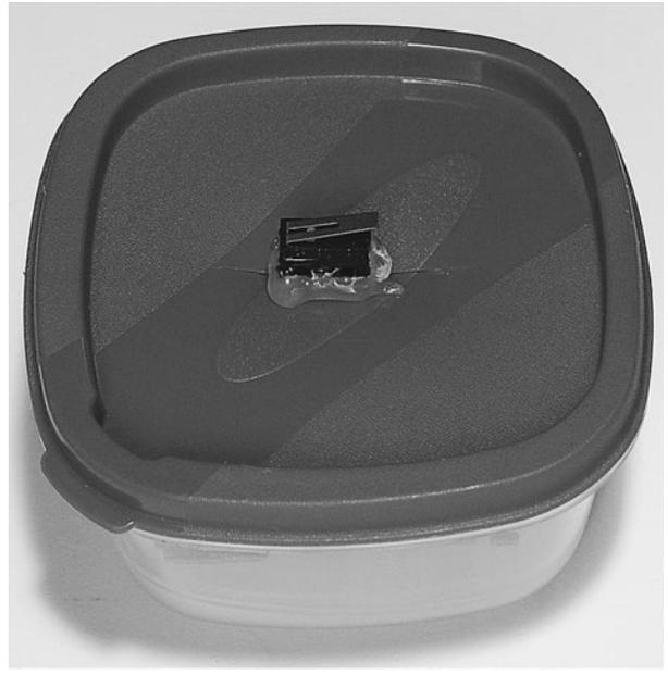
**Figure 11-8** The micro-switch attached to the box lid
