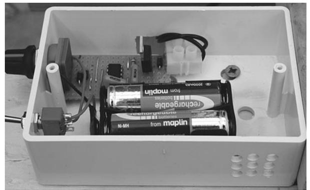
**Figure 8-32** The motor controller and batteries boxed
