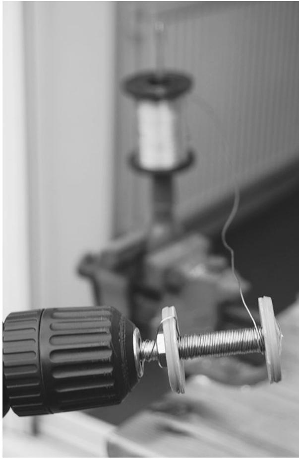
**Figure 13-4** Winding using an electric drill
