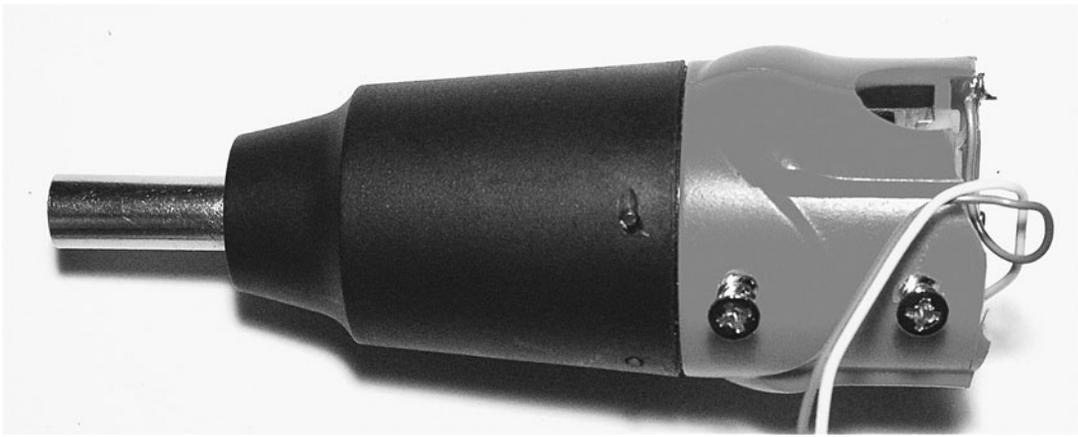
**Figure 15-10** Sawn-off screwdriver
