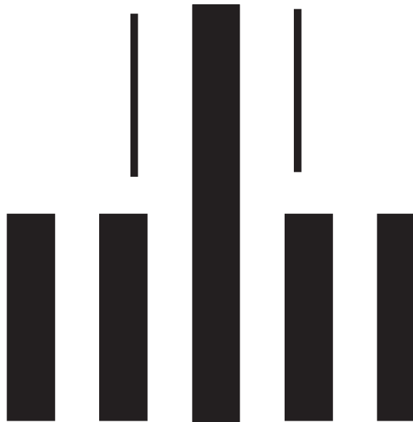
FIGURE 21.18 Layout with simple SRAF to compensate for iso-dense bias.
