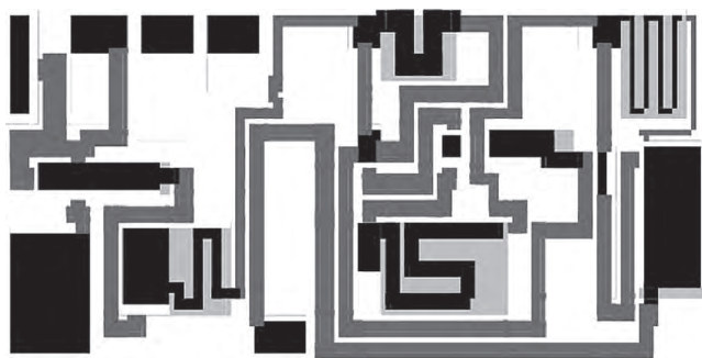
FIGURE 19.3 Microwave frequency (~60 GHz) device-level floorplan shows devices, planar wiring on a single layer, and several instances of “detours,” which are inserted to match lengths and electrical properties of wires in this small design. (From Aktuna, M. et al., IEEE Trans. CAD , 18, 375, 1999. With permission.)
