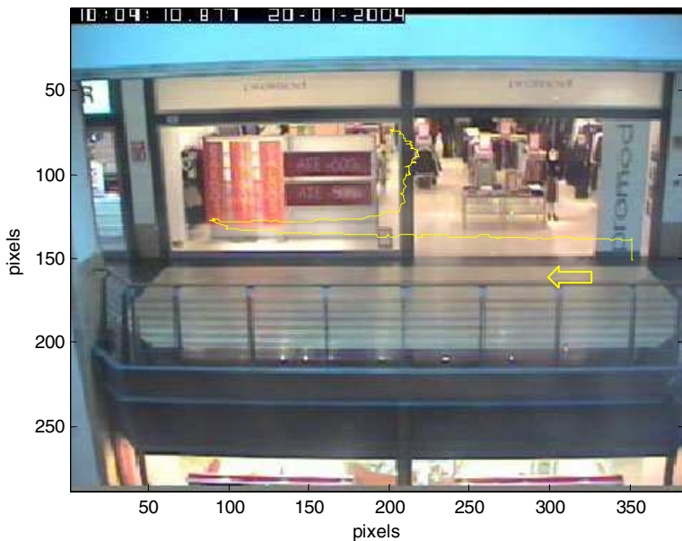
Fig 3. Trajectory of a person who approaches display window browses the window and then goes into the store
