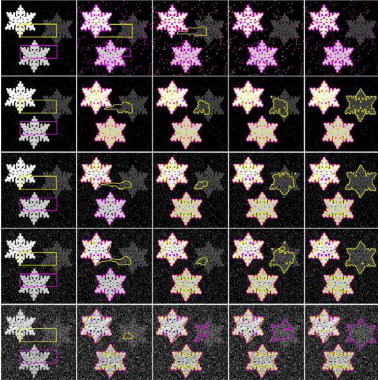
Fig. 6. The first row represents the evolution applying the MCV method [33] on the image with the noise density equaling 0.005, The second row to the fifth row represent the evolution applying the proposed method on the different images with the noise density 0.005, 0.05, 0.1 and 0.3 respectively. The noise adding into the image is the salt and pepper noise. The MCV method [33] is not robust against the noise even with the smallest noise density 0.005 in this experiment, but the proposed method is relatively robust against the noise. It can correctly segment the image, when the noise density increases to 0.3.
