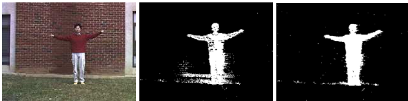
(a) original frame of a person in a red sweater (b) detection using MOG (c) detection using CB
