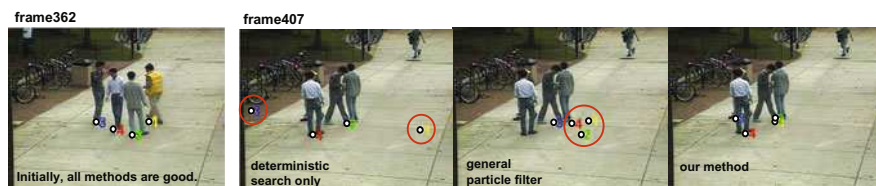
Fig. 14. Comparison on three methods: While the deterministic search with a single hypothesis (persons 2 and 4 are good, cannot recover lost tracks) and the general particle filter (only person 3 is good, insufficient observations during occlusion) fail in tracking all the persons correctly, our proposed method succeeds with a minor error. The view 2 was only shown here. The proposed system tracks the ground positions of people afterwards over nearly 1000 frames.
