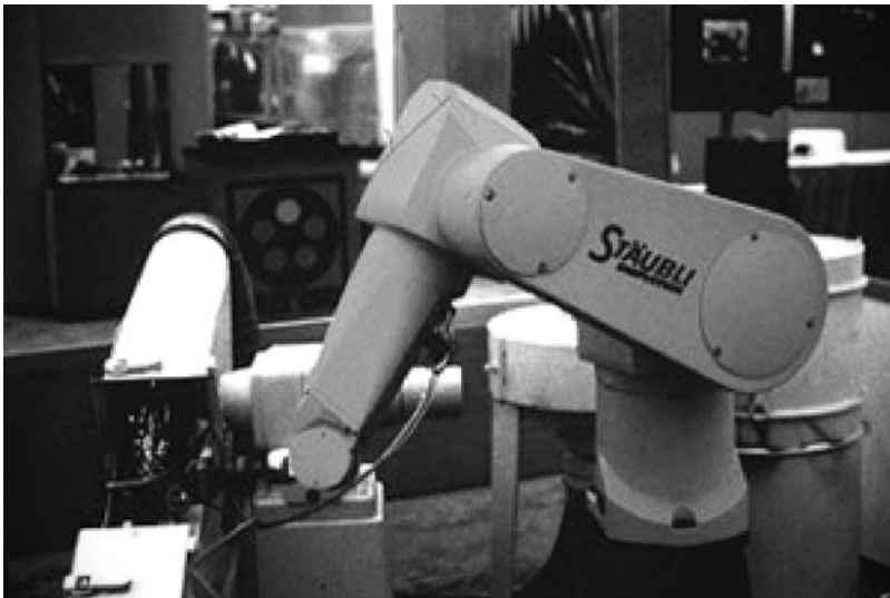
FIGURE 71.8 Articulated arm; six-axis arm grinding from a casting. (Courtesy of Staubli Unimation, Inc.)
