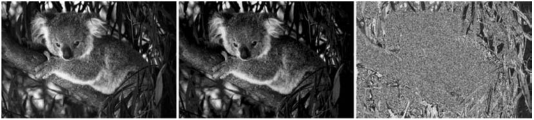
FIGURE 76.3 The original image is shown on the left, the quantized version with \kappa = 3 bits per pixel in the middle, and the difference image on the right. One can just begin to see artifacts in the lower left corner and in the details on the leaves.
