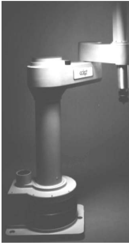
FIGURE 71.9 Type I SCARA arm. High-precision, high-speed midsized SCARA I. (Courtesy of Adept Technologies, Inc.)
