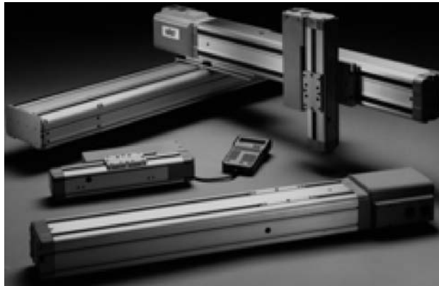
FIGURE 71.11 Cartesian robot. Three-axis robot constructed from modular single-axis motion modules. (Courtesy of Adept Technologies, Inc.)
