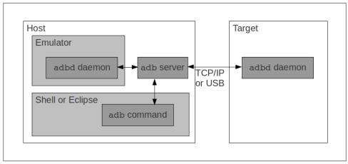
Figure 3-3. How ADB's parts are interconnected
