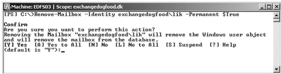
Figure 3.51 Permanently Removing a User Mailbox
