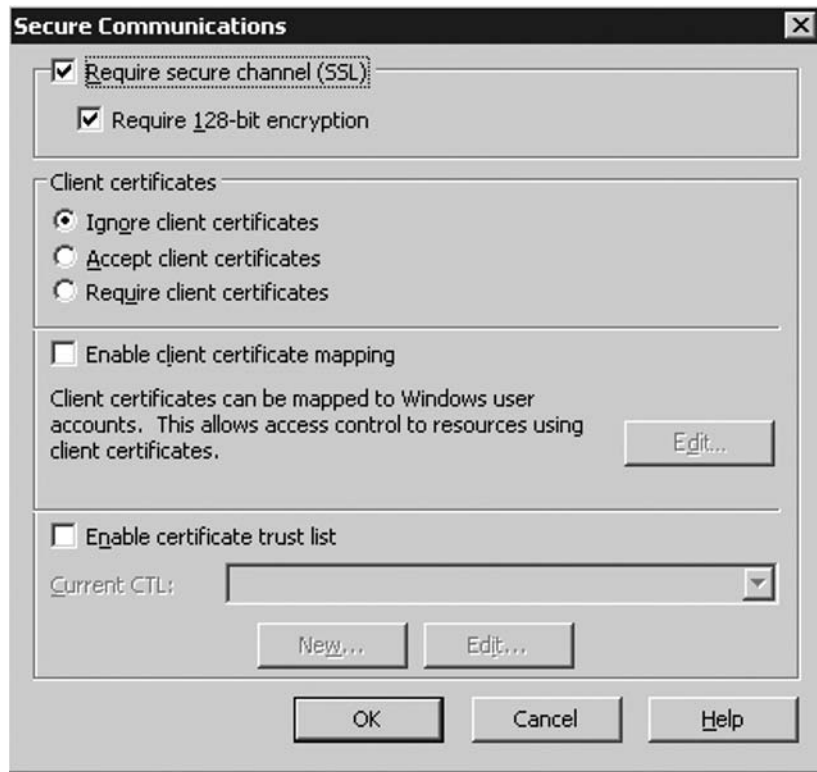
Figure 5.13 Enabling SSL on the Default Web Site
