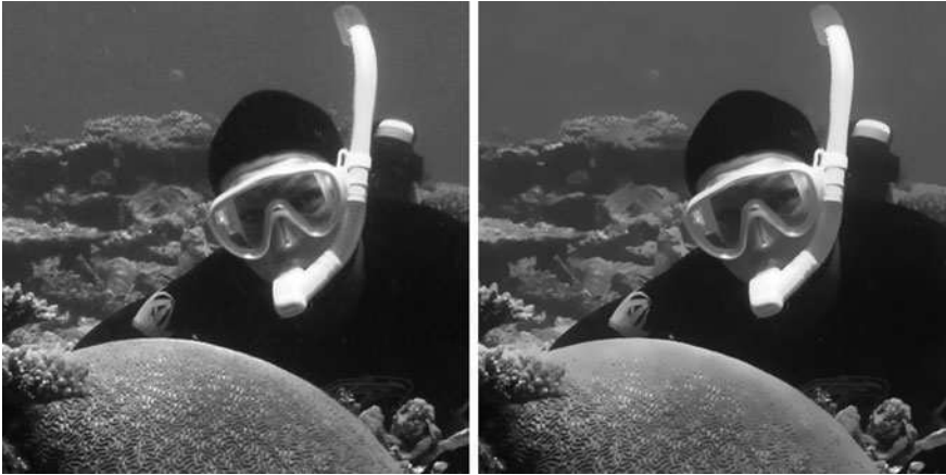
Fig. 13.3 Fragment of an underwater image 733 \times 740 pixels with a large number of suspended particles and the result of application of the edge preserving smoothing filter with the radius r = 12 , subject to intensity constraint K(p) = I_p \pm I_p \cdot 0.09
