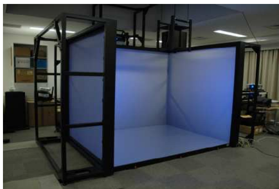
Figure 6.1 Immersive projection display K-Cave
