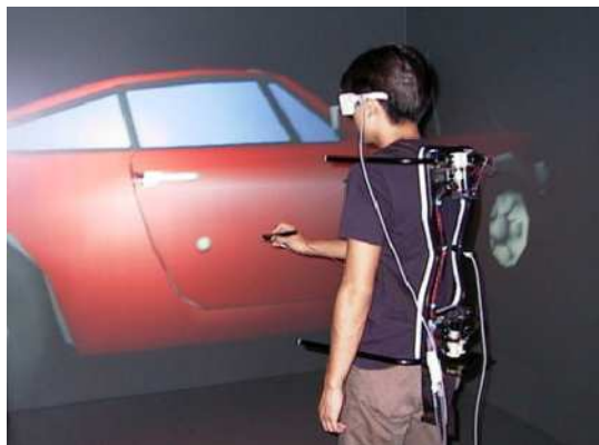
Figure 6.4 Wearable force feedback device HapticGEAR
