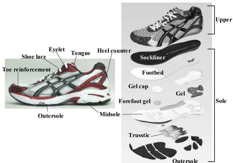
Figure 19.1 Running shoe construction with names of parts
