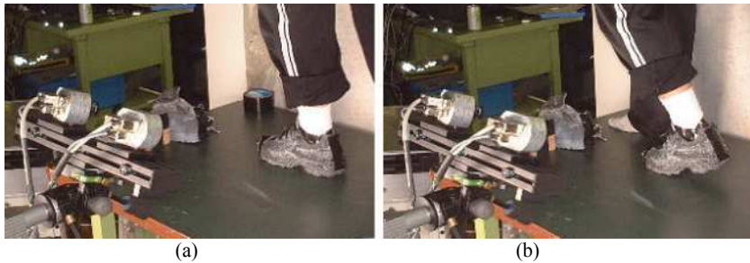
Figure 19.12 Photograph of CCD camera configuration: (a) foot flat condition, and (b) heel rise condition
