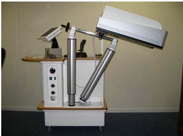
Fig. 12. Showing the side view of Prototype #2 with an adjustable viewing display on articulated specialist arm
