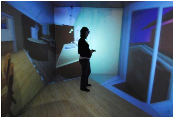
Fig. 2. A user immersed in the kitchen of a virtual reality apartment in a 6-wall retro-projected immersive room (often referred to as a CAVE™).
