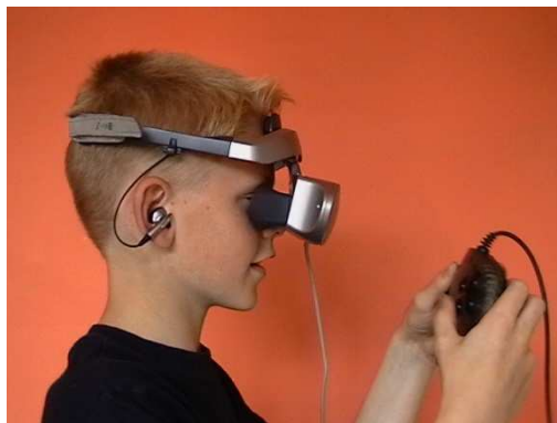
Fig. 1. Cy-Visor DH-4400 a binocular headset worn by a 9-year old child (reproduced with parental permission)
