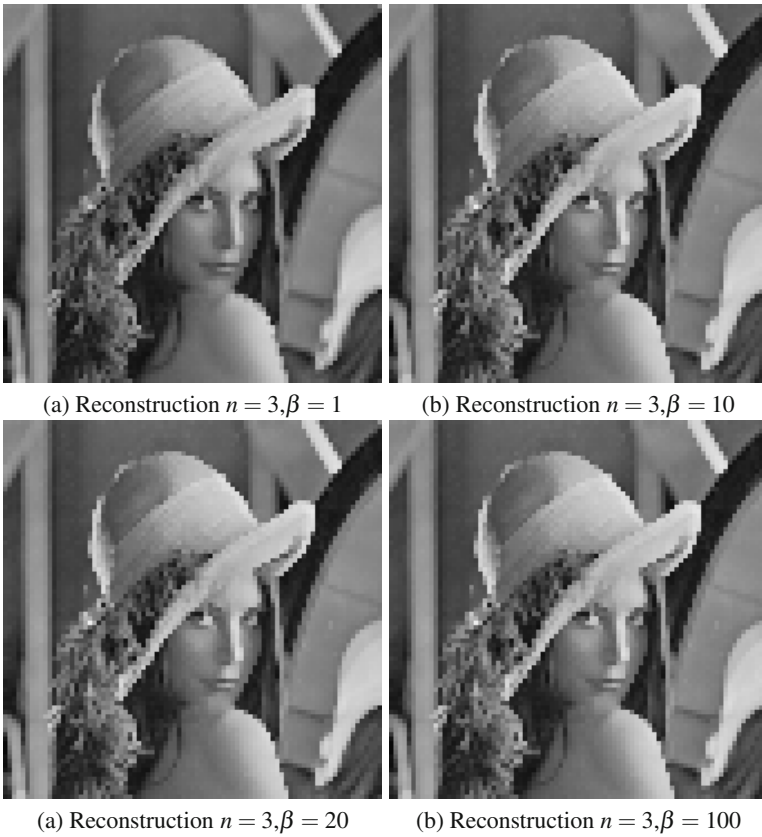
Fig. 7 Reconstructions of Lena image using the first algorithm of compression and BADD-OWA operators. Compression block size n = 3 .
