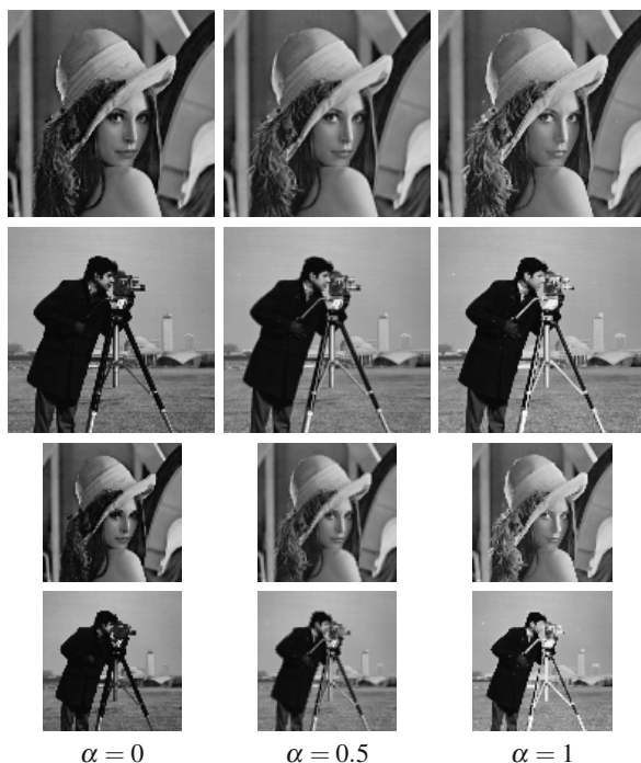
Fig. 2 Compression of Lena and Camera images with ME-OWA operators and compression block size n = 2 and n = 3
