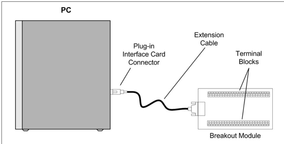
Figure 7-13. PC interface card breakout module example
