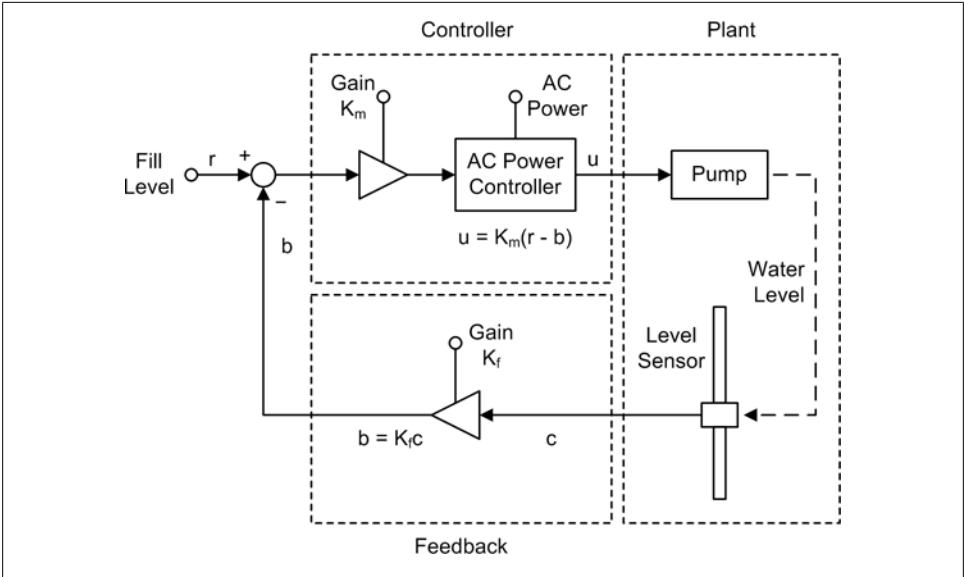
Figure 9-11. Closed-loop water tank control system details
