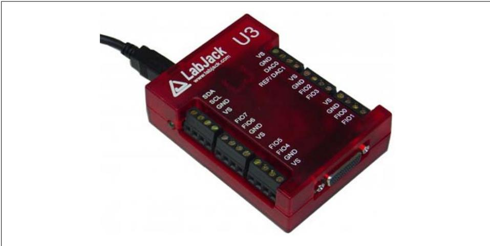
Figure 14-6. LabJack U3 USB DAQ device
