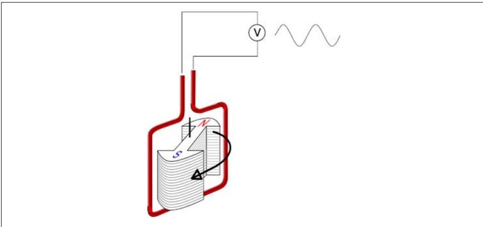
Figure 2-21. AC generator (image by Egmason, Wikipedia Commons, under the Creative Commons Attribution 3.0 Unported license: [http://commons.wikimedia.org/wiki/File:Alternator\\_1.svg](http://commons.wikimedia.org/wiki/File:Alternator_1.svg))
