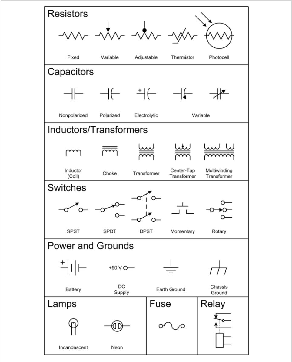
Figure 2-5. Common electronic schematic symbols
