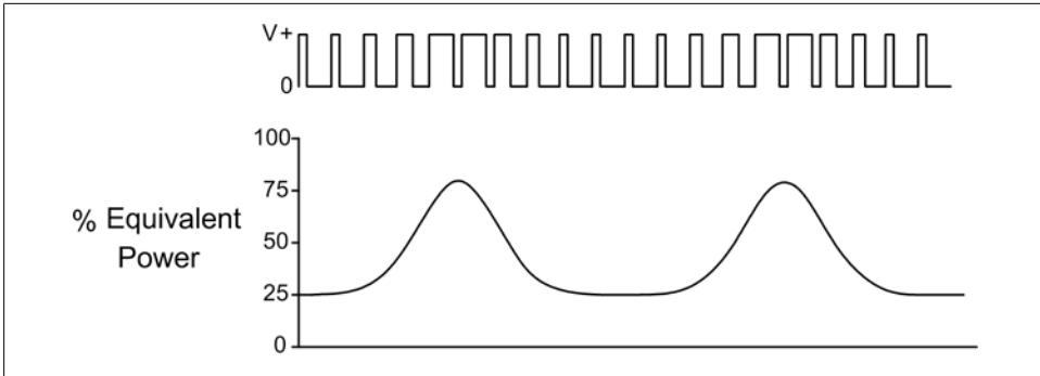
Figure 2-35. Pulse-width modulation
