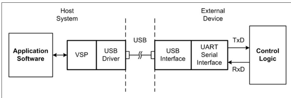
Figure 7-34. USB-to-serial interface
