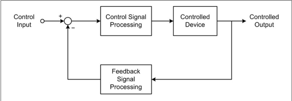
Figure 1-6. Closed-loop control
