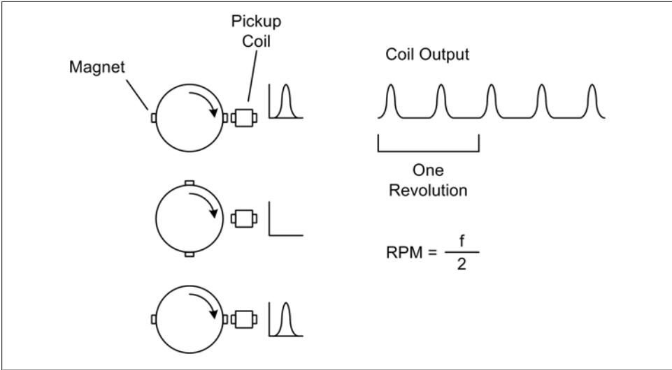
Figure 2-22. Electromagnetic tachometer
