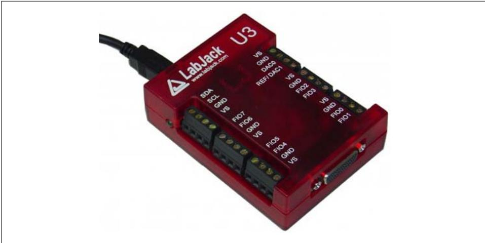
Figure 7-32. LabJack USB interface device
