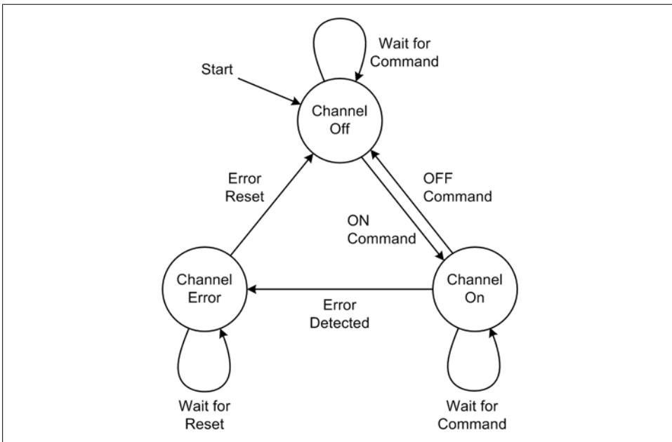
Figure 8-9. Example state diagram
