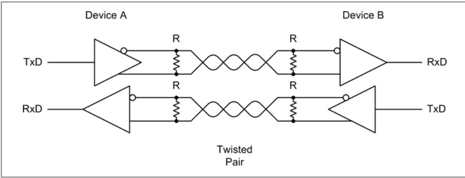
Figure 7-25. RS-485 interface drivers in four-wire mode
