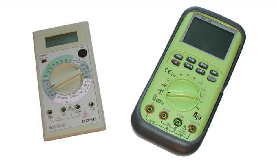
Figure 6-3. Digital multimeters
