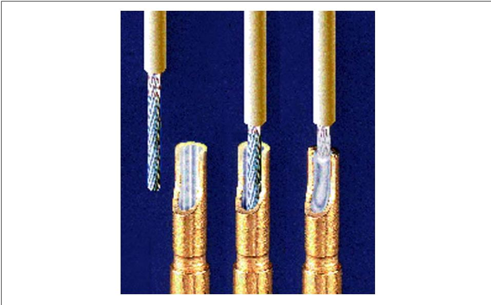
Figure 7-14. Solder cup connection (image credit: NASA)
