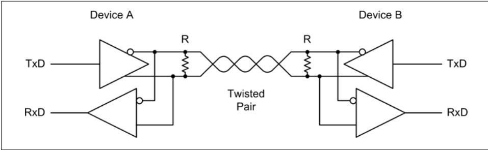
Figure 7-24. RS-485 interface drivers in two-wire mode
