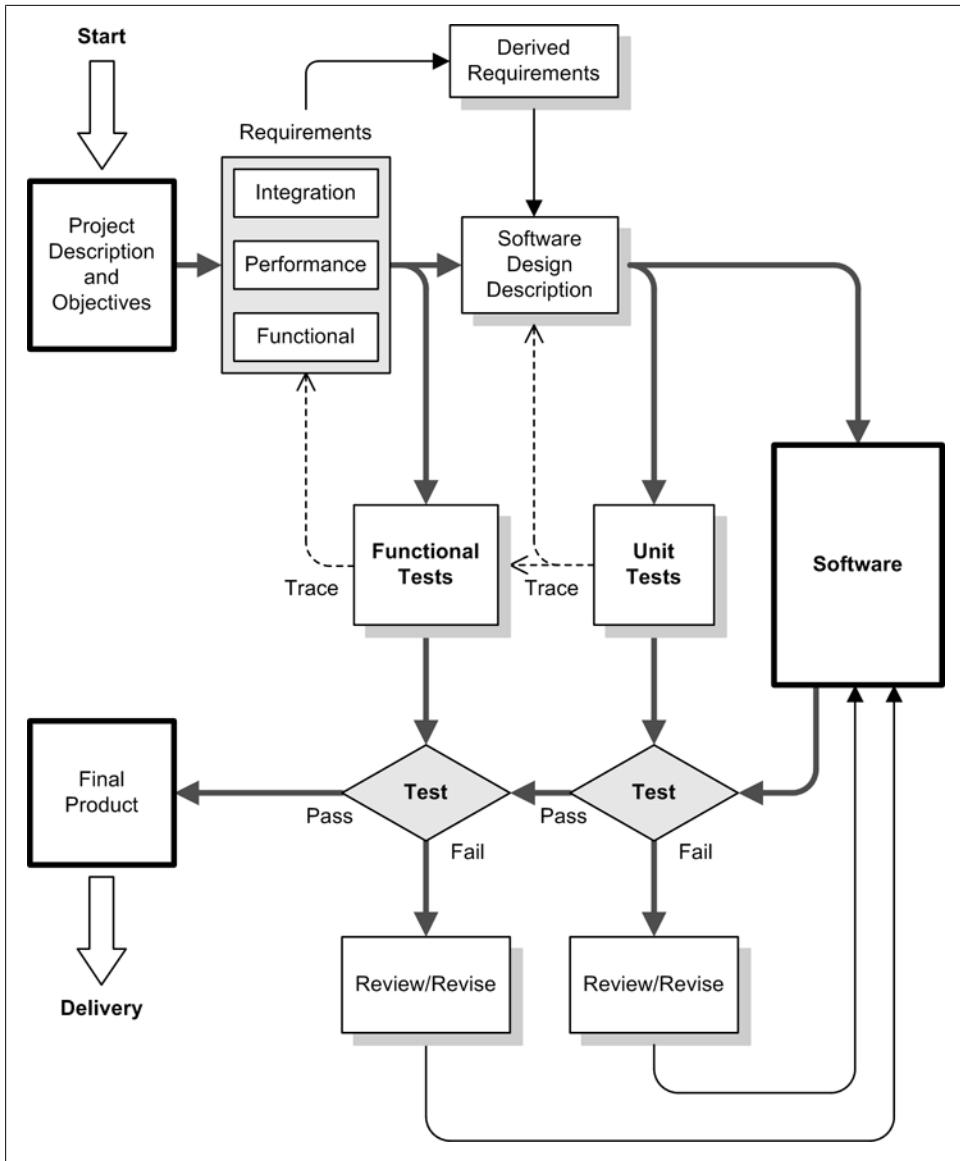
Figure 8-4. Software requirements in the development flow
