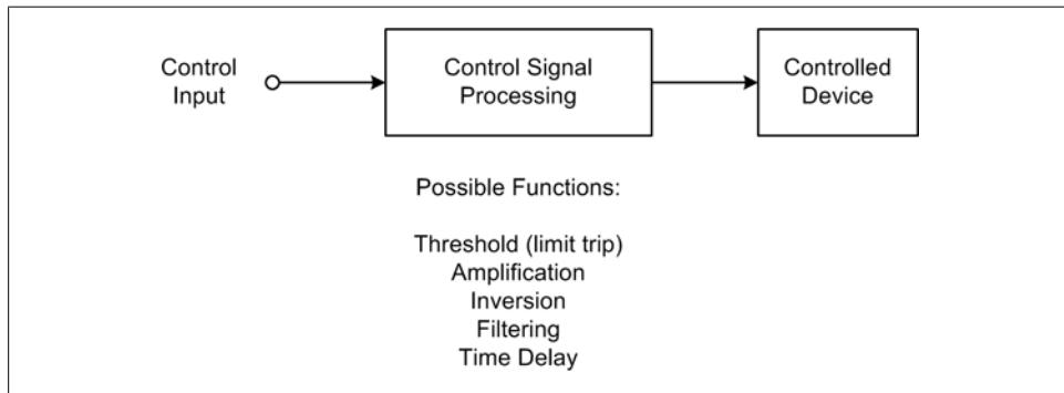
Figure 1-3. Open-loop control
