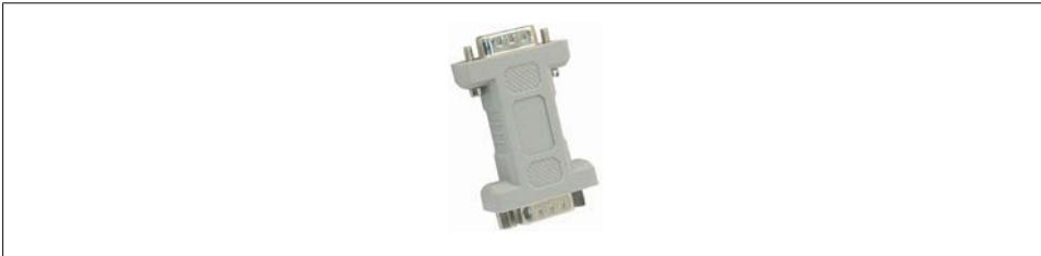
Figure 7-22. DB-9 null-modem adapter
