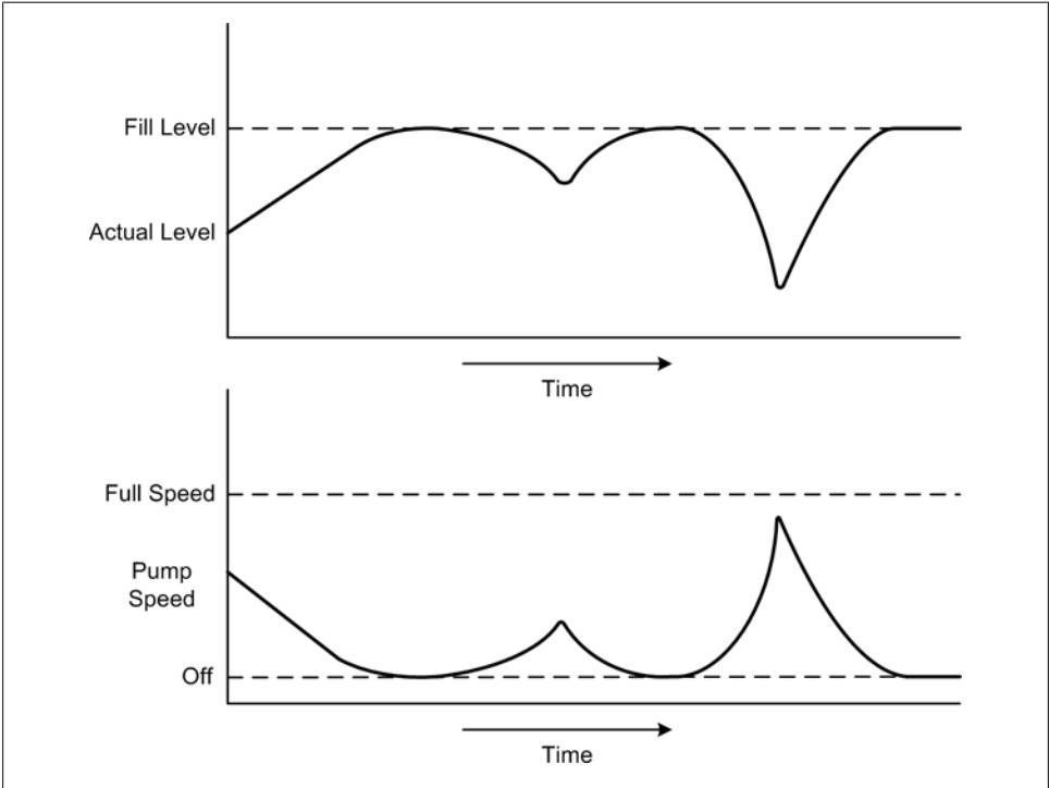
Figure 9-12. Water tank control system response graphs
