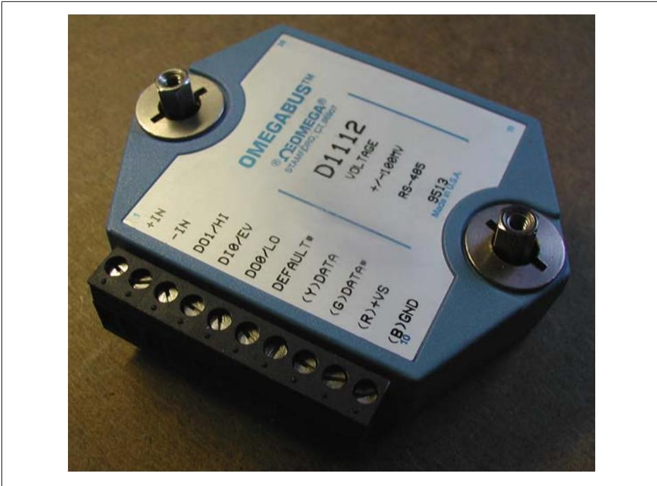
Figure 14-3. Omega D1112 RS-485 data transmitter
