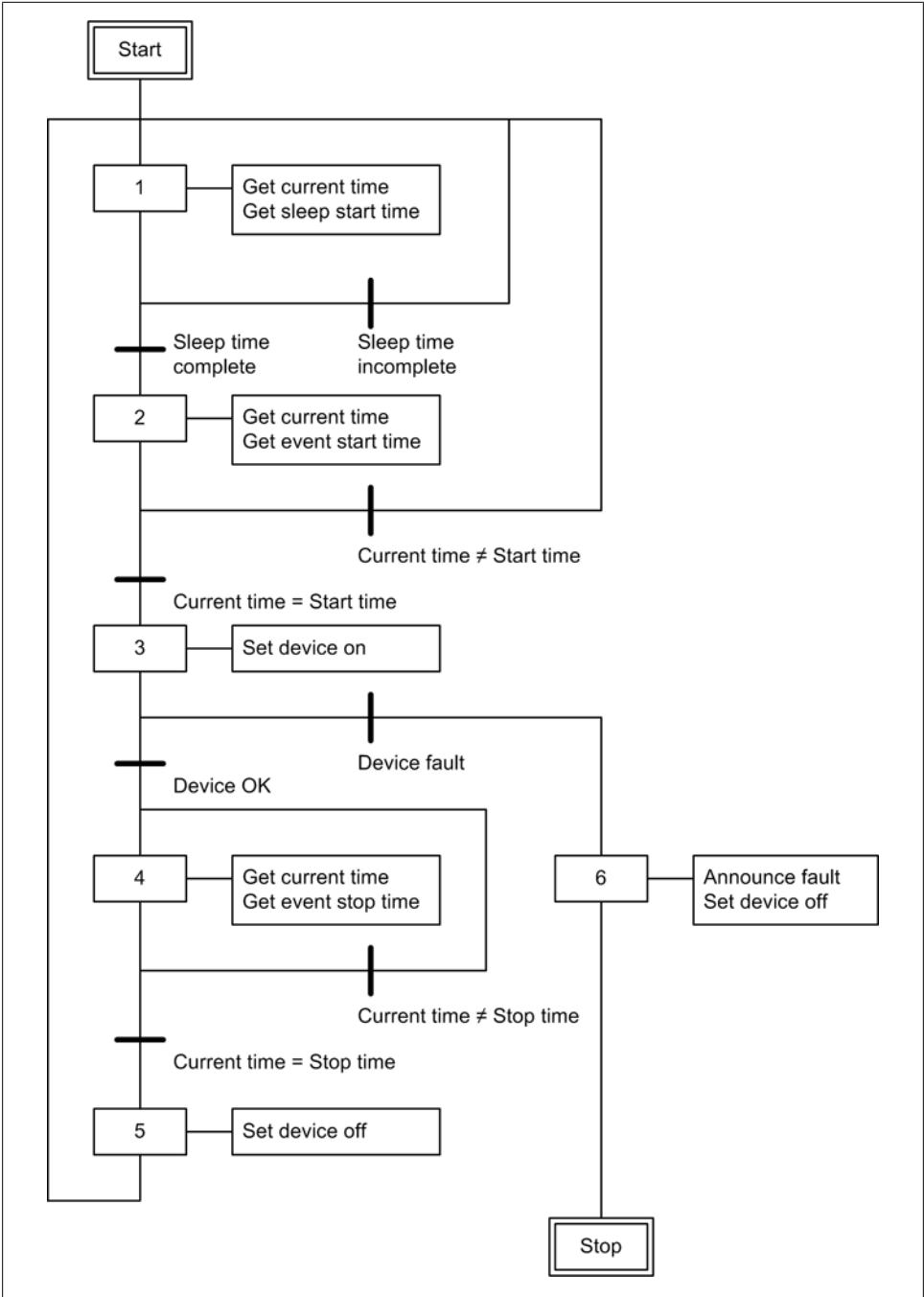
Figure 9-23. Example SFC diagram
