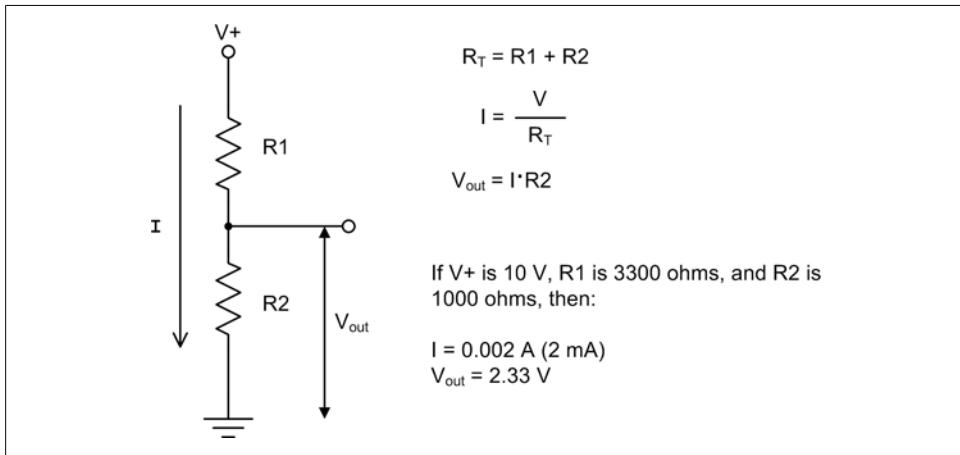
Figure 2-13. Voltage divider
