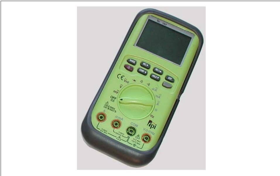
Figure 14-1. tpi model 183 DMM
