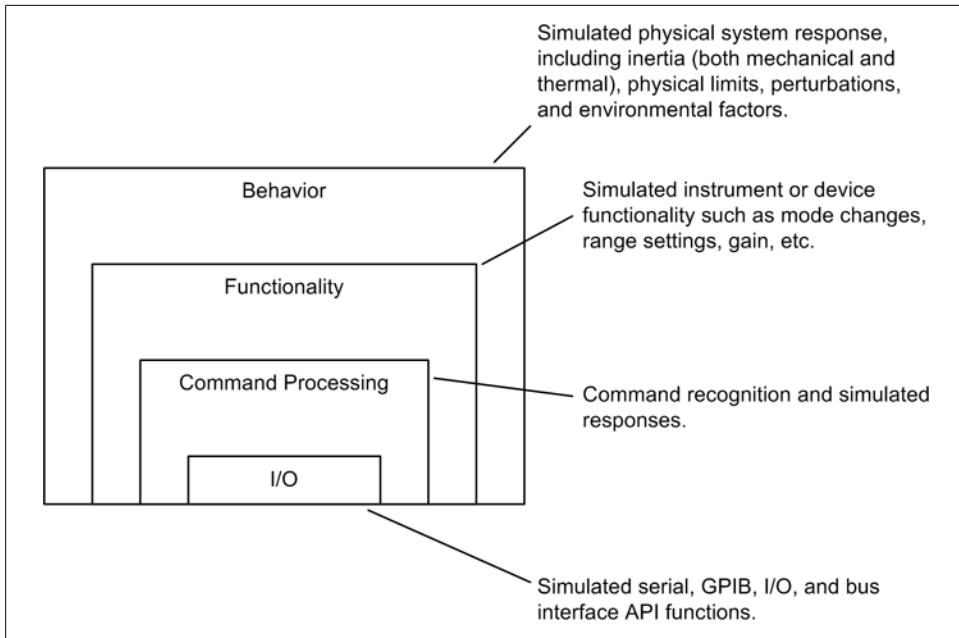
Figure 10-16. Simulation levels
