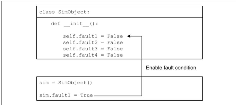
*Figure 10-4. Simulator fault injection using object variables*
