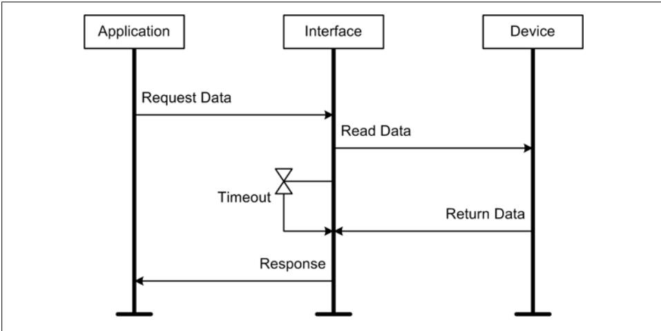
Figure 11-10. I/O transaction
