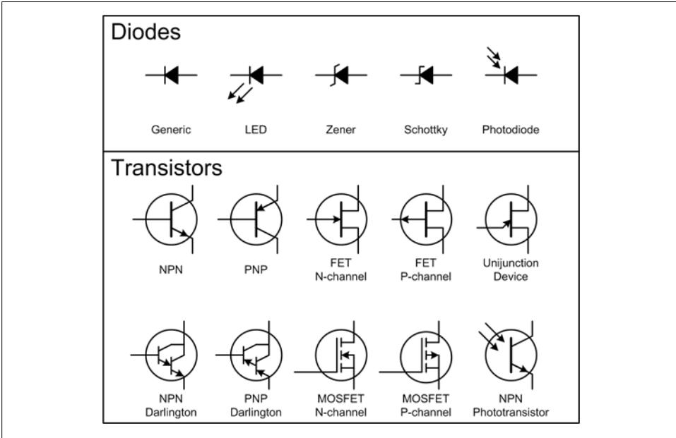
Figure 2-6. Solid-state components
