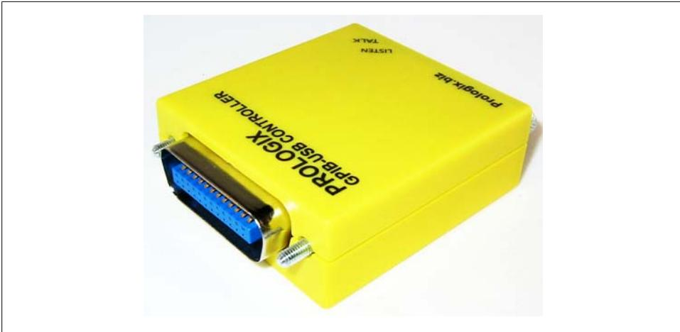
Figure 7-40. USB-to-GPIB interface
