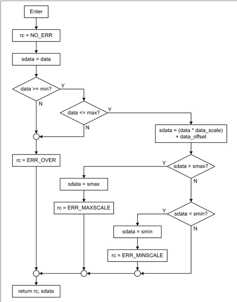
Figure 8-18. `ScaledInput()` flowchart
