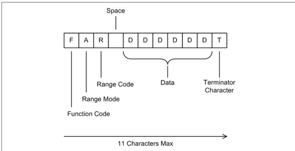
Figure 14-2. tpi model 183 data output format
