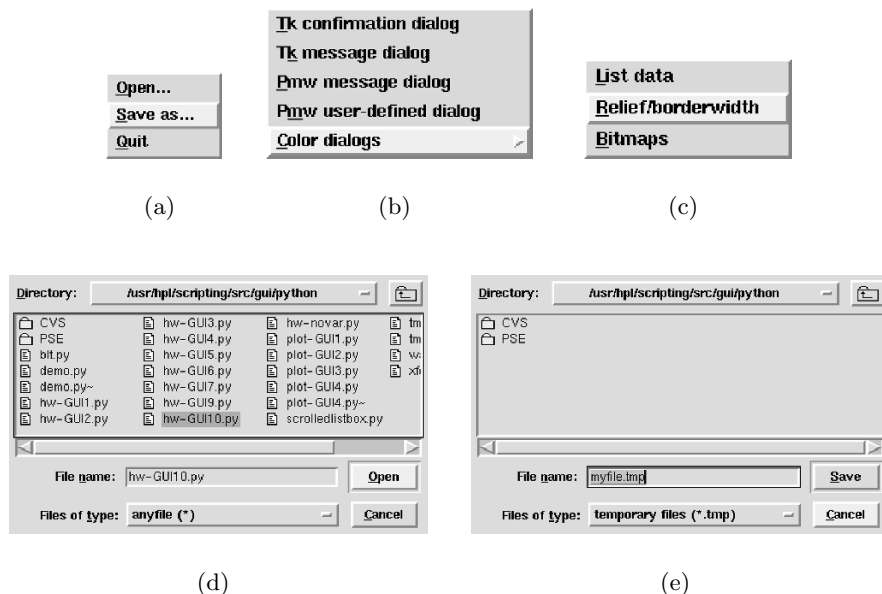
Fig. 6.17. The GUI in Figure 6.15 on page 258 has a menu bar with File, Dialogs, Demo, and Help menu buttons. The former three menus are displayed in (a), (b), and (c). The entries Open... and Save as... in the File menu in (a) pop up the file dialogs in (d) and (e).
