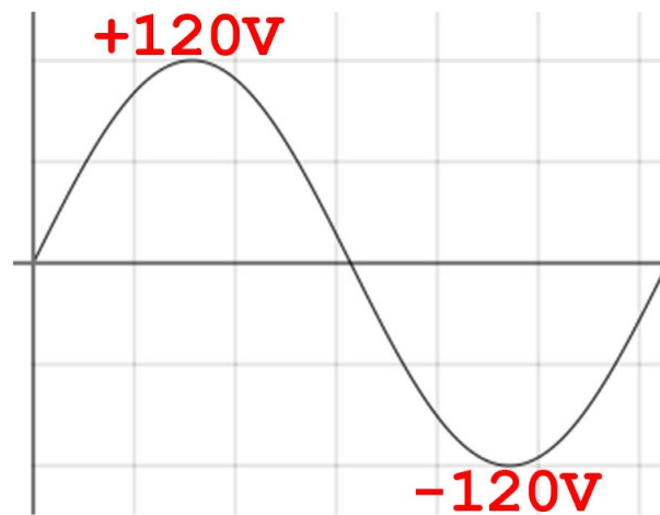
Figure 12.1 Alternating current (AC)
