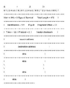
Figure 9-14 Moderate-size IP diagram.
