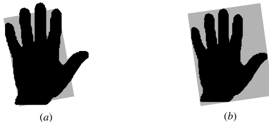
FIGURE 12.6 The rectangle shown in (a) was fitted according to (12.7) as compared to the minimum bounding rectangle shown in (b).
