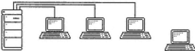
*Multi-user computers* are like personal computers in most ways except that they are shared by more than one user simultaneously. Each user interacts with the multi-user computer using a terminal or application-specific client-server LAN protocol. The icons above represent multi-user computers and their associated terminals.
