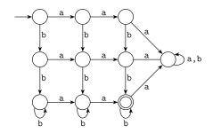
(d) These are DFAs for the two languages  $\{w | w \text{ has an even number of a's} \}$  and  $\{w | \text{ each a in } w \text{ is followed by at least one b} \}$ .
