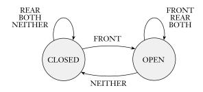
**FIGURE 1.2** State diagram for an automatic door controller
