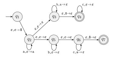
FIGURE **2.17** State diagram for PDA  $M_2$  that recognizes  $\{a^ib^jc^k | i, j, k \ge 0 \text{ and } i = j \text{ or } i = k\}$
