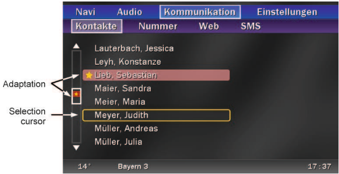
Fig. 6.16. A list of names used in the test system for the “Component Emphasis” adaptation. The system recommends an entry (“Lieb, Sebastian”) by highlighting the respective line.
