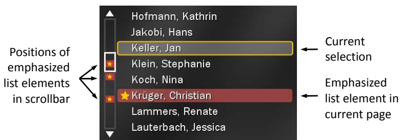
Fig. A.2. Three elements are emphasized in a selection list by the List Element Selection pattern to support the selection of frequently elements. Only one item is visible in the current screen and the positions of the other elements are shown in the scrollbar.
