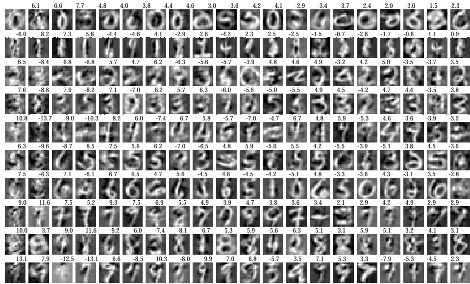
Figure 18.10 Illustration of all the reduced set vectors constructed by the iterative approach of Section 18.5.1 for n = 20 . The associated coefficients are listed above the images. Top: recognizer of digit 0, ..., bottom: recognizer of digit 9. Note that positive coefficients (roughly) correspond to positive examples in the classification problem.
