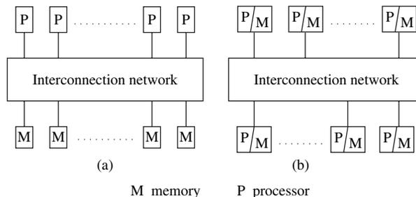
**Figure 1.4** Interconnection networks for shared memory multiprocessor systems. (a) Omega network [4] for  $n = 8$  processors  $P_0$ – $P_7$  and memory banks  $M_0$ – $M_7$ . (b) Butterfly network [10] for  $n = 8$  processors  $P_0$ – $P_7$  and memory banks  $M_0$ – $M_7$ .
