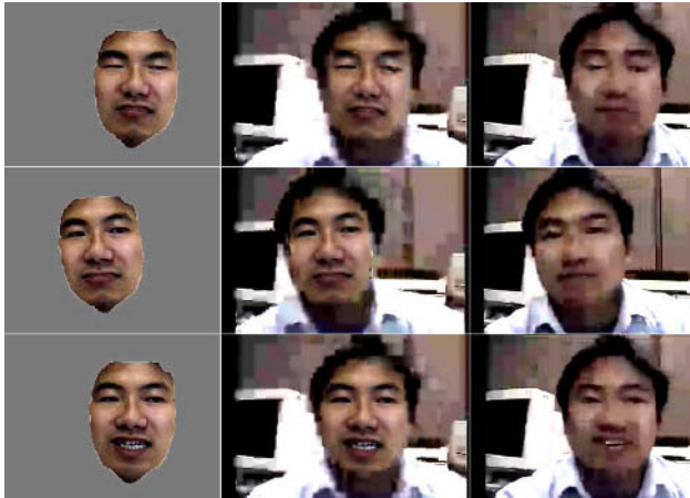
Figure 8. (a) The synthesized face motion; (b) the reconstructed video frame with synthesized face motion; (c) the reconstructed video frame using H.26L codec.
