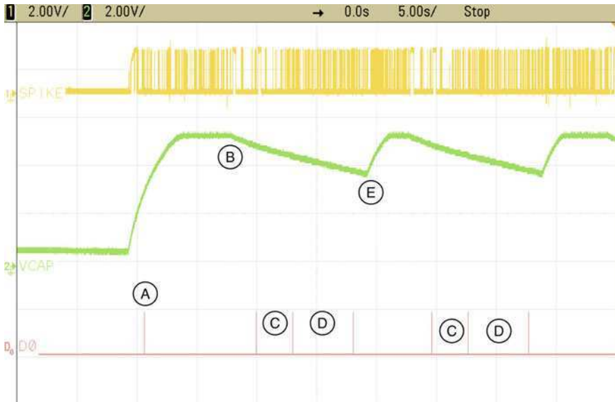
Fig. 10.12 Two read cycles of wireless operation, showing the spike detector output (top), the unregulated stored voltage (middle), and a microcontroller output (bottom) pulsed to show operation. The data was taken at a distance of approximately 1 m from the reader
