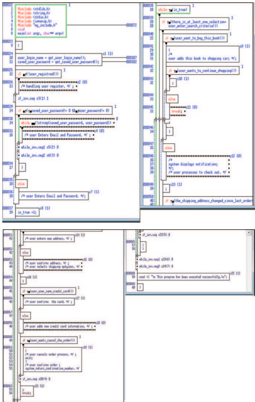
Fig. 12.10 The generated J-Dialog from the listed dummy source code, shown with the test coverage measurement result after dynamic testing
