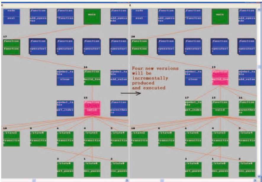
Fig. 7.36 Assigning bottom-up order for incremental software development, including incremental unit coding and unit testing
