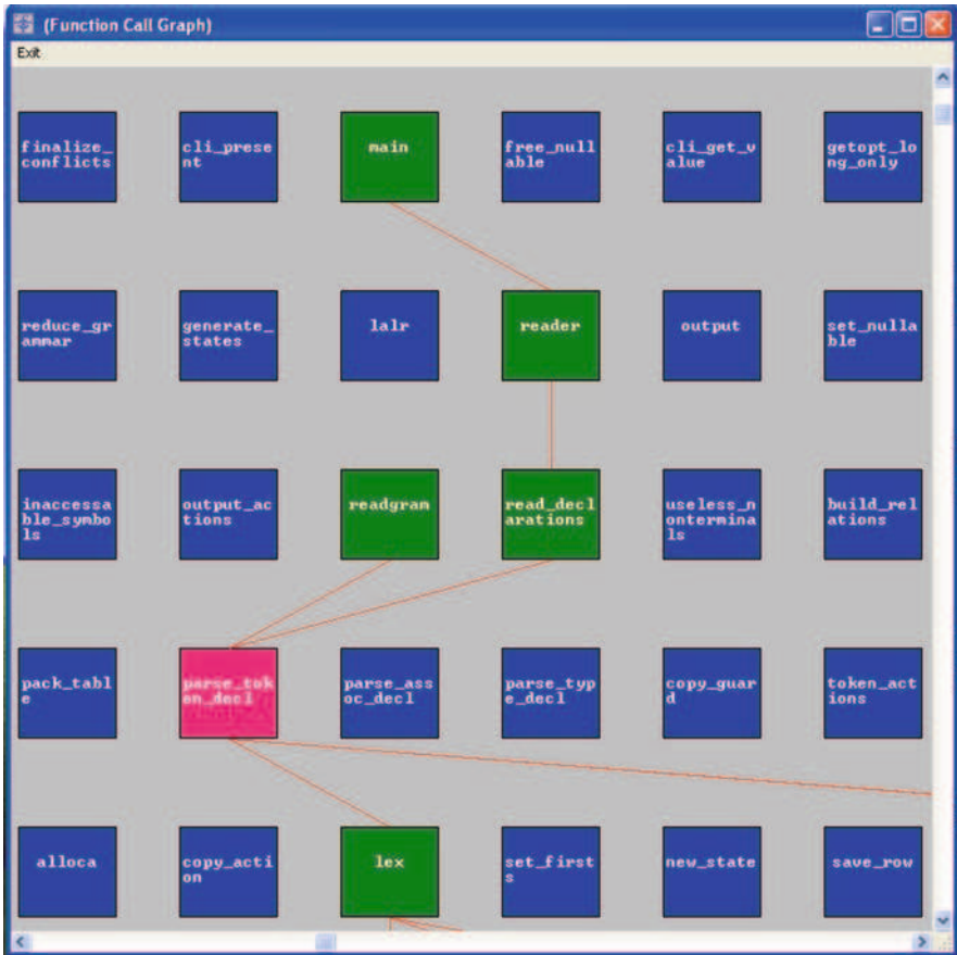
Fig. 6.4 A module and the related modules (calling and called by it) traced and highlighted
