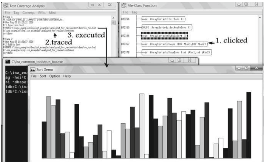
Fig. 13.26 An example of external traceability and dynamic traceability among source code and test cases and the related document or program execution
