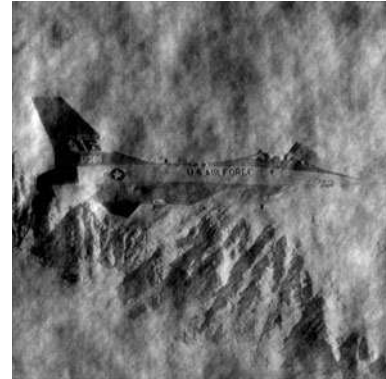
(d) Image obtained by taking the inverse Fourier transform from the synthesized spectrum (magnitude of the “Lena” original spectrum and phase of the “Airplane” original spectrum)
