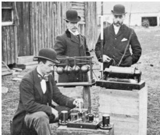
Figure 12.4 Marconi's transmitter, 1897. (Scanned with permission of the ITU from Anthony R. Michaelis, From Semaphore to Satellite , International Telecommunication Union, Geneva, 1965, p. 122.)
