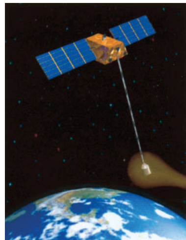
Figure 27.16 Satellite de-orbiting with a Terminator Tether. (Courtesy of Tethers Unlimited.)
