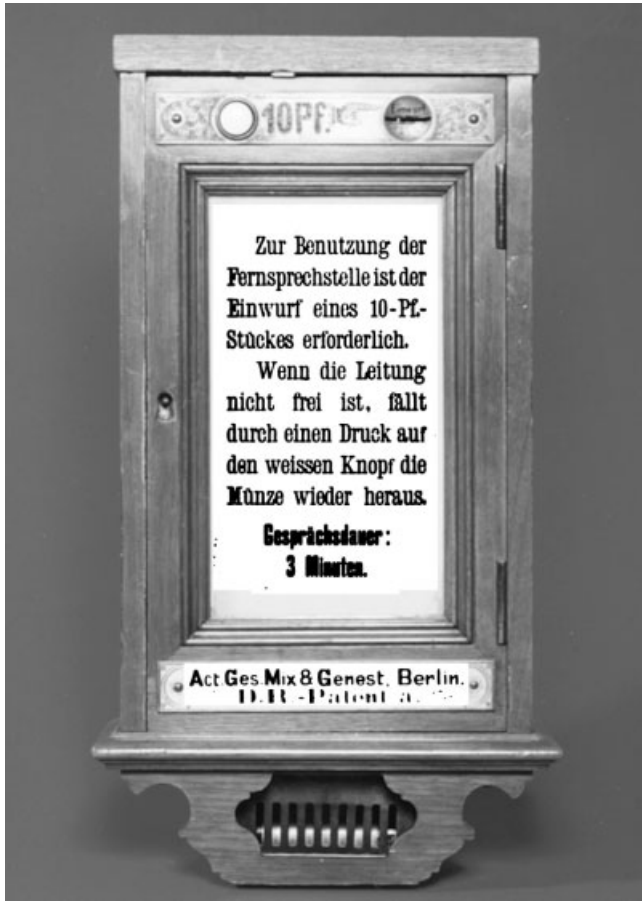
Figure 10.12 First coin-box telephone in Germany, 1891. (Courtesy of Alcatel SEL.)
