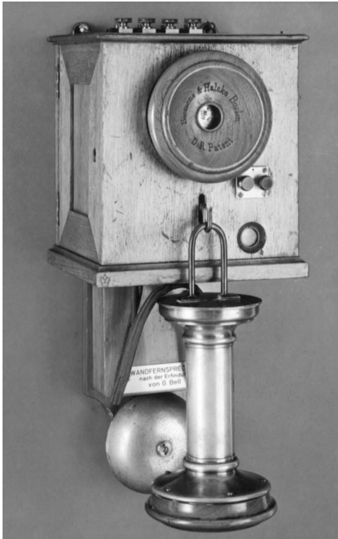
Figure 10.11 Wall-mounted telephone, as used around 1885. (Courtesy of Museum für Kommunikation, Frankfurt, Germany.)
