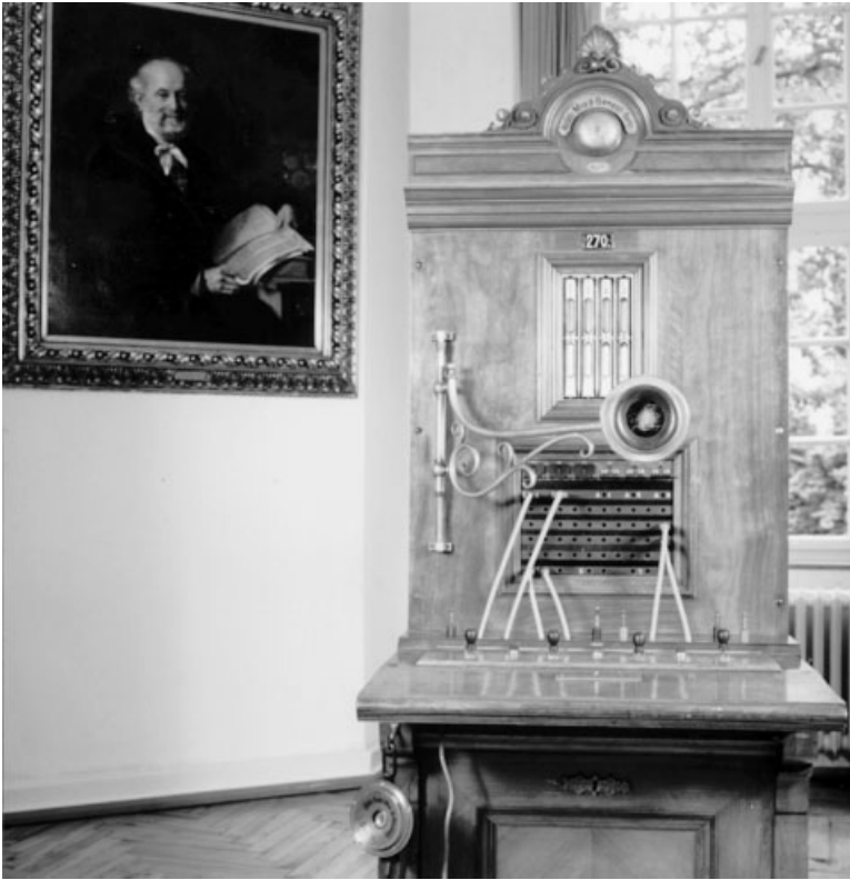
Figure 11.3 Manual exchange used in Germany around 1900. (Courtesy of Alcatel SEL.) See insert for a color representation of this figure.
