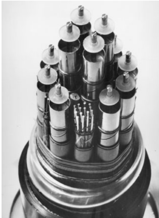
Figure 26.1 Coaxial cable with 12 standard CCI tubes, 1970. (Courtesy of Museum für Kommunikation, Frankfurt, Germany.)
