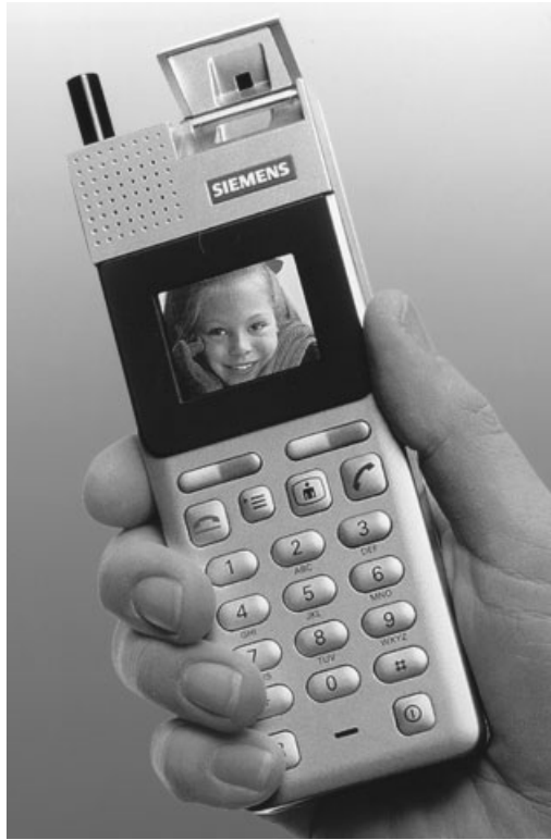
Figure 32.5 DECT prototype handset for videophone transmission, 1998. (Courtesy of Siemens Press Photo.)
