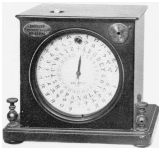
Figure 8.14 Breguet telegraph as used initially in Japan. (Scanned with permission of the ITU from Anthony R. Michaelis, From Semaphore to Satellite , International Telecommunication Union, Geneva, 1965, p. 64.)
