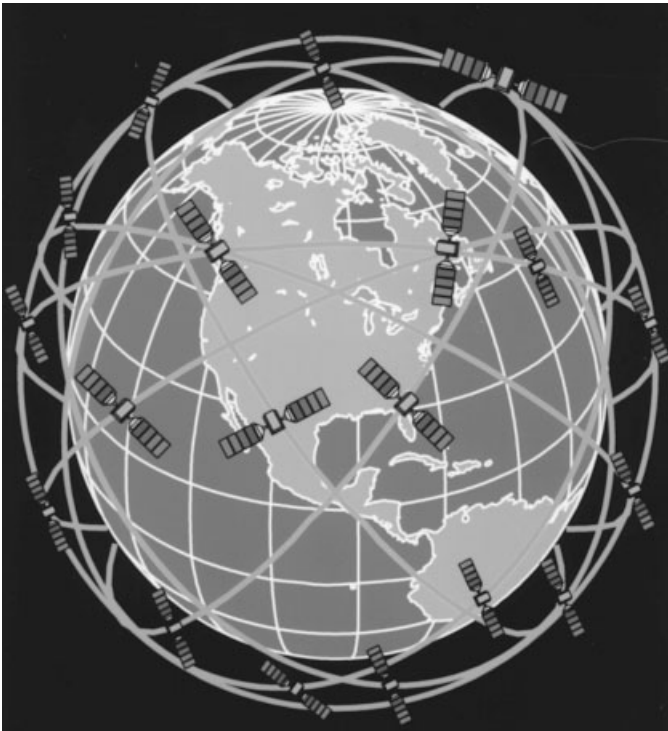
Figure 27.13 Globalstar 48-satellite constellation. (Courtesy of Globalstar.)
