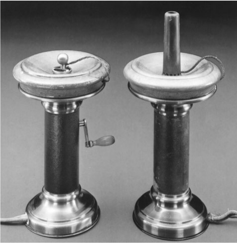
Figure 10.10 Telephone of Siemens with rattle (left) and whistle (right) calling, 1878. (Courtesy of Museum für Kommunikation, Frankfurt, Germany.)
