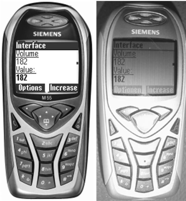
Fig. 7 Simple User Interface for a Siemens M55 mobile phone generated from DISL
