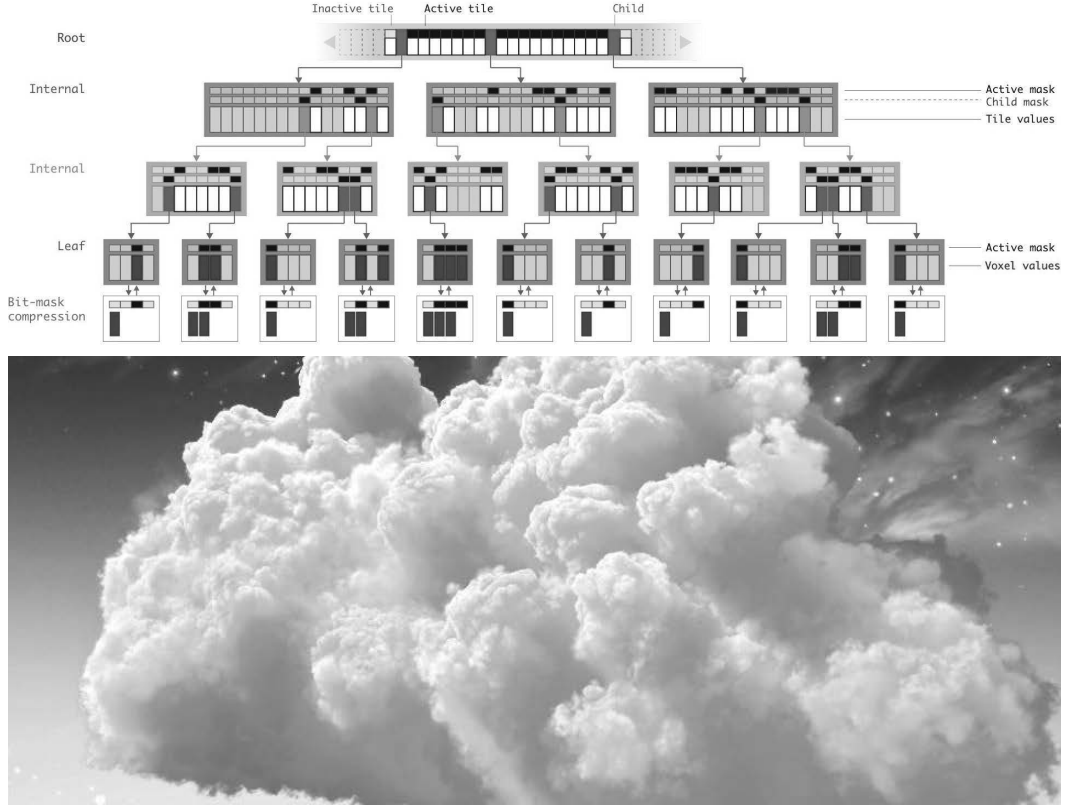
FIGURE 5.1: (Top) Schematic of the OpenVDB data structure for sparse volumes [48] and (bottom) a typical cloud model stored as a sparse volume. The data structure consists of a tree starting with a root node , one or more internal nodes , and finally leaf nodes that store the volume data, for example, density. Existing values can be accessed in parallel, but inserting new values is not threadsafe. However, OpenVDB supports a number of important parallel algorithms. (See Color Insert.)
