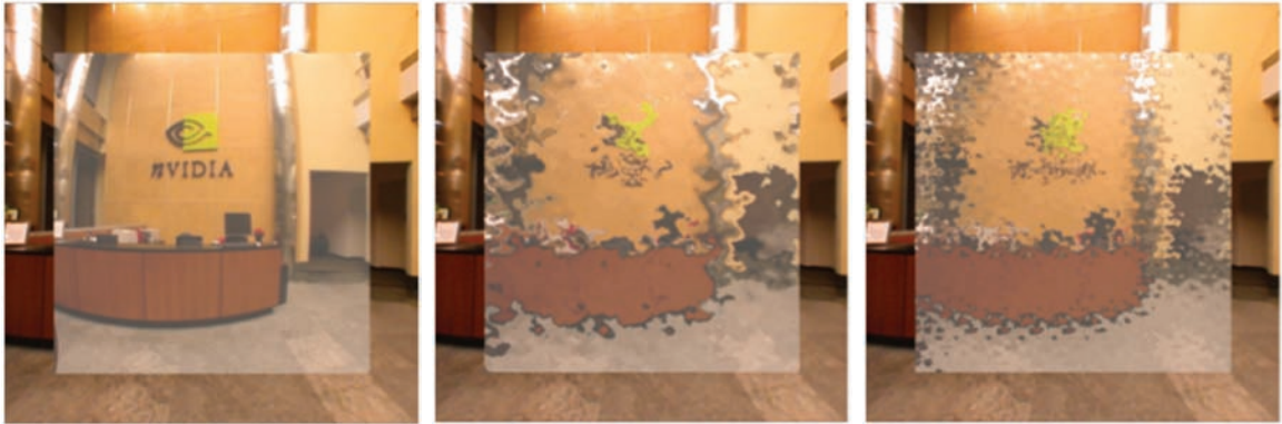
Figure 16.12. The unperturbed normal (left), a small value of uNoiseAmp (middle), and a larger value of uNoiseAmp (right).
