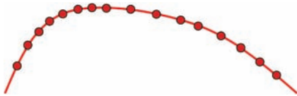
Figure 13.8. The Bézier curve with its positions at uniform values of u .
