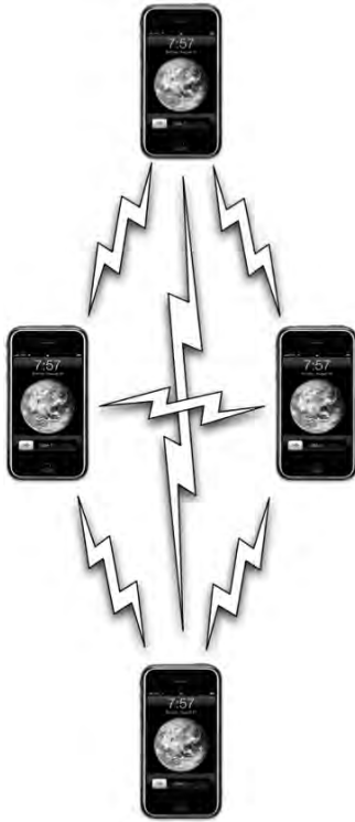
Figure 8–7. In the peer-to-peer model, peers can talk to each other directly, and can continue to do so even in the absence of a server.
