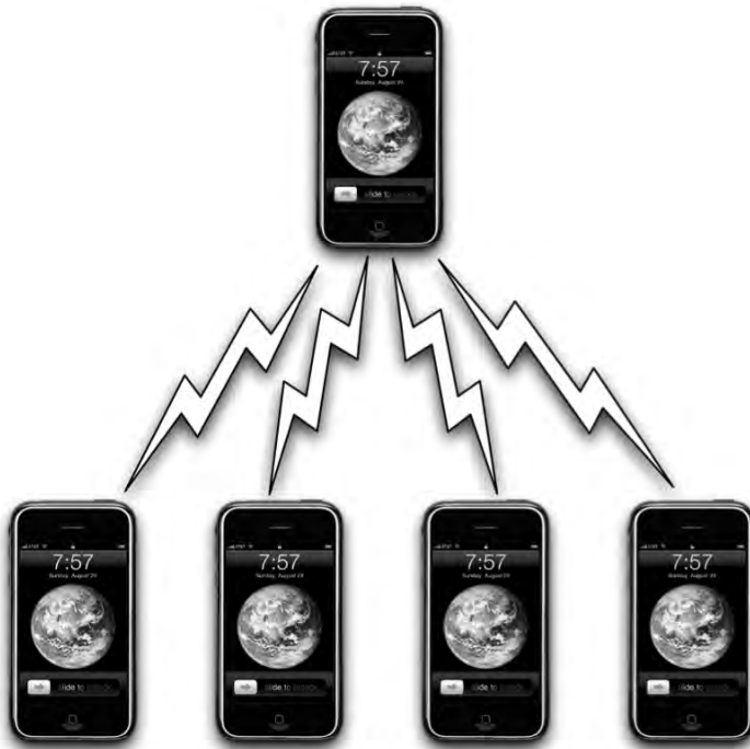
Figure 8–6. The client-server model features one machine acting as a server with all communications—even communications between clients—going through the server.
