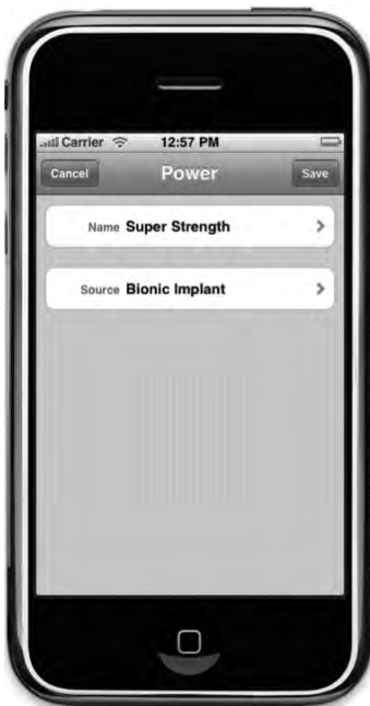
Figure 7-2. The new view for editing powers is actually an instance of the same object used to edit heroes.
