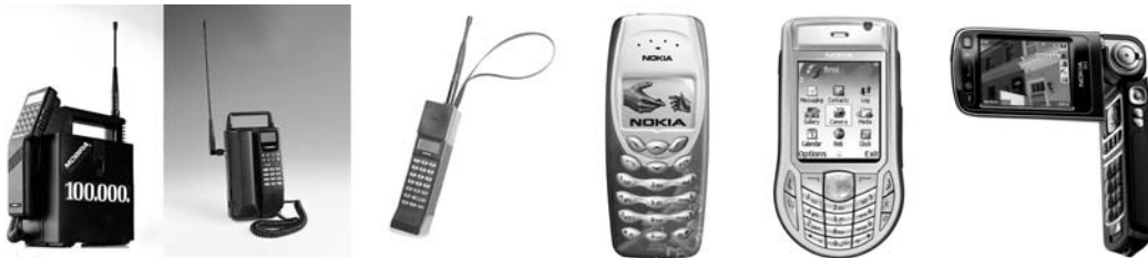
Figure 1.1: The evolution of mobile phones from the early car phones on the left to the multimedia computer on the right spans roughly two decades. From the left: Mobira Talkman, Nokia R72, Mobira Cityman, Nokia 3410 (the first GSM phone with a 3D graphics engine), Nokia 6630 (the first phone to support both OpenGL ES and M3G), and Nokia N93 (the first phone with hardware acceleration for both APIs). Images Copyright © 2007 Nokia Corporation.
