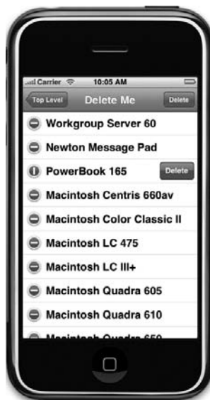
Figure 9-7. The fifth of the Nav application's six subcontrollers implements edit mode to allow the user to delete items from the table.
