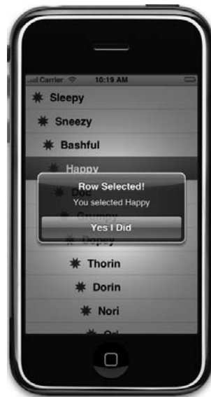
Figure 8-10. In this example, the first row is not selectable, and an alert is displayed when any other row is selected. This was done using the delegate methods.
