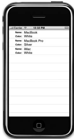
Figure 8-13. Adding subviews to the table view cell can give you multiline rows.
