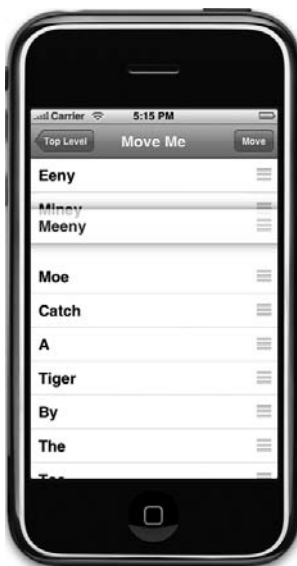
Figure 9-6. The fourth of the Nav application's six subcontrollers lets the user rearrange rows in a list by touching and dragging the move icon.
