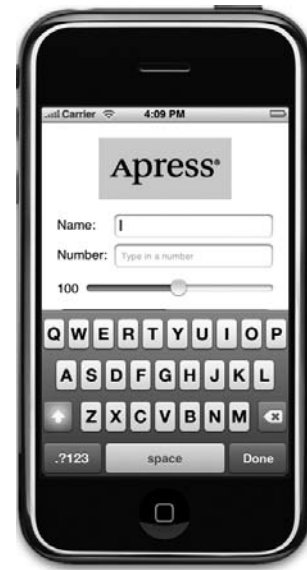
Figure 4-15. The keyboard comes up automatically when you touch the text field.
