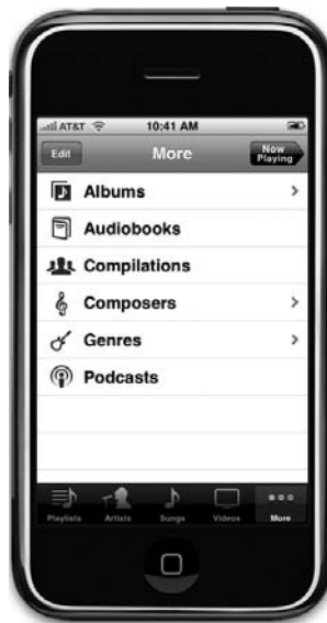
Figure 6-4. The iPod application uses both a navigation bar and a tab bar.
