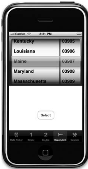
Figure 7-5. In this picker, one component is dependent on the other. As we select a state in the left component, the right component changes to a list of ZIP codes in that state.
