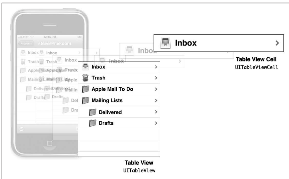
Figure 8-2. Each table view is an instance of UITableView , and each visible row is an instance of UITableViewCell .
