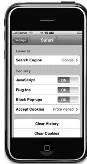
Figure 9-1. The Settings application uses a navigation controller. In the upper left (1) is the navigation button used to pop the current view controller off the stack, returning you to the previous level of the hierarchy. The title (2) of the current content view controller is also displayed.
