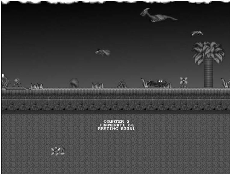
Figure 11.3 The TimedLoop program demonstrates how to slow a program down to a consistent frame rate.
