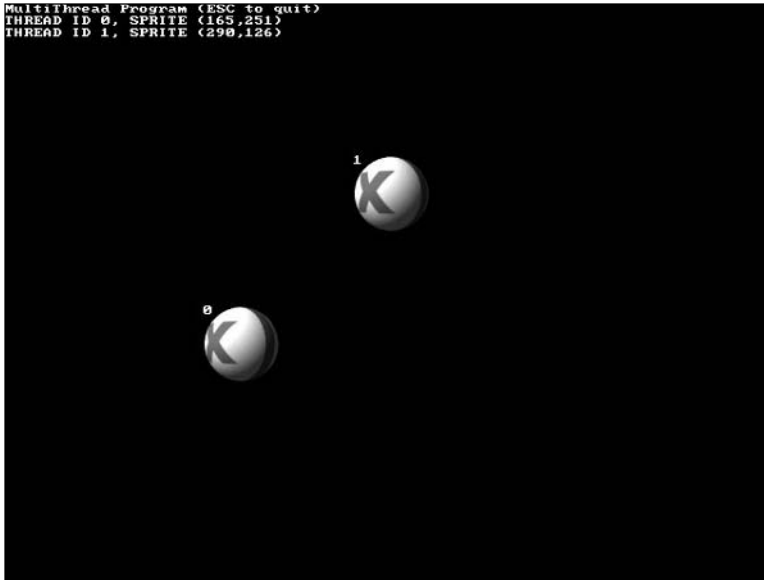
Figure 11.4 The MultiThread program uses threads to control sprite animation on the screen.
