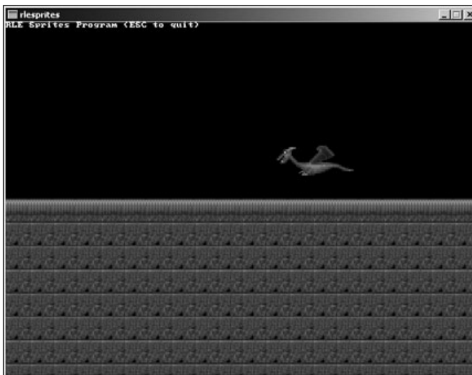
Figure 9.9 The RLESprites program demonstrates how to use run-length encoded sprites to save memory and speed up sprite blitting.
