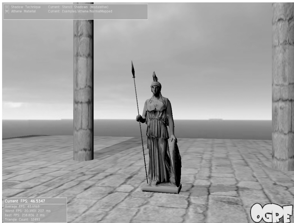
Figure 11-2. Demo_Shadows with modulative stencil shadows enabled
