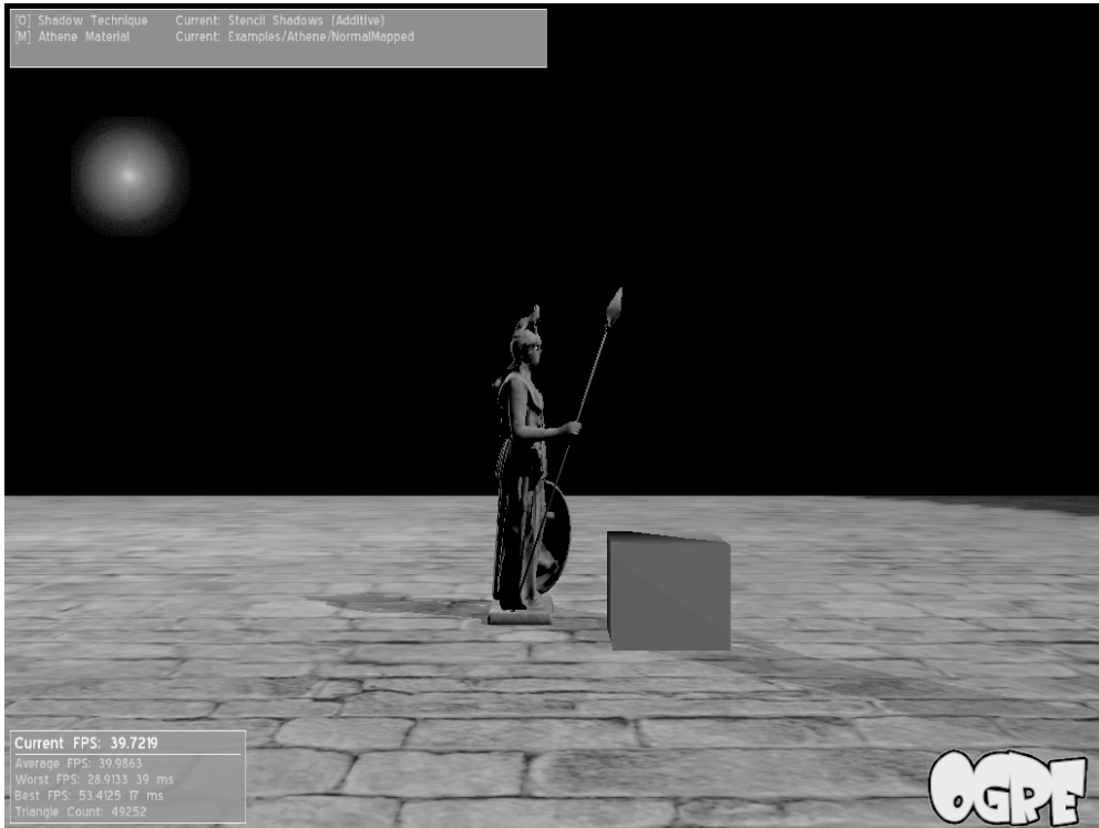
Figure 11-5. Shadow volumes are not occluded by geometry.
