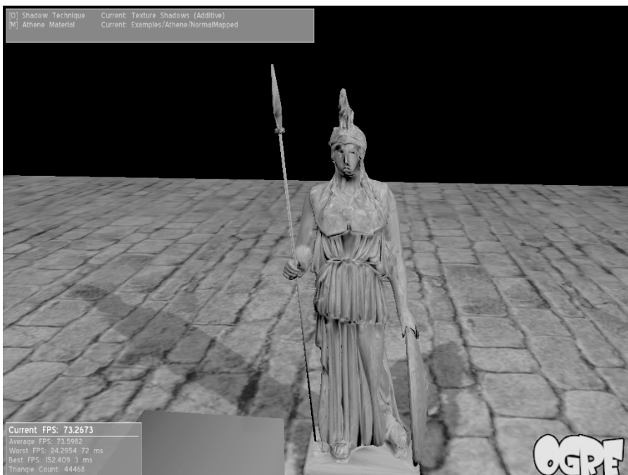
Figure 11-7. Texture shadows. Note the lack of self-shadowing on the Athene's right arm and left leg with the texture technique.
