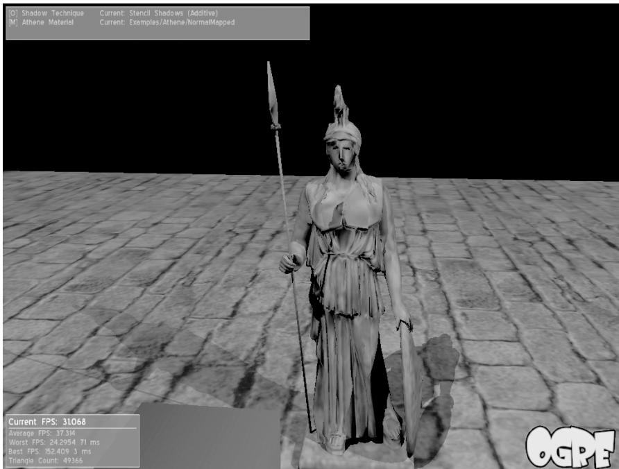
Figure 11-6. Stencil shadows. Note the self-shadowing on the Athene's right arm and left leg.
