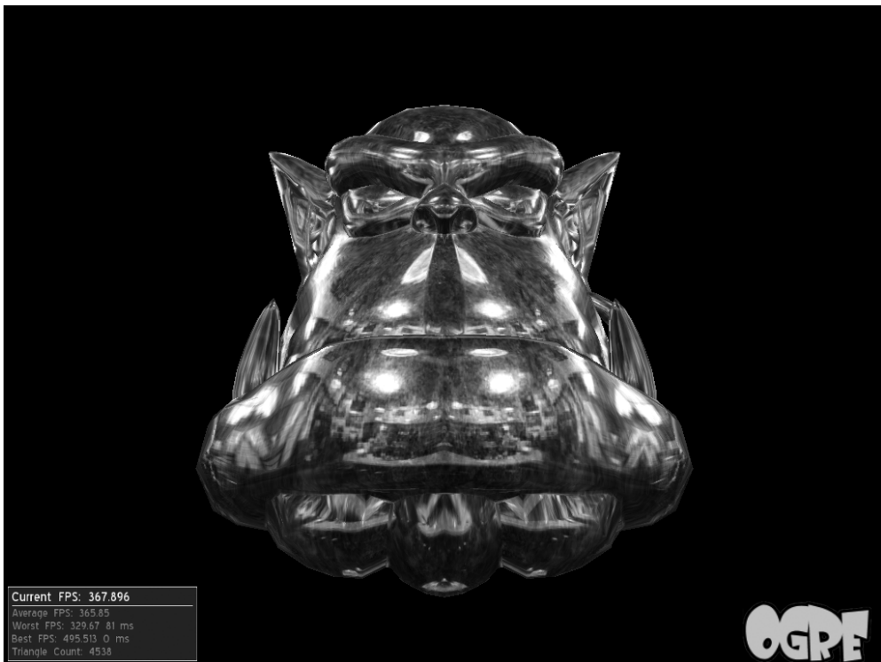
Figure 6-5. The Ogre Demo_EnvMapping sample application, demonstrating the blending of the environment map with the rusty-steel texture
