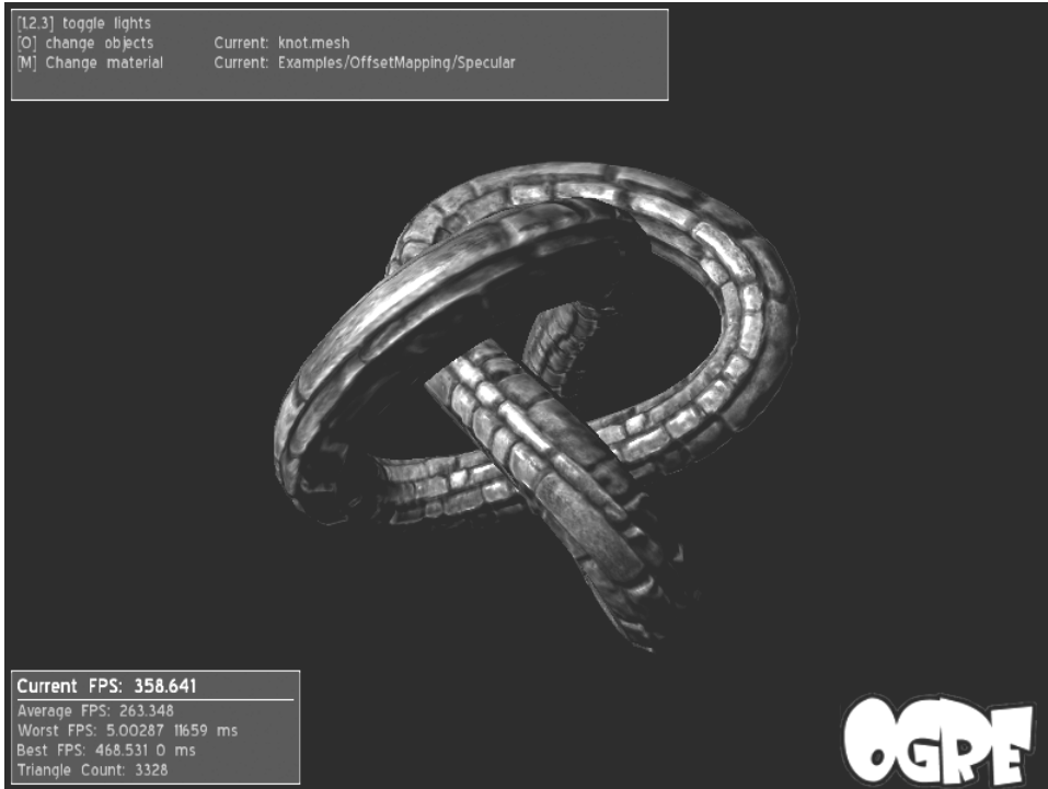
Figure 6-8. Parallax (offset) mapping in the Demo_Dot3Bump sample
