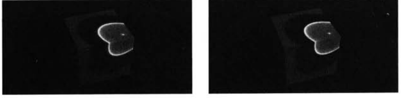
Figure 7.5. The caustic from a lens on a cube using 10,000 photons. The left image is the unfiltered radiance estimate and has some blur at the edges. The right image shows the result of using the cone filter with k = 1.1 —note how the edges are much sharper and more well-defined.
