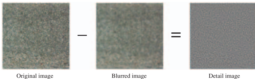
Figure 14.27 Subtracting out low frequencies.
